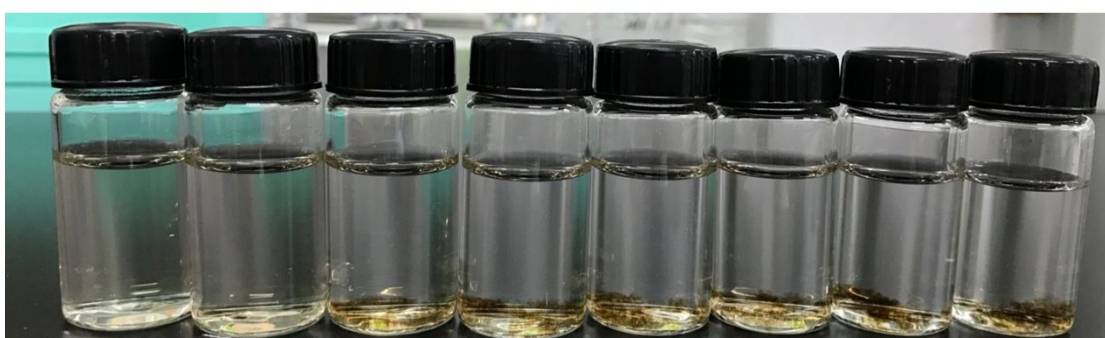
Figure S7. The long-term sedimentation images of 1000 nm (GO-1) (A) and 200 nm (GO-4) (B) GO nanoparticles in the presence of 0, 60, 80, 120, 150, 200, 300 and 600 mM NaCl after 24 h at pH 6.0 and 25 °C.
