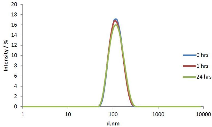
Figure S7. Average DLS result for FITC RB nanosensors in HH Combo medium over 24 hrs.
