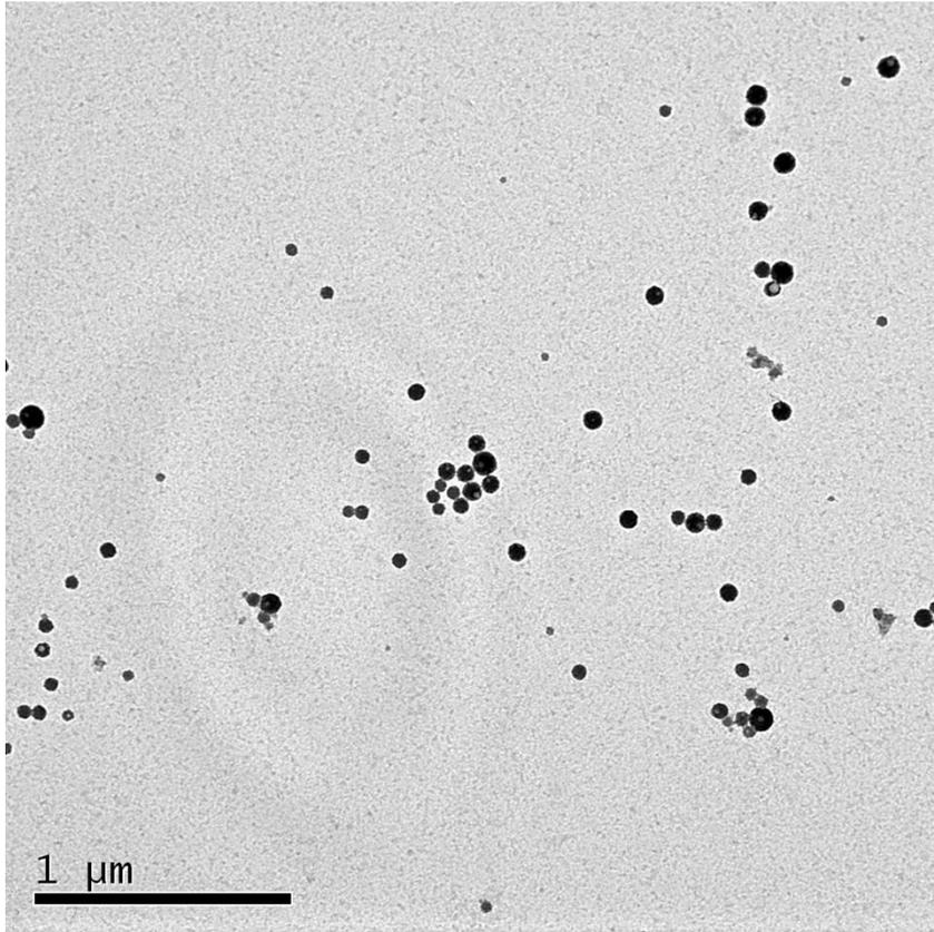
Figure S5. Typical TEM images (A and B) of FITC RB-doped silica nanoparticles
