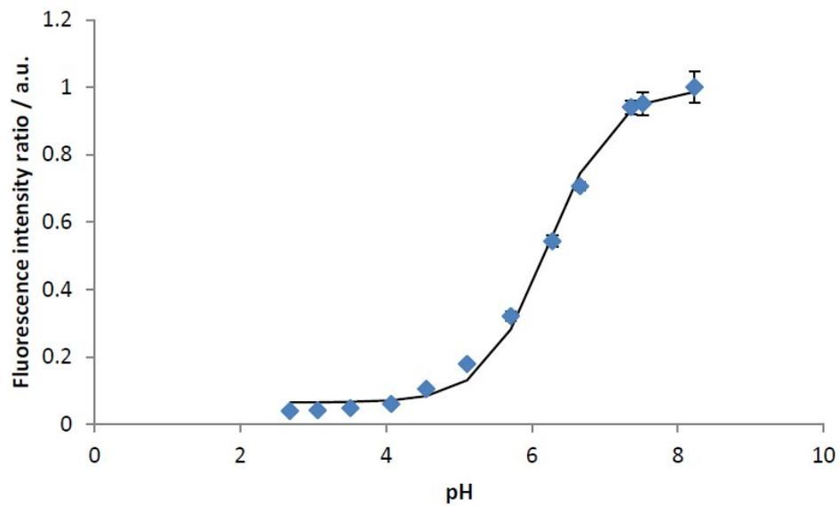
Figure S9. FITC RB nanosensors, bulk calibration in buffer, normalised fluorescence intensity ratio of  $I_{\text{FITC}}/I_{\text{RB}}$  with varying pH. Error bars represent one standard deviation.
