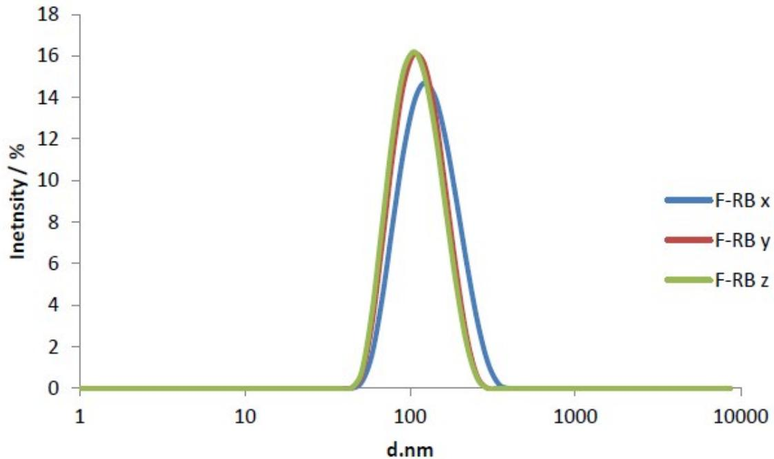
Figure S2. DLS of FITC RB nanosensors prepared from FITC RB sol after 24 hrs
