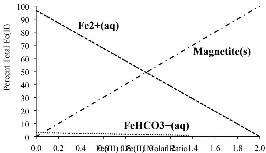
**Figure ESI.6:** Theoretical ferrous iron speciation as a function of ferric iron concentration. As ferric iron concentration approached the stoichiometric ratio for magnetite ( $\text{Fe}^{2+}\text{Fe}^{3+}_2\text{O}_4$ ), magnetite replaced ferrous ions as the dominant species.
