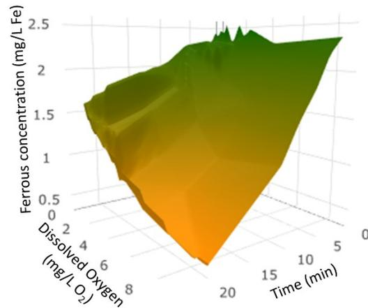
**Figure ESI.2:** The impact of (A) pH and (B) dissolved oxygen on ferrous oxidation rates. Surfaces were interpolated from time series of decreasing ferrous concentrations under conditions of varying pH or dissolved oxygen.
