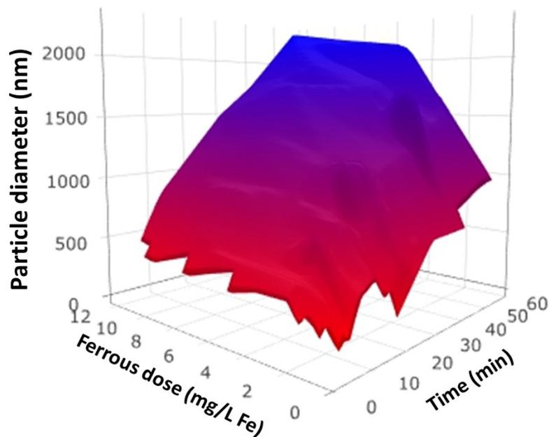
**Figure ESI.4:** Floc formation over time for varying ferrous doses. The surface shown was interpolated from dynamic light scattering measurements for 84 independent particle diameter measurements.
