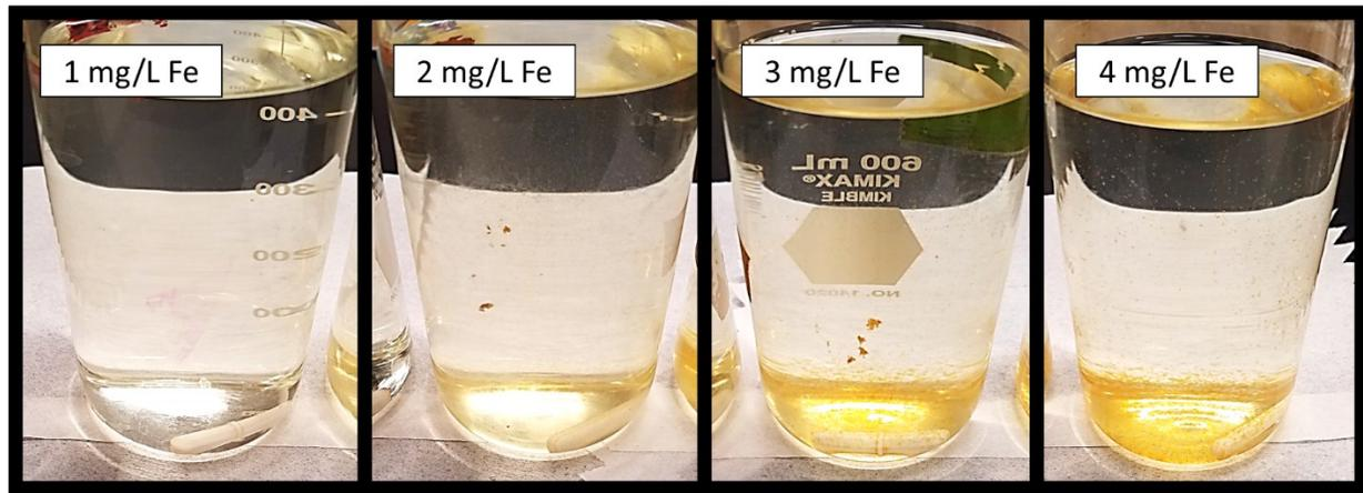
**Figure ESI.3:** Floc formation at varying ferrous iron doses. Iron was spiked as  $\text{FeCl}_2 \cdot 4\text{H}_2\text{O}$  and allowed to form at slow mixing (60 rpm) for 90 minutes. By visual evaluation, abundant, large flocs formed at 3 mg/L Fe and above, while few settleable flocs formed at lower concentrations. These results support the floc formation trends observed via dynamic light scattering.
