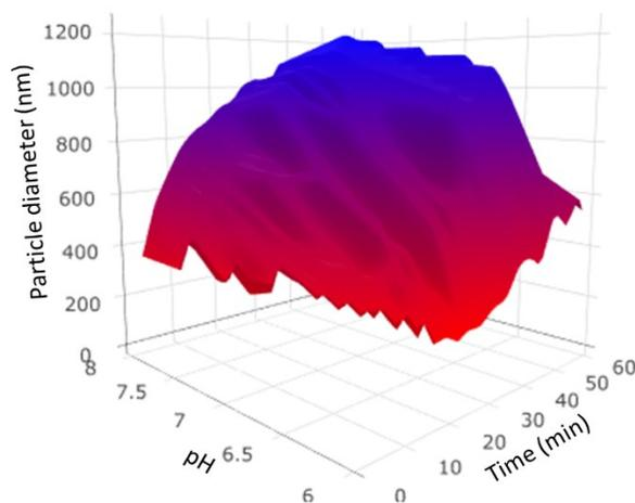
**Figure ESI.5:** Growth of iron flocs over time as a function of pH. Iron was spiked as  $\text{FeCl}_2$  (2.5 mg/L Fe) into 3 mM  $\text{NaHCO}_3$ . Surfaces were interpolated from more than 100 data measurements across the ranges shown.
