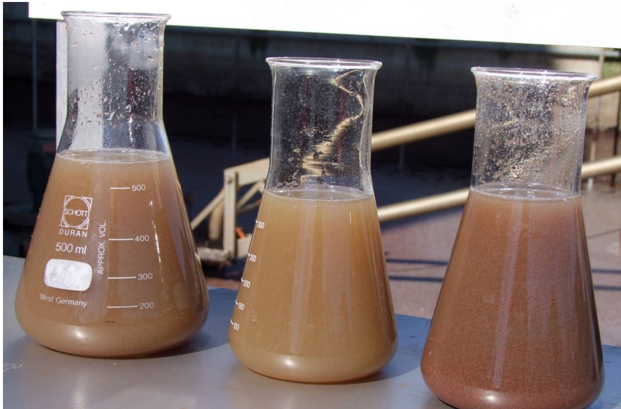
Figure F2. Sidestream deammonification sludge passed through a cyclone. From left to right: Mixed liquor, overflow (reject) and underflow (retained).
