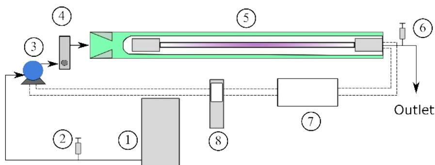
**Figure B (SI).** Flow-through Reactor. (1) water reservoir, (2) inlet sampling point, (3) pump, (4) flow meter, (5) photoreactor, (6) outlet sampling point (dashed lines = electric connections and solid lines = water connections), (7) ballast, (8) power meter (13)
