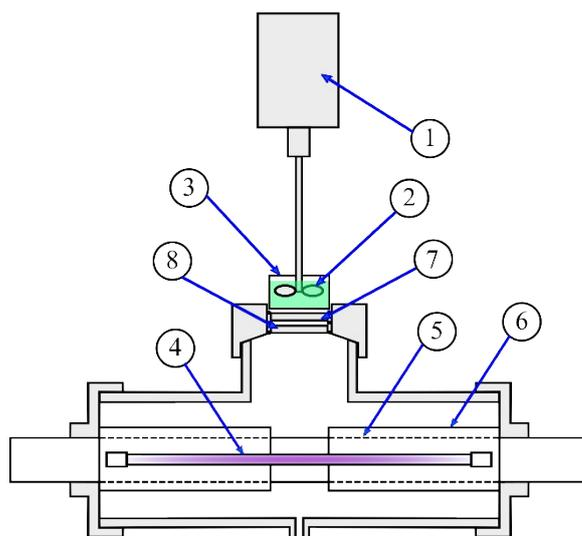
**Figure A (SI).** Collimated Beam Reactor. (1) motor, (2) stirrer, (3) reaction vessel, (4) vacuum UV lamp, (5) quartz sleeve, (6) Teflon cylinder, (7) optical filter, (8) Suprasil® quartz (12)
