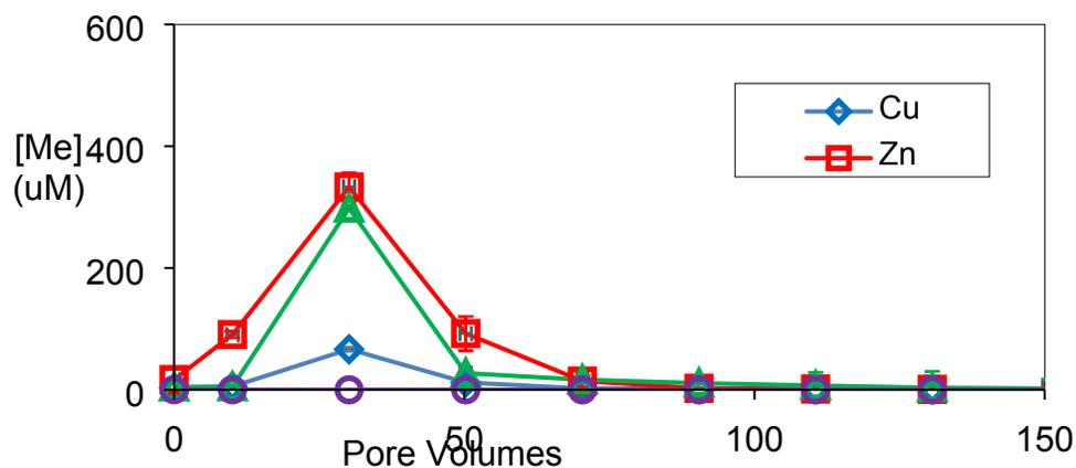
**Figure S8.** Concentrations of effluent Cu, Zn, Cd and Pb during regeneration with pH 3 HCl of columns that treated NOM-containing stormwater. X-axis designates pore volumes of regenerant treatment, immediately following column adsorption tests. Error bars represent standard error of multiple sample tests.
