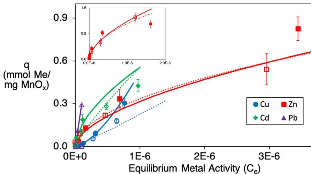
**Figure S3.** Batch adsorption isotherms and Freundlich model fits for Cu, Zn, Cd and Pb with 500 mg manganese oxide-coated sand in simulated stormwater with 8.0 mg-C/L Suwannee River (closed symbols, solid line) NOM and 6.3 mg-C/L Sigma humic acid (open symbols, dotted line). Samples equilibrated for 24 h. Zn data are truncated to illustrate the relative trends of metals; the complete Zn isotherm is inset. Error bars from triplicate experiments smaller than symbols in some cases.
