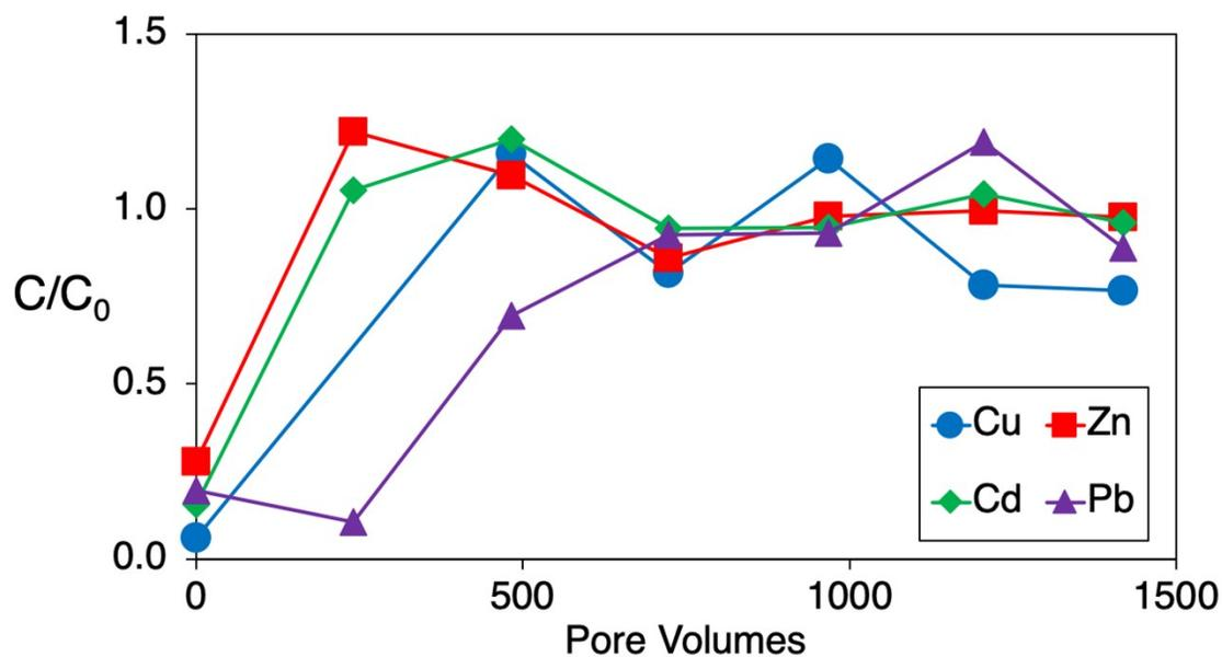
**Figure S4.** Relative concentration of metals in effluent from control columns of acid-washed sand. Experiments conducted in pH 7 NOM-free simulated stormwater.
