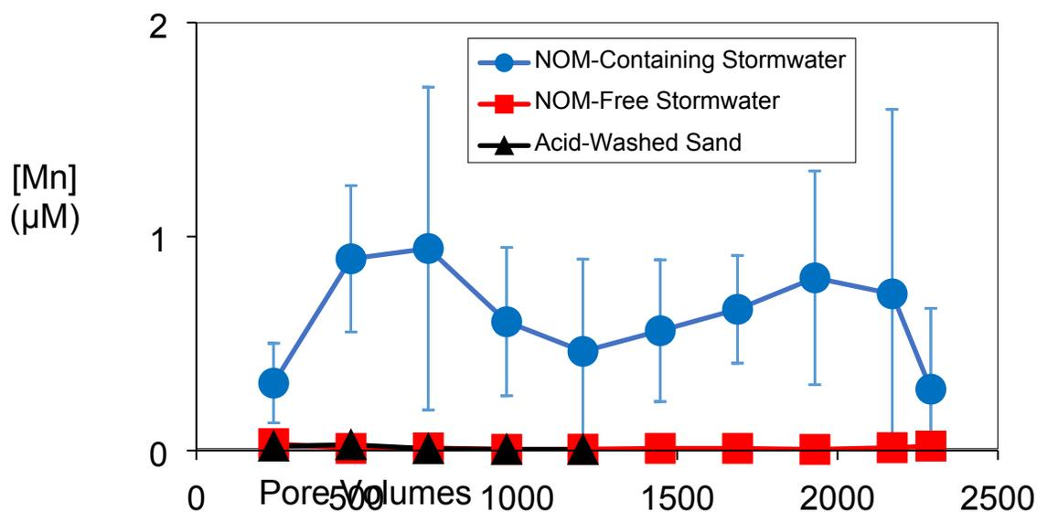
**Figure S6.** Average concentration of Mn in effluent from columns treating metals in NOM-containing (orange circles) and NOM-free (green squares) simulated stormwater. Mn in effluent from acid-washed sand control column was negligible (black triangles). Some error bars are smaller than the data symbols.
