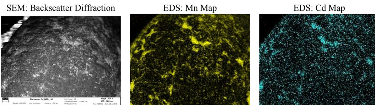
**Figure S5.** Backscatter diffraction scanning electron micrograph (left) and energy dispersive X-ray spectroscopy element maps (center, right) of representative geomedia used to treat of Cd-containing stormwater in columns. All images are magnified by a factor of approximately 530X. In the SEM image, Mn-oxide appears bright. In the element maps, Mn appears yellow and Cd appears cyan.
