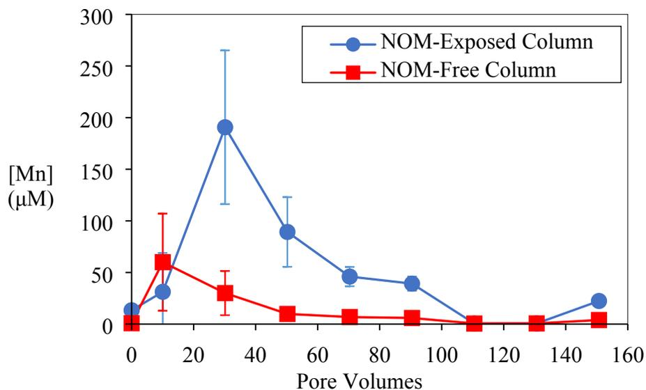
**Figure S9.** Concentrations of Mn in the column effluent during regeneration with pH 3 HCl. Results are shown for columns that treated metals in NOM-containing stormwater (circles) and NOM-free (squares) simulated stormwater. The x-axis designates pore volumes of regenerant treatment, immediately following column adsorption tests. Error bars represent standard error from all regeneration experiments
