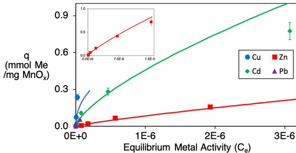
**Figure S2.** Batch adsorption isotherms and Freundlich model fits for Cu, Zn, Cd and Pb with 500 mg manganese oxide-coated sand in NOM-free simulated stormwater at pH 7. Samples equilibrated for 24 h. No isotherm model was developed to fit Pb due to low aqueous equilibrium concentrations. Zn data are truncated to illustrate the relative trends of metals; the complete Zn isotherm is inset. Error bars from triplicate experiments smaller than symbols in some cases.
