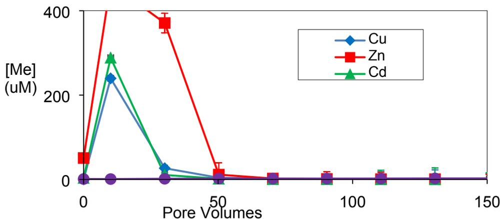
**Figure S7.** Concentrations of effluent Cu, Zn, Cd and Pb during regeneration with pH 3 HCl of columns that treated NOM-free stormwater. X-axis designates pore volumes of regenerant treatment, immediately following column adsorption tests. Error bars represent standard error of multiple sample tests.
