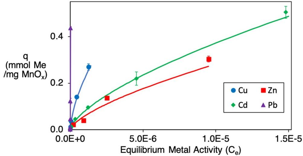
**Figure S1.** Batch adsorption isotherms and Freundlich model fits for Cu, Zn, Cd and Pb with 500 mg manganese oxide-coated sand in NOM-free simulated stormwater at pH 5. Samples equilibrated for 24 h. Error bars from triplicate experiments smaller than symbols in some cases.
