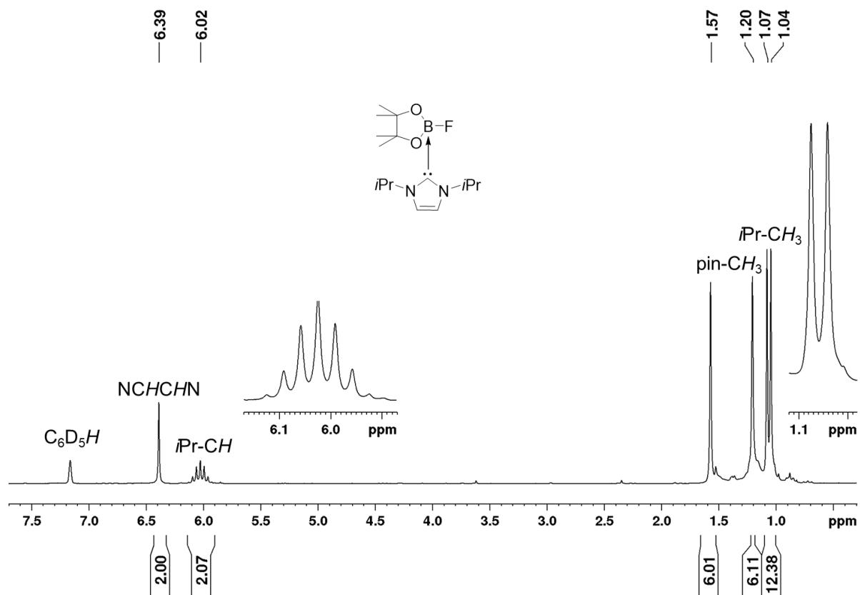
**Figure S3.**  $^1\text{H}$  NMR spectrum of  $\text{FBpin}\cdot\text{iPr}_2\text{Im}$  **1** recorded in  $\text{C}_6\text{D}_6$  (500 MHz).
