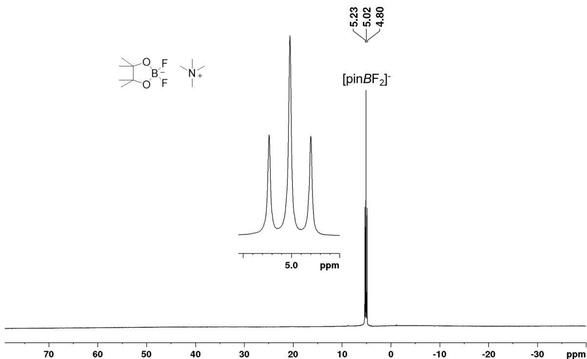
**Figure S23.**  $^{11}\text{B}\{\text{H}\}$  NMR spectrum of  $[\text{pinBF}_2]\text{[NMe}_4\text{]} \mathbf{6}$  recorded in  $\text{CD}_3\text{CN}$  (128 MHz).
