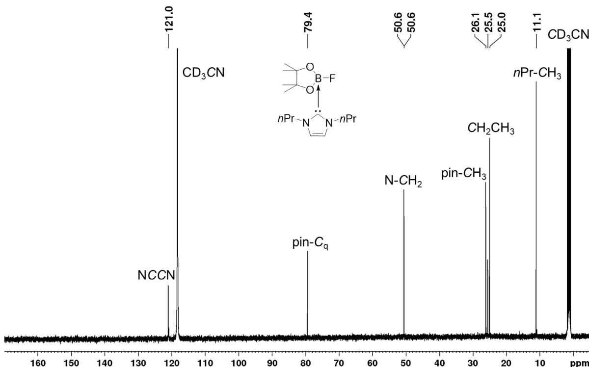
**Figure S14.**  $^{13}\text{C}\{^1\text{H}\}$  NMR spectrum of  $\text{FBpin}\cdot n\text{Pr}_2\text{Im}$  4 recorded in  $\text{CD}_3\text{CN}$  (125 MHz).
