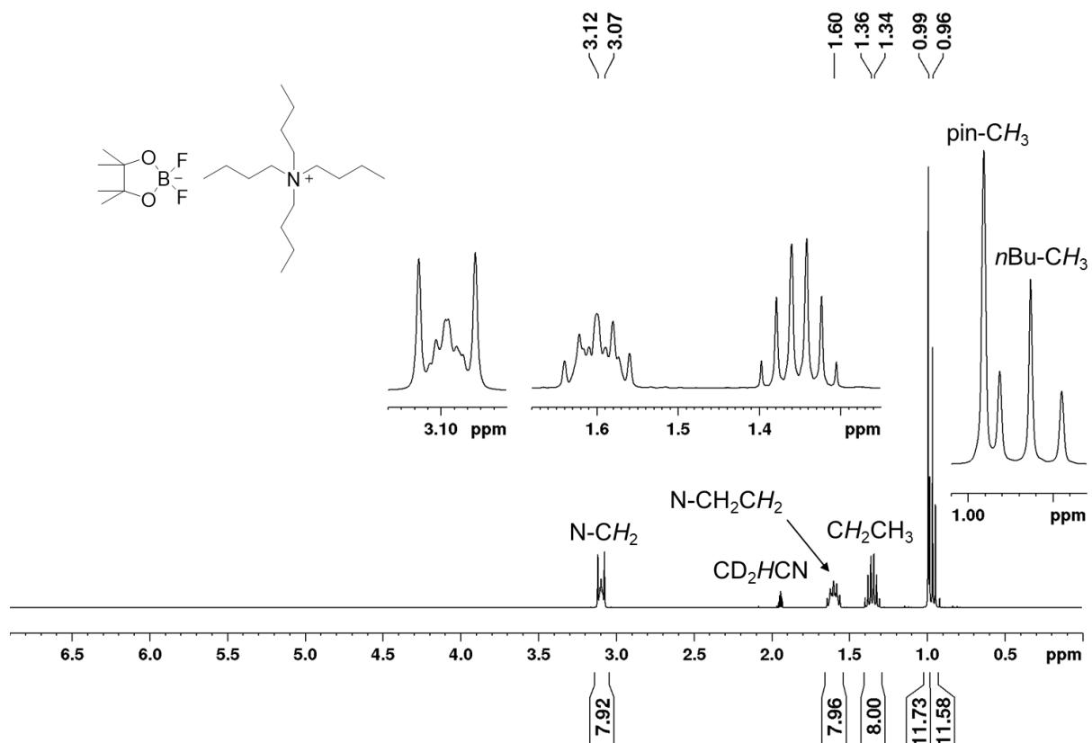
**Figure S25.**  $^1\text{H}$  NMR spectrum of  $[\text{pinBF}_2][\text{NnBu}_4]$  **7** recorded in  $\text{CD}_3\text{CN}$  (400 MHz).
