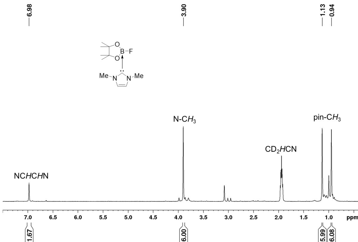
**Figure S7.**  $^1\text{H}$  NMR spectrum of  $\text{FBpin}\cdot\text{Me}_2\text{Im}$  **2** recorded in  $\text{CD}_3\text{CN}$  (200 MHz).
