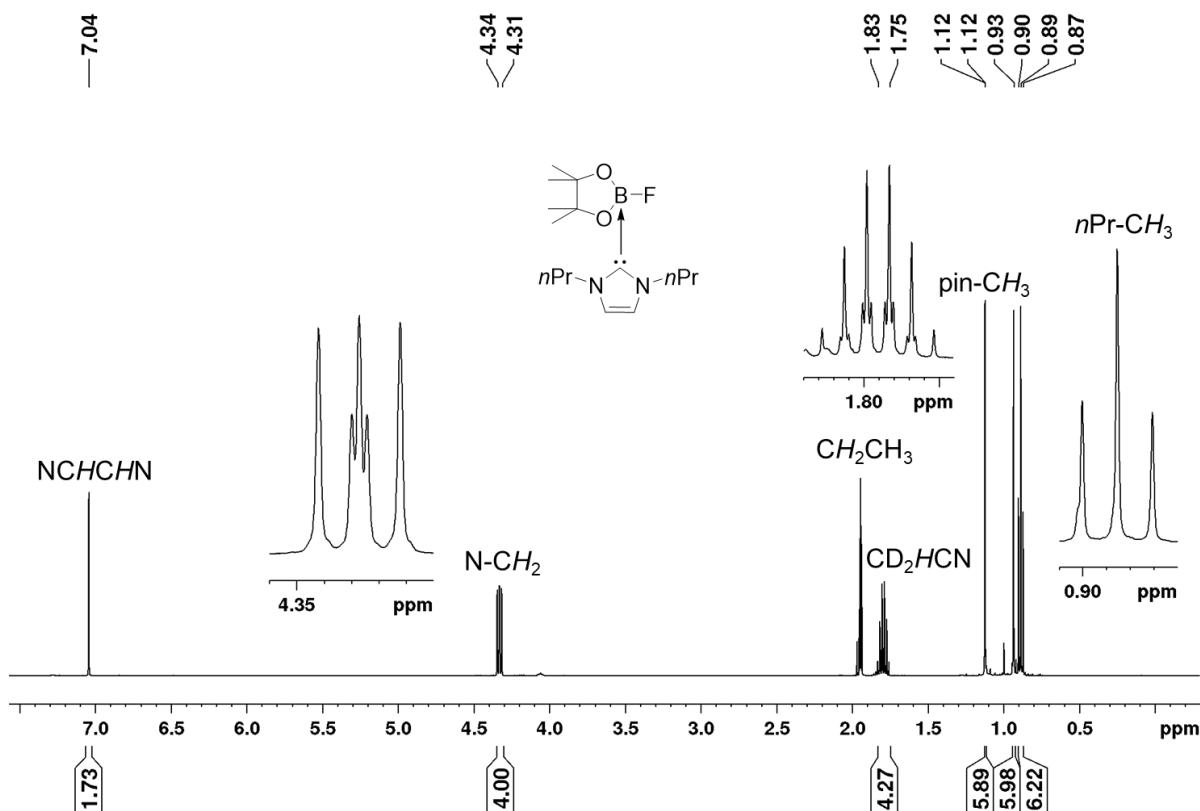
**Figure S13.**  $^1\text{H}$  NMR spectrum of  $\text{FBpin}\cdot n\text{Pr}_2\text{Im}$  4 recorded in  $\text{CD}_3\text{CN}$  (500 MHz).
