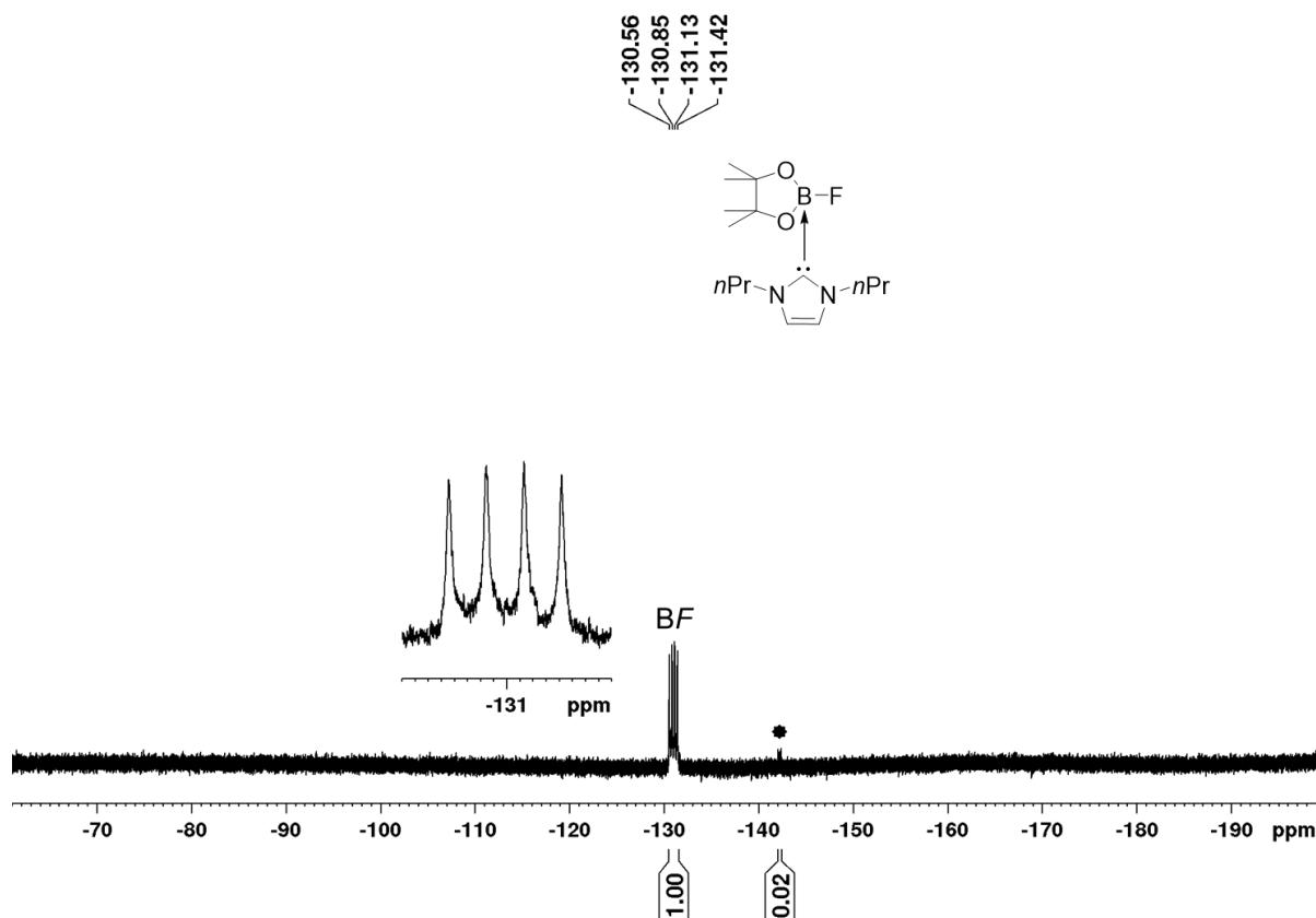
**Figure S16.**  $^{19}\text{F}$  NMR spectrum of  $\text{FBpin}\cdot\text{nPr}_2\text{Im}$  **4** recorded in  $\text{CD}_3\text{CN}$  (471 MHz). (\* =  $[\text{pinBF}_2][\text{NMe}_4]$  **6**)
