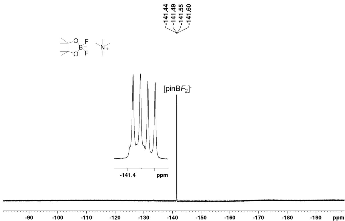
**Figure S24.**  $^{19}\text{F}$  NMR spectrum of  $[\text{pinBF}_2]\text{[NMe}_4\text{]} \mathbf{6}$  recorded in  $\text{CD}_3\text{CN}$  (376 MHz).
