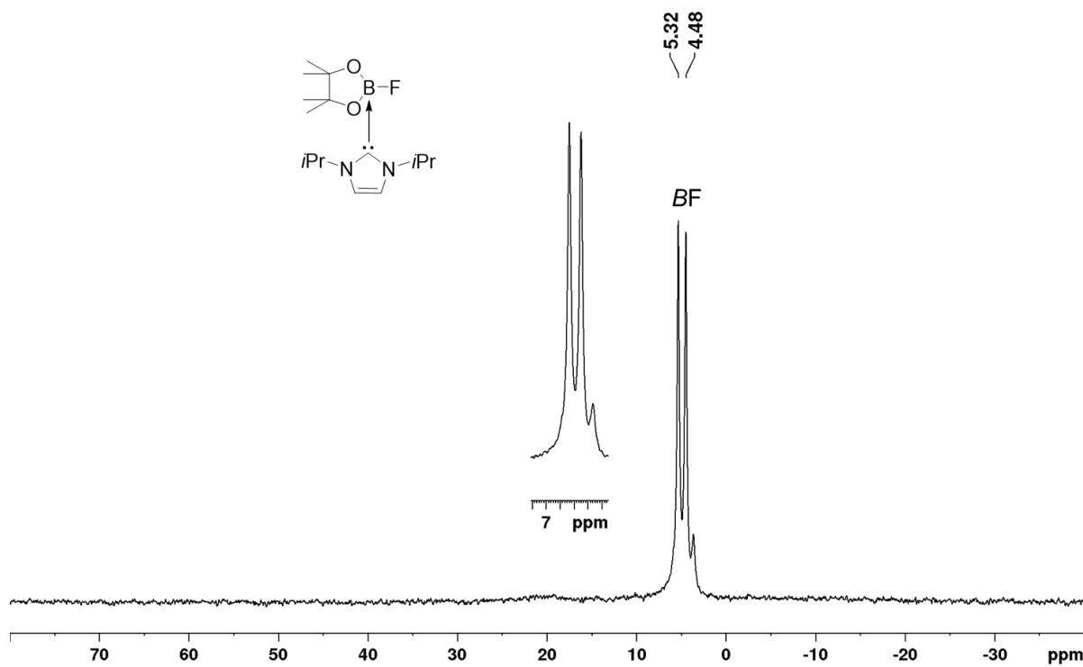
**Figure S5.**  $^{11}\text{B}\{\text{H}\}$  NMR spectrum of  $\text{FBpin}\cdot\text{iPr}_2\text{Im}$  **1** recorded in  $\text{C}_6\text{D}_6$  (160 MHz).
