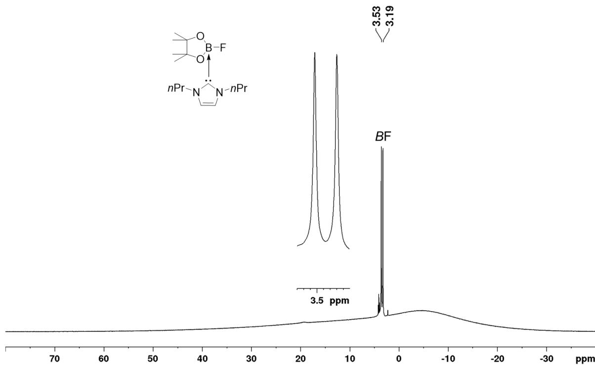
**Figure S15.**  $^{11}\text{B}\{\text{H}\}$  NMR spectrum of  $\text{FBpin}\cdot\text{nPr}_2\text{Im}$  **4** recorded in  $\text{CD}_3\text{CN}$  (160 MHz).
