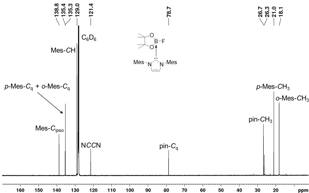
**Figure S18.**  $^{13}\text{C}\{^1\text{H}\}$  NMR spectrum of FBpin·Mes<sub>2</sub>Im **5** recorded in  $\text{C}_6\text{D}_6$  (125 MHz).
