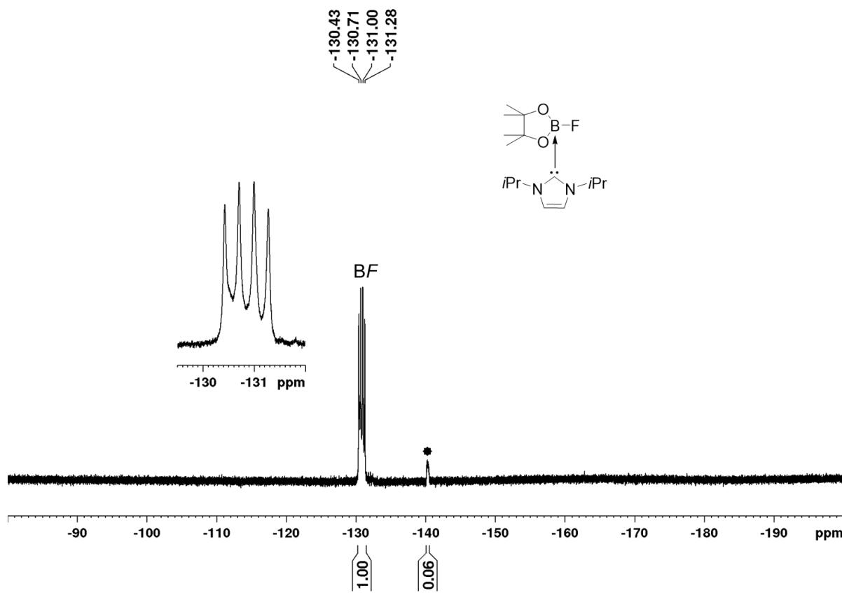
**Figure S6.**  $^{19}\text{F}$  NMR spectrum of  $\text{FBpin}\cdot\text{iPr}_2\text{Im}$  **1** recorded in  $\text{C}_6\text{D}_6$  (471 MHz). (\* =  $[\text{pinBF}_2][\text{NMe}_4]$  **6**)
