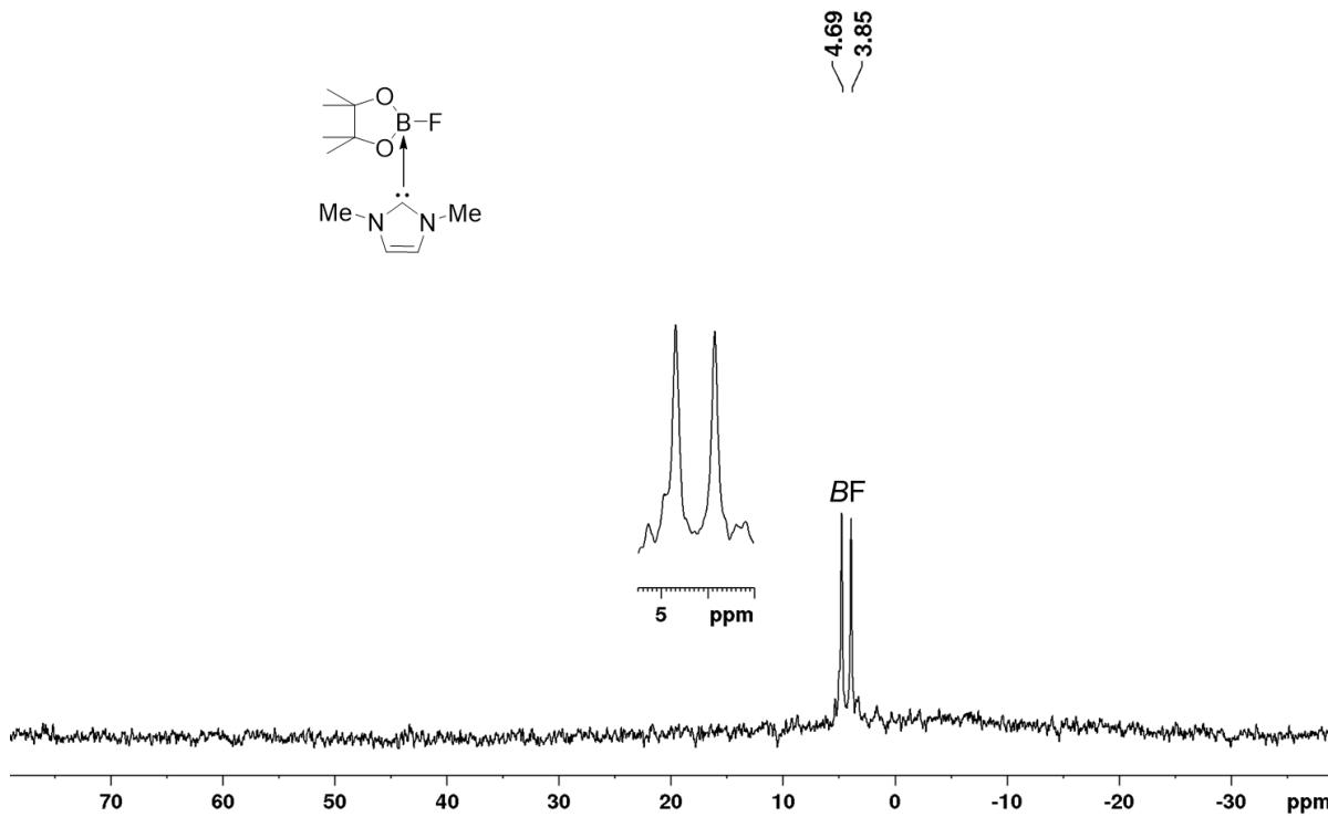
**Figure S8.**  $^{11}\text{B}\{^1\text{H}\}$  NMR spectrum of  $\text{FBpin}\cdot\text{Me}_2\text{Im}$  **2** recorded in  $\text{CD}_3\text{CN}$  (64 MHz).
