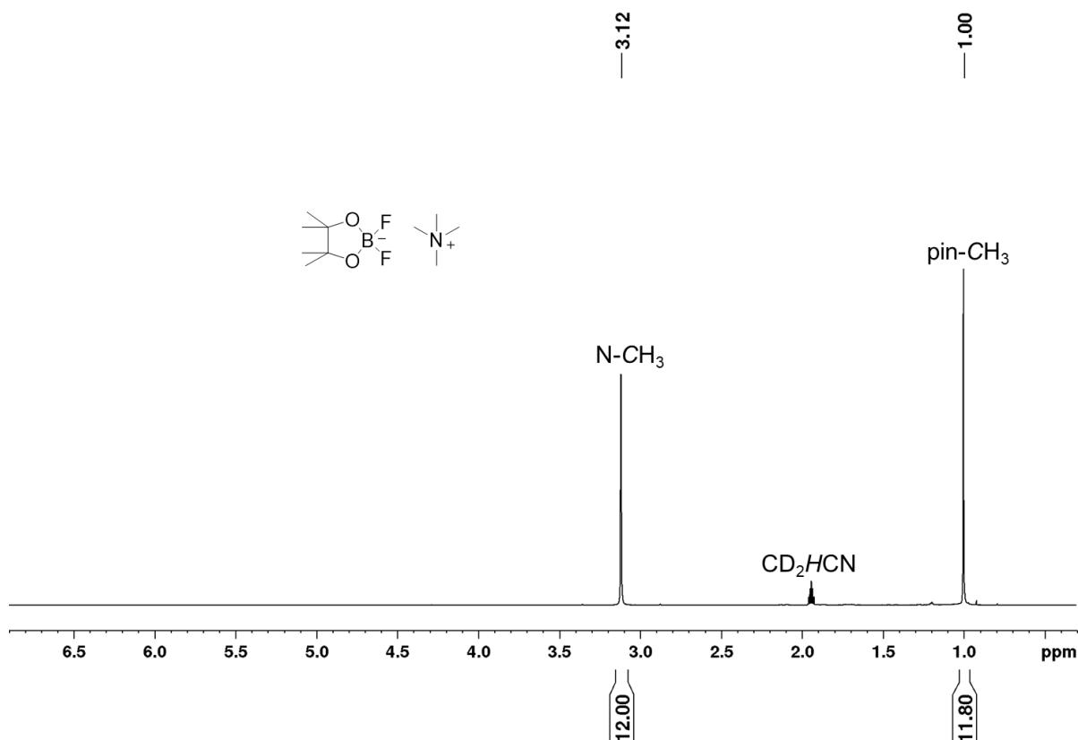
**Figure S21.**  $^1\text{H}$  NMR spectrum of  $[\text{pinBF}_2][\text{NMe}_4]$  **6** recorded in  $\text{CD}_3\text{CN}$  (400 MHz).
