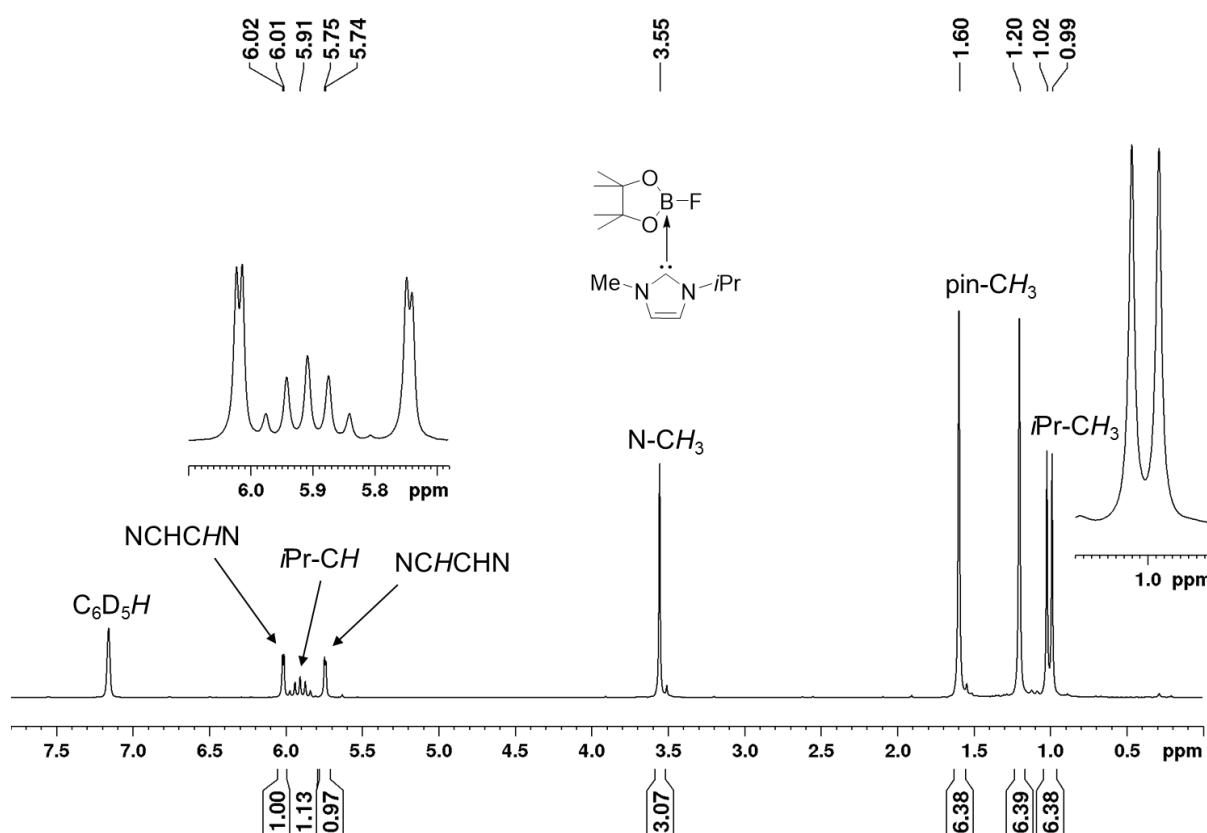
**Figure S10.**  $^1\text{H}$  NMR spectrum of  $\text{FBpin}\cdot\text{Me}_3\text{Im}$  **3** recorded in  $\text{C}_6\text{D}_6$  (200 MHz).
