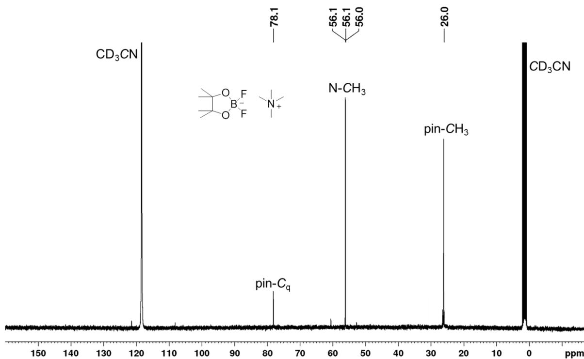
**Figure S22.**  $^{13}\text{C}\{\text{H}\}$  NMR spectrum of  $[\text{pinBF}_2][\text{NMe}_4]$  **6** recorded in  $\text{CD}_3\text{CN}$  (100 MHz).
