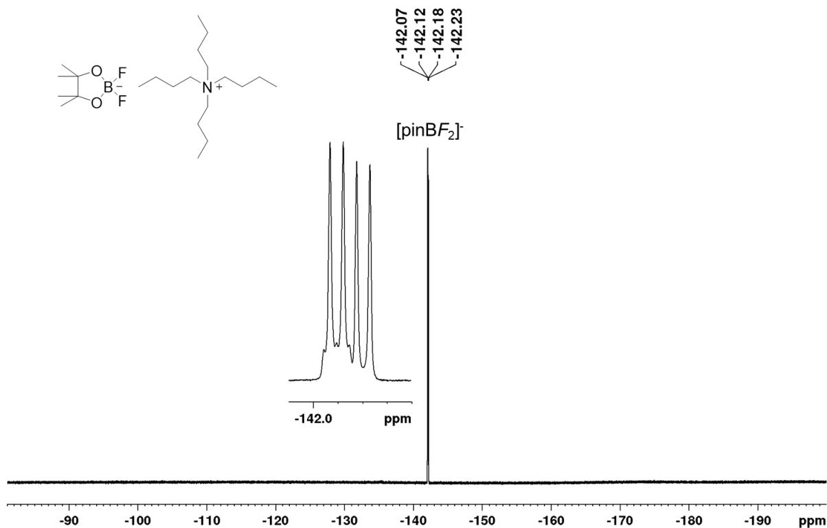
**Figure S28.**  $^{19}\text{F}\{\text{H}\}$  NMR spectrum of  $[\text{pinBF}_2]\text{[NnBu}_4\text{]} 7$  recorded in  $\text{CD}_3\text{CN}$  (376 MHz).
