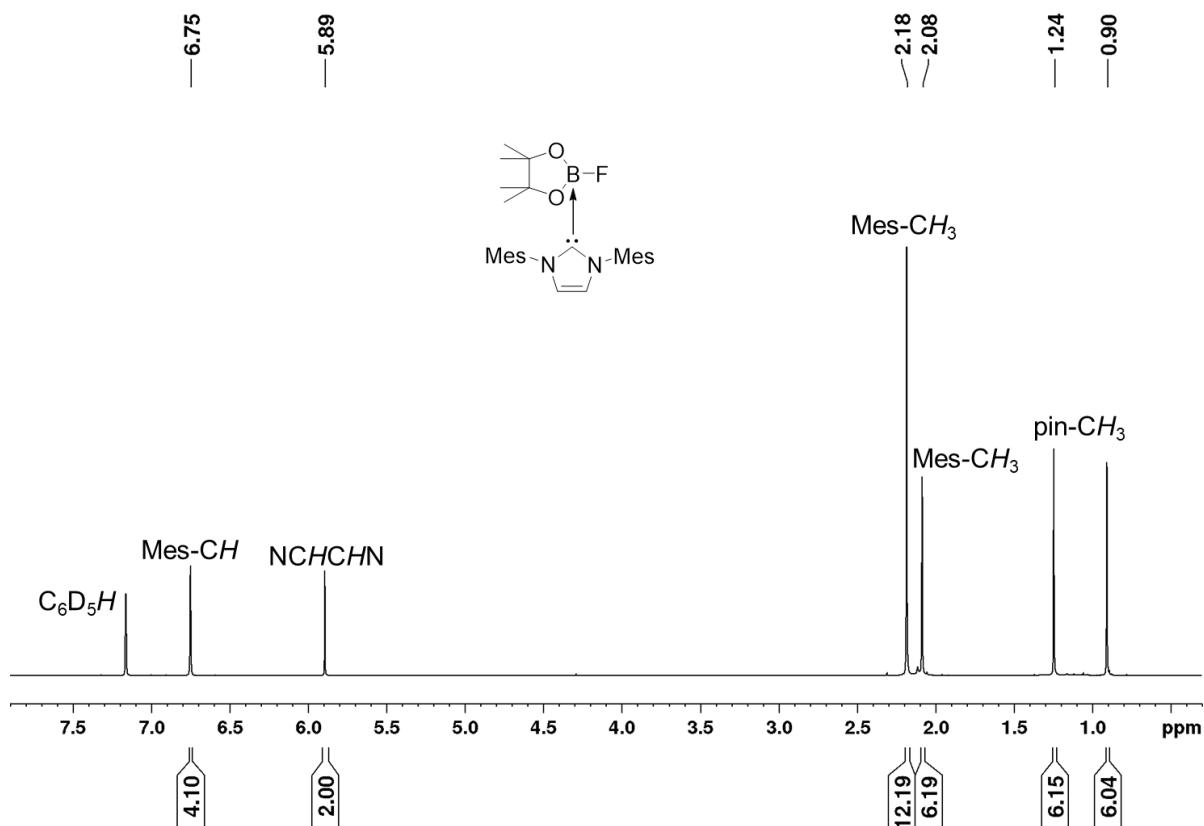
**Figure S17.**  $^1\text{H}$  NMR spectrum of FBpin·Mes<sub>2</sub>Im **5** recorded in  $\text{C}_6\text{D}_6$  (500 MHz).
