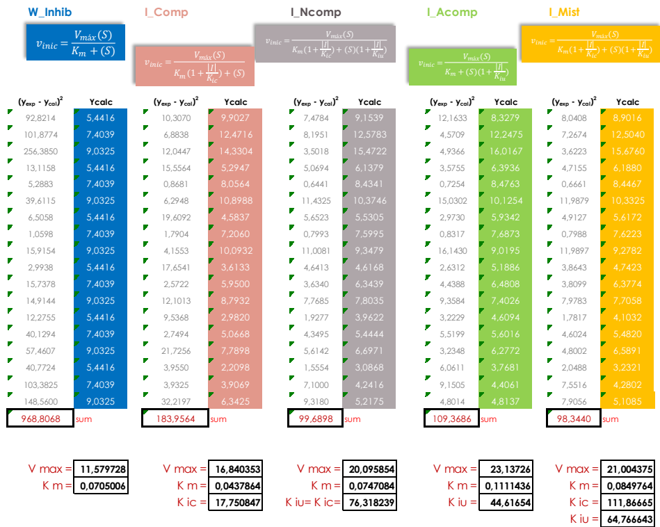
Figure 2S: Sum of the squares (sum) of the different models (without inhibition, competitive inhibition, noncompetitive inhibition, uncompetitive inhibition and mixed inhibition) from the results obtained from DPP-4 inhibition by flavonoid C11 .
