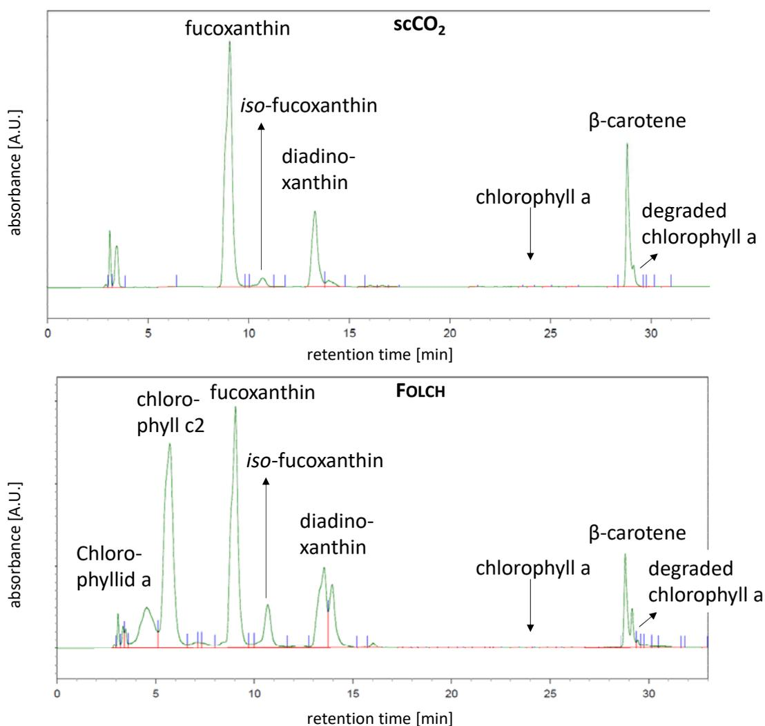
**Figure S17** Typical chromatogram of algae oil extracted according to Folch (bottom) and with scCO<sub>2</sub> (top). Oil extracted by scCO<sub>2</sub> does not contain polar chlorophylls. Chlorophyll a is not found in both oils, as it is degraded by the highly active chlorophyllase a in *P. tricornutum*.<sup>13,14</sup>
