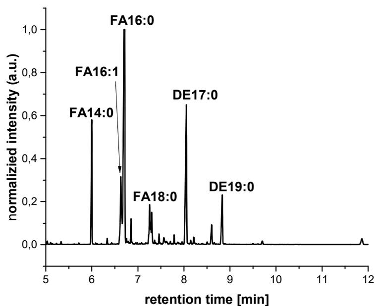
**Figure S26** Typical gas chromatogram of a post-alkoxyacylation mixture of crude freeze-dried algae (*P. tricornutum*).
