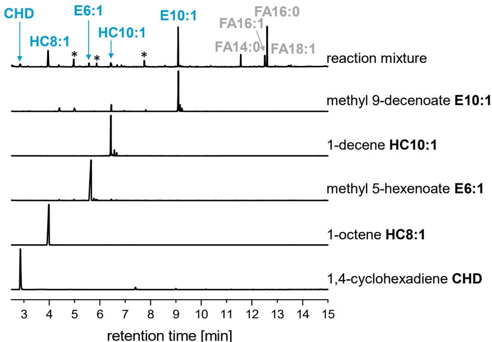
**Figure S21** Gas chromatogram of the ethenolysis of  $\text{scCO}_2$  extracted algae oil in  $\text{scCO}_2$  (after transesterification with methanol) with Hoveyda-Grubbs 1<sup>st</sup> generation catalyst (top) and gas chromatograms of genuine samples of the ethenolysis products and the self-metathesis product 1,4-cyclohexadiene CHD for identification. Side-products likely originating from ethyl vinyl ether are labelled with an asterisk.
