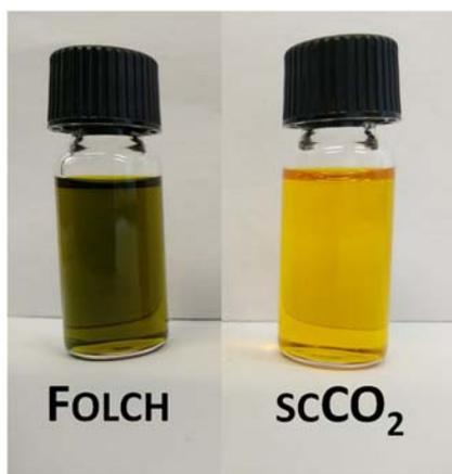
**Figure S7** Appearance of algae oils extracted according to Folch and with  $scCO_2$ , respectively, diluted in  $CH_2Cl_2$ , showing the differences in pigment extraction. The Folch extraction also extracts chlorophylls, while  $scCO_2$  extracts carotenoids selectively (cf. section 5.5).
