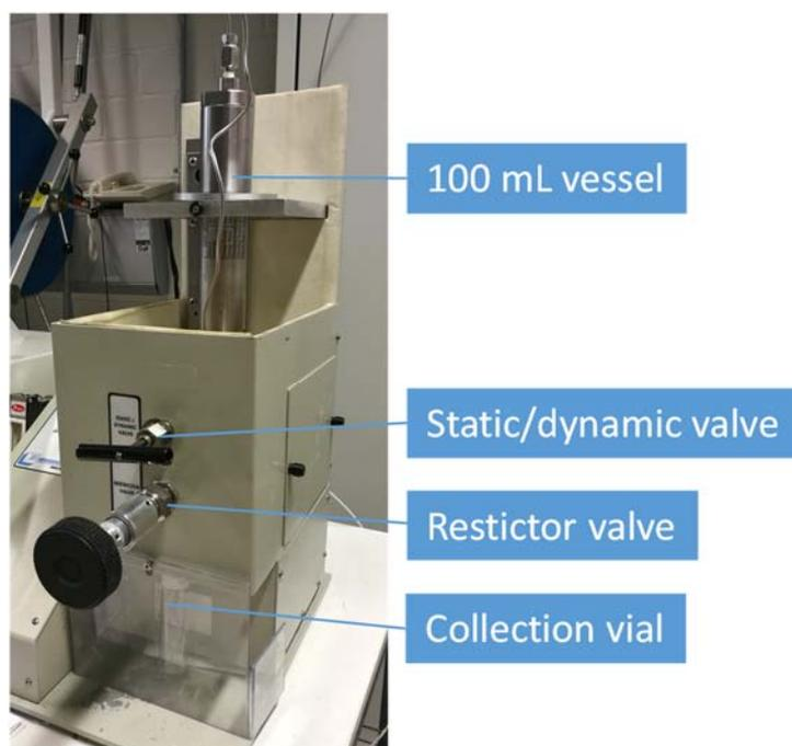
**Figure S2** Supercritical fluid extractor SFX-110W.
