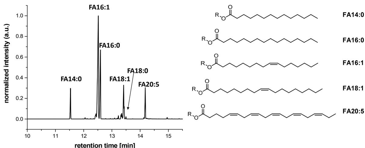
**Figure S5** Gas chromatogram of algae oil from *P. tricornutum* extracted via the method of Folch.<sup>4</sup> The sample was transesterified with methanol for gas chromatography.
