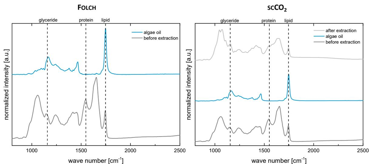
**Figure S14** FT-IR spectra of algae oil extracted according to Folch (left) and with  $\text{scCO}_2$  (right), respectively, and of *P. tricornutum* biomass prior to and after extraction.
