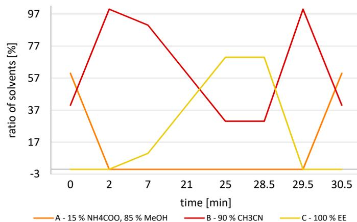
**Figure S16** Gradient profile of the HPLC separation method. A – 85 % MeOH/15 % 0.5 M NH<sub>4</sub>CH<sub>3</sub>COO, B – 90 % acetonitrile/10 % H<sub>2</sub>O, C – 100 % ethyl acetate.
