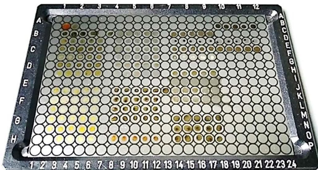
**Figure S13** Silica plate with algae oil samples, always applied in >5 technical replicates. The right (A to P) and bottom (1 to 24) labeling applies here.
