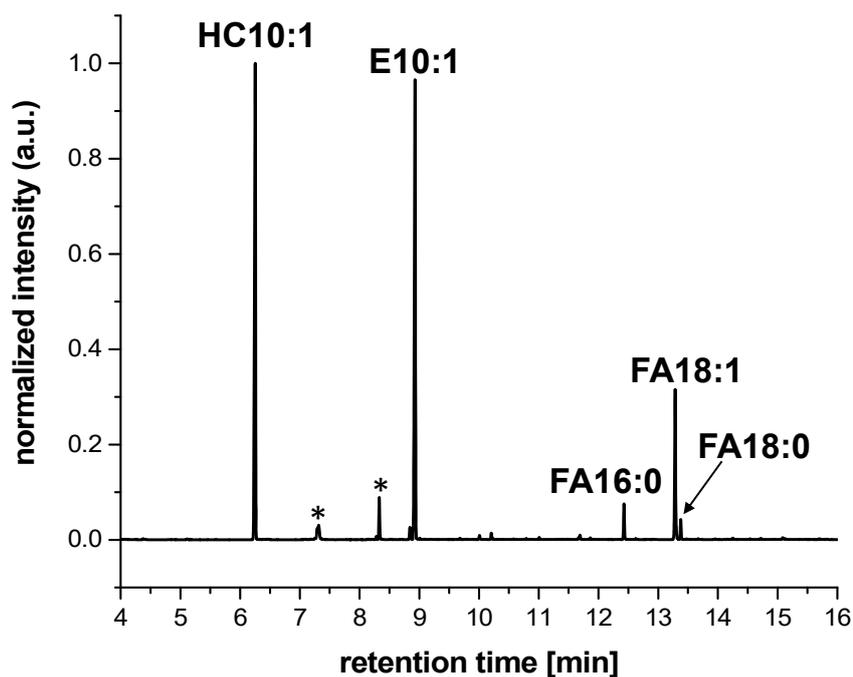
**Figure S19** Gas chromatogram of the reaction mixture of ethenolysis in  $scCO_2$  of methyl oleate with 0.5mol% Hoveyda-Grubbs 1<sup>st</sup> generation catalyst. The starting material (FA18:1 methyl oleate) and the ethenolysis products (E10:1 methyl 9-decenoate, HC10:1 1-decene) are labelled. Side-products likely originating from ethyl vinyl ether are labelled with an asterisk.
