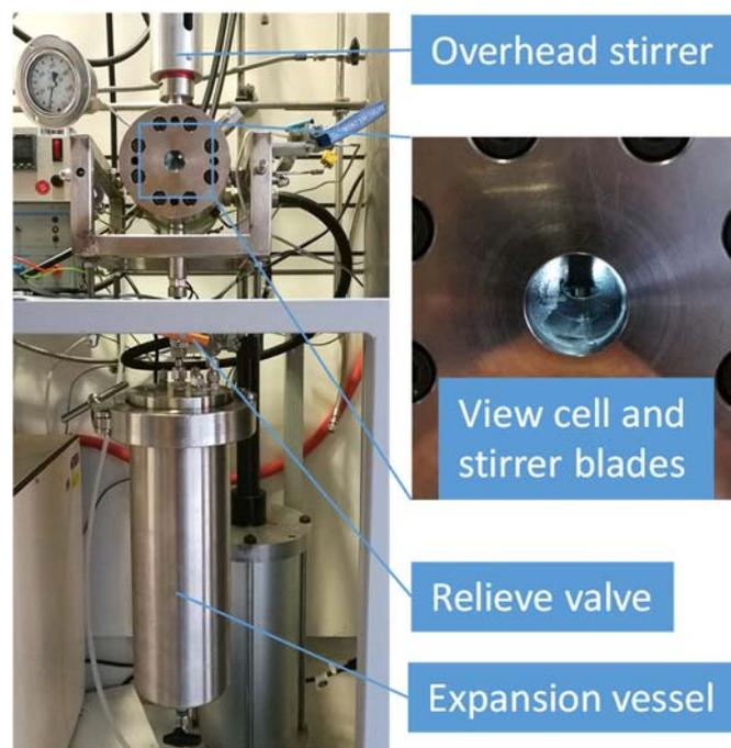
**Figure S1** High-pressure reactor employed.
