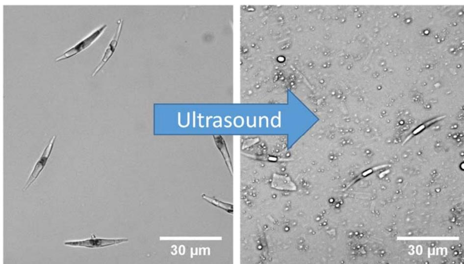
**Figure S4** Light microscopy images of *P. tricornutum* before (left) and after cell disruption by ultrasound (right). The images were recorded on an Olympus BX 51 equipped with a Zeiss AxioCam MRm. Visible droplets can be attributed to intracellular and extracellular lipid droplets.
