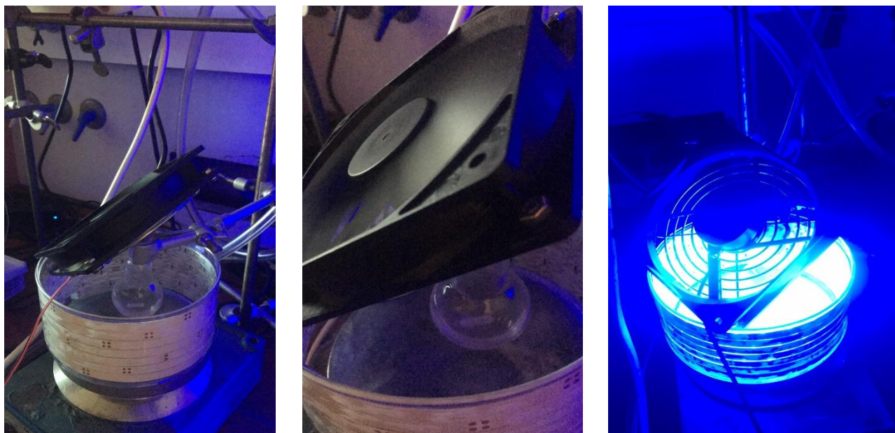
Figure S1: LED reaction setup for photocatalytic reactions.
