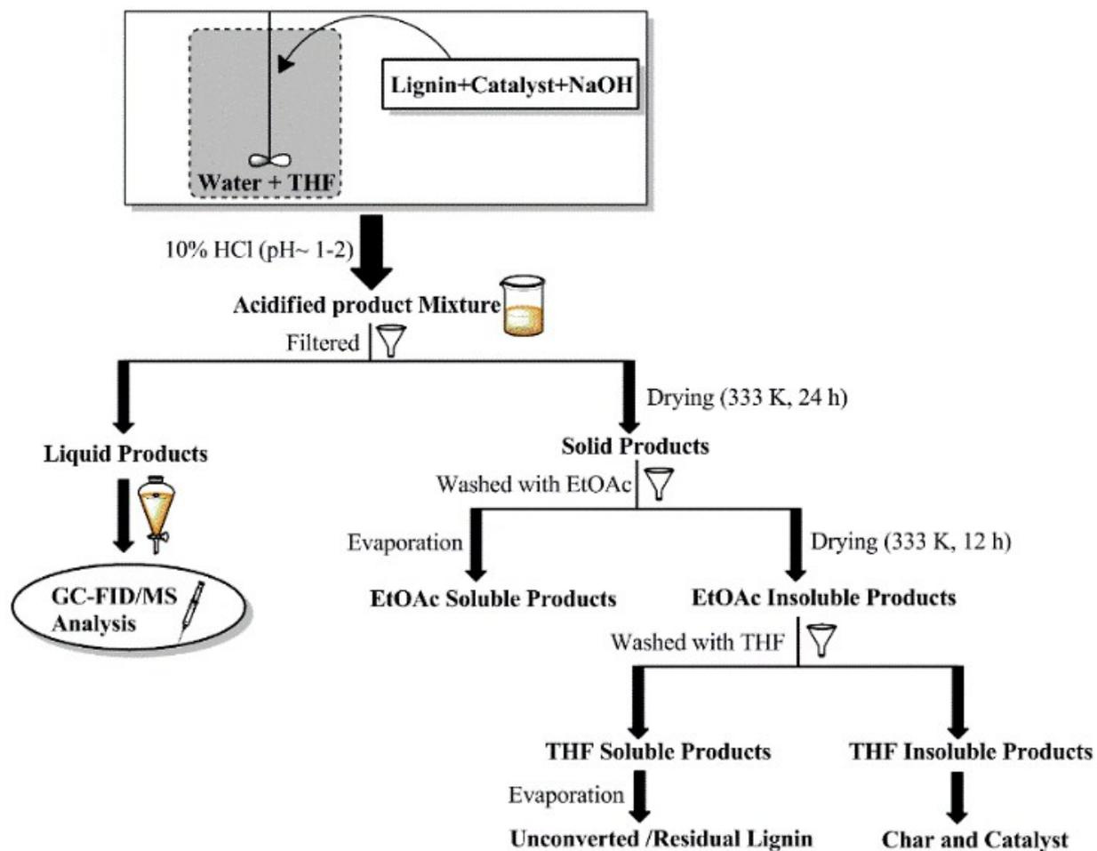
**Figure S2** Workup procedure for separation of depolymerized products.
