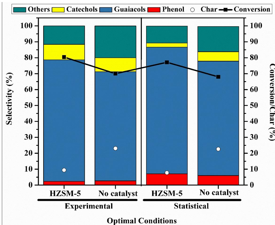
**Figure S17** Experimental trails at the optimal condition obtained in experimental and statistical sensitivity analysis in the presence and absence of HZSM-5. Reaction conditions: Statistical Optimal: 12g lignin, HZSM280, lignin-to-solvent ratio (1:16.6 w/v), water-to-THF (0.86:1 v/v), NaOH (1.2g), Time (2h), Temperature (533 K), RPM (800). Experimental Optimal: 12g lignin, HZSM280, lignin-to-solvent ratio (1:16.6 w/v), water-to-THF (0.8:1 v/v), Time (2h), Temperature (523 K), RPM (800).
