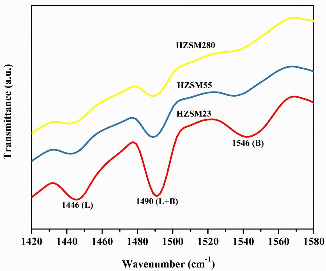
Figure S5 Pyridine FTIR spectra of HZSM-5.
