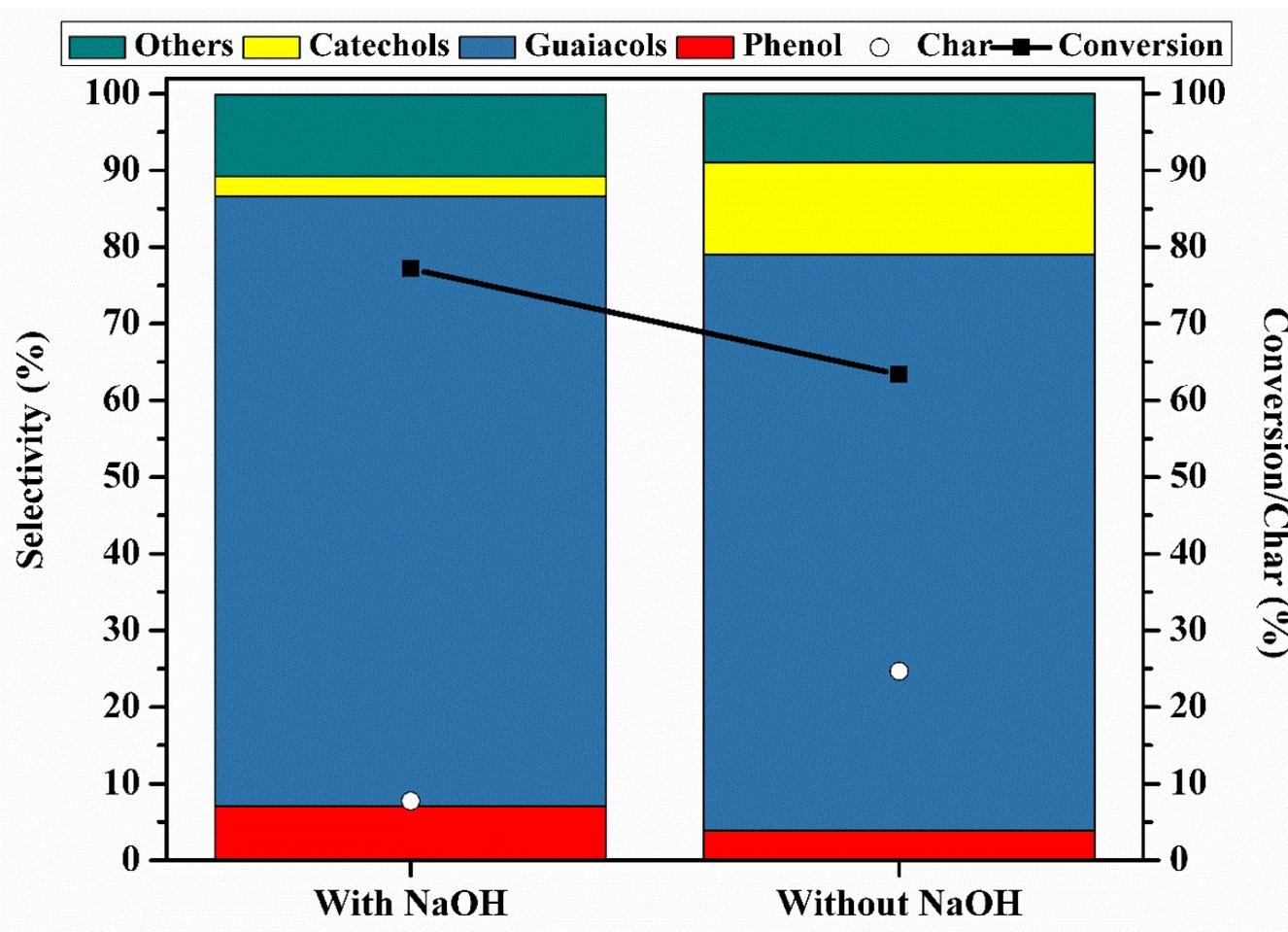
**Figure S16** Product distribution obtained during the lignin depolymerization reaction in the presence and absence of NaOH. Reaction conditions (Optimal): 12g lignin, HZSM280 (2g), lignin-to-solvent ratio (1:16.6 w/v), water-to-THF (0.86:1 v/v), NaOH-to-lignin ratio=0.1, Time (2h), Temperature (533 K), RPM (800).
