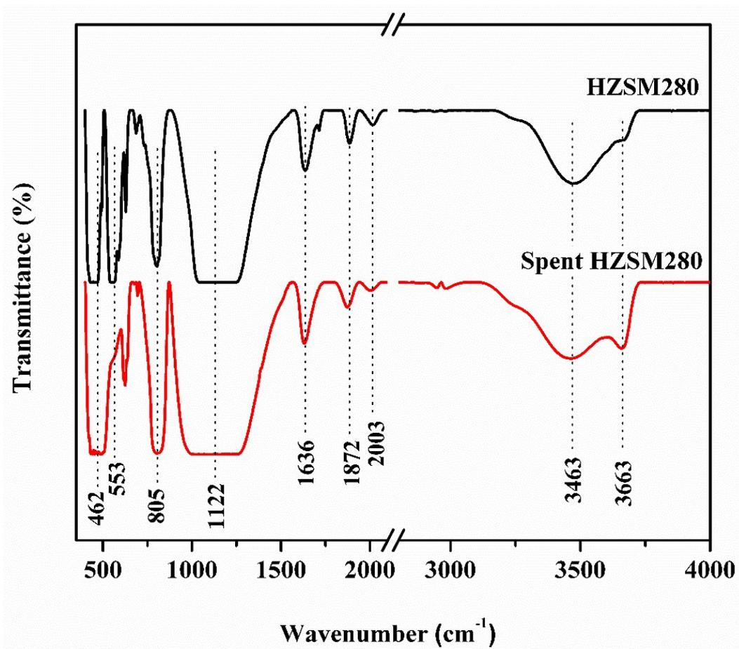
Figure S19. FTIR spectra of fresh and spent HZSM280.
