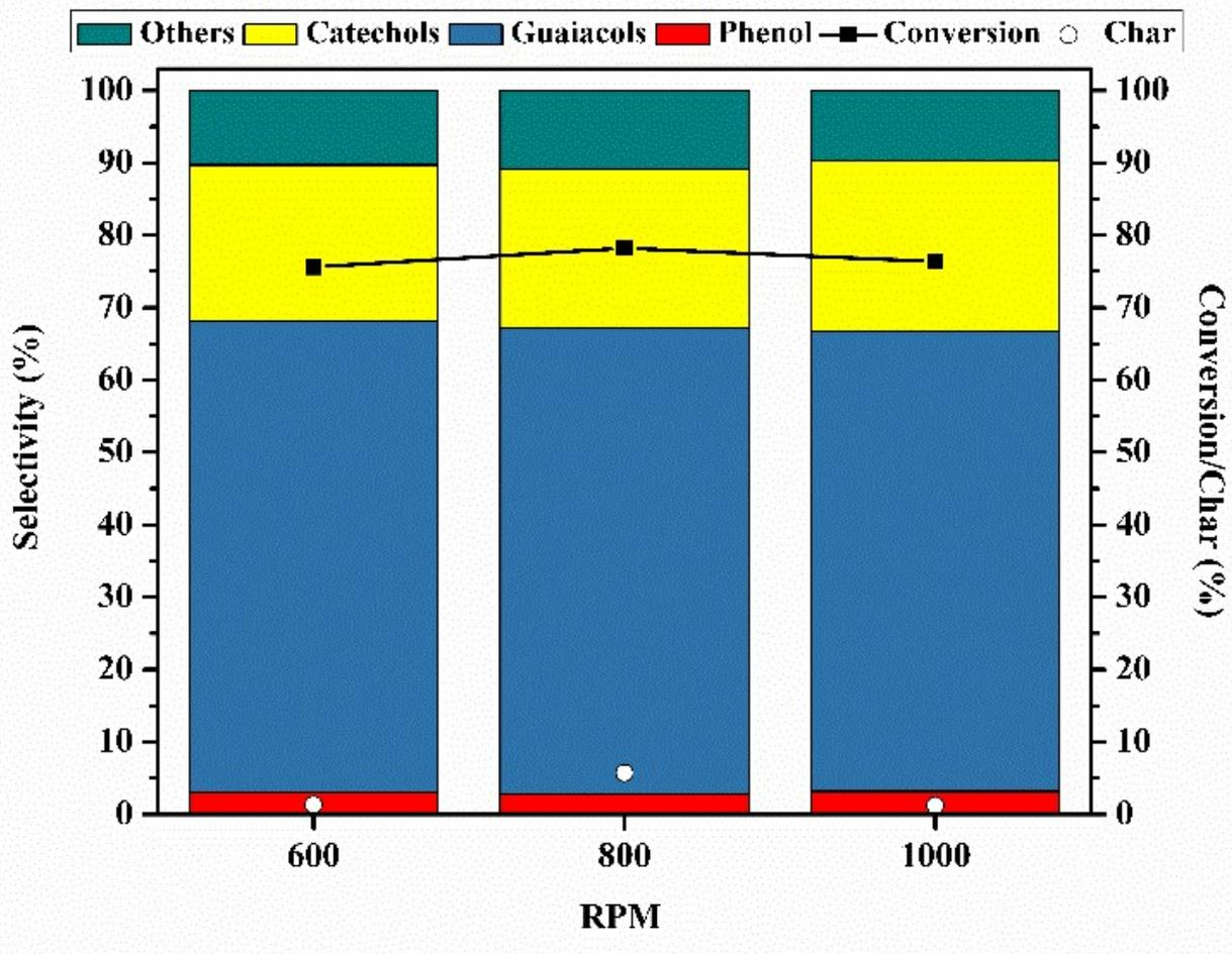
**Figure S1(a)** Effect of stirrer speed on lignin depolymerization. Reaction conditions: 12g lignin, HZSM55 (1.2g), NaOH (1g), lignin-to-solvent ratio (1:15.0 w/v), water-to-THF ratio (1:1 v/v), Temperature (533 K), Time (2h).
