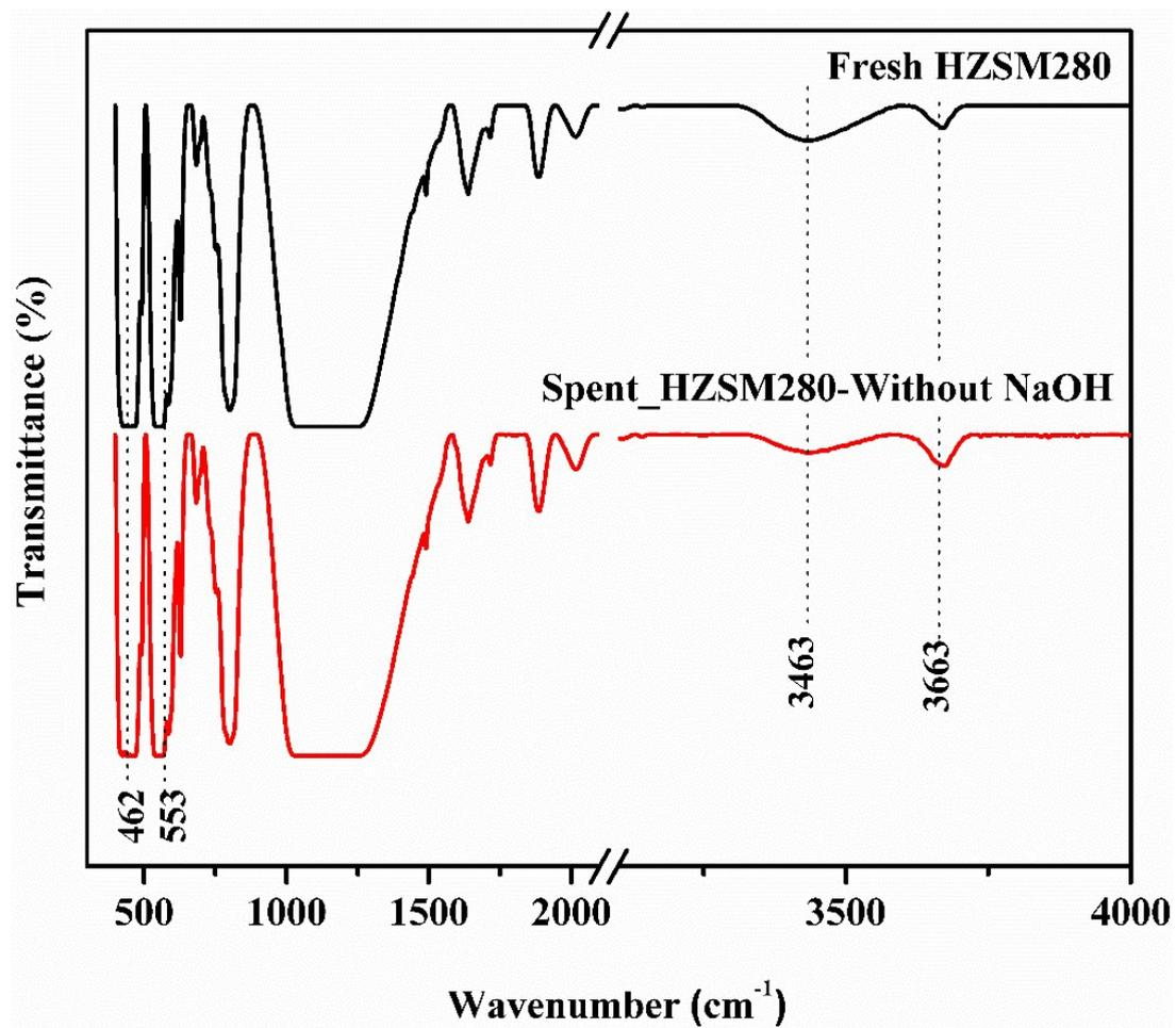
**Figure S18(b)** FT-IR spectra of parent and spent HZSM280 after lignin depolymerization reaction in the absence of NaOH.
