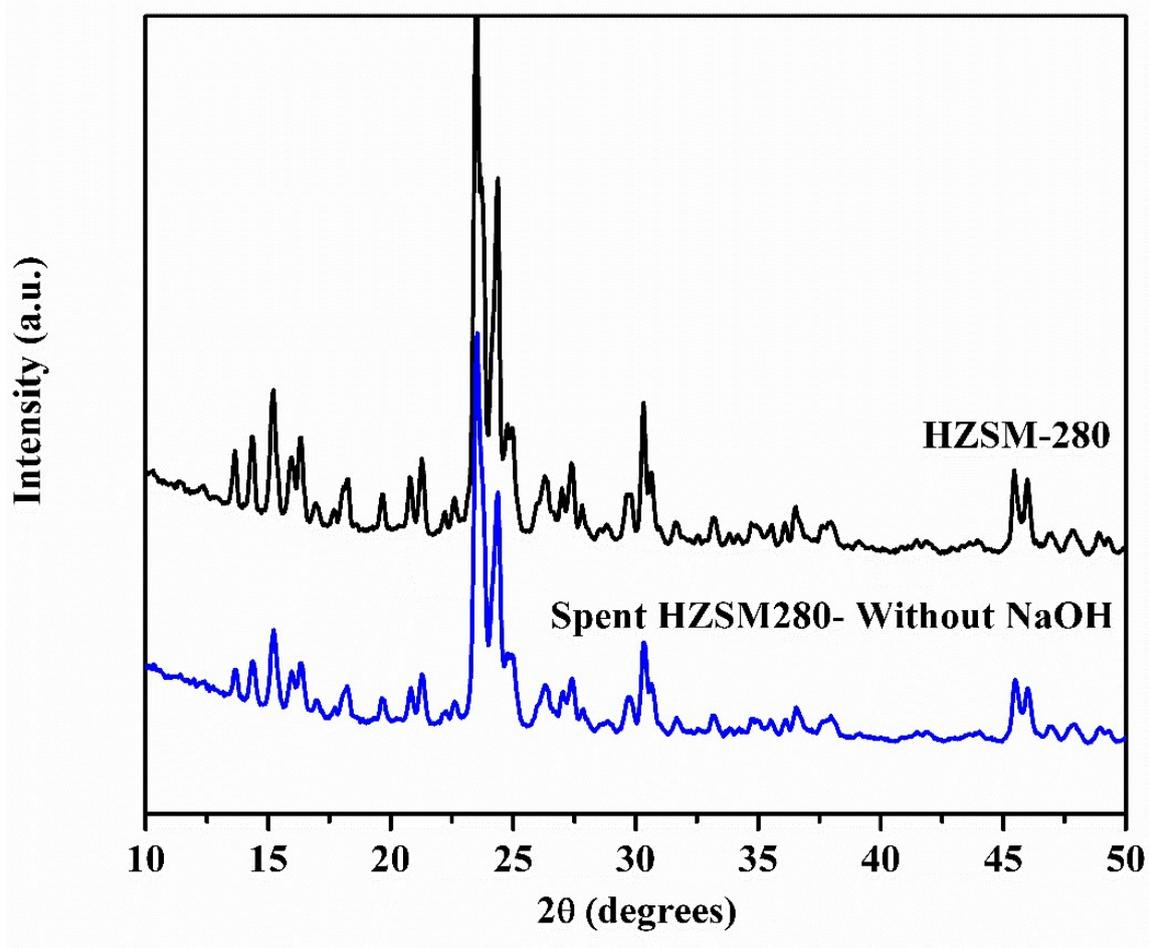
**Figure S18(a)** XRD pattern of parent and spent HSM280 after lignin depolymerization reaction in the absence of NaOH.
