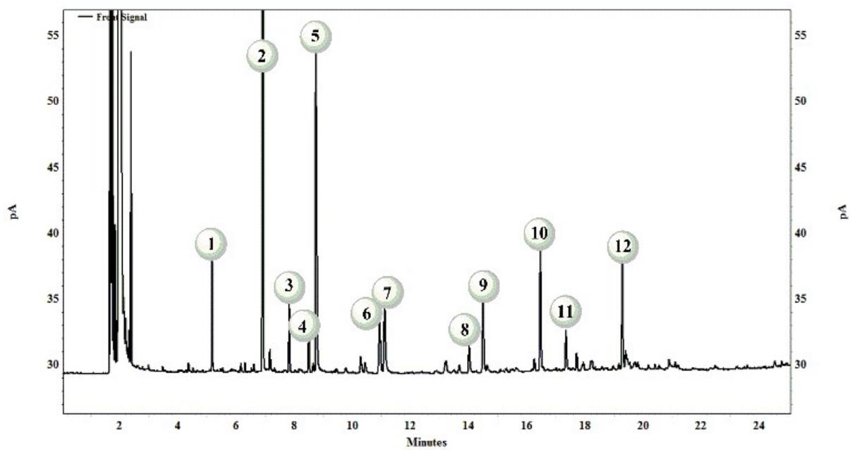
**Figure S8** GC-FID chromatogram for EtOAc soluble products. Reaction Conditions: 12g lignin, HZSM280 (1.2g,) NaOH (1g), lignin-to solvent ratio (1:15.0 w/v), water-THF ratio (0.8:1 v/v), Temperature (533 K), Time (2h), RPM (800).
