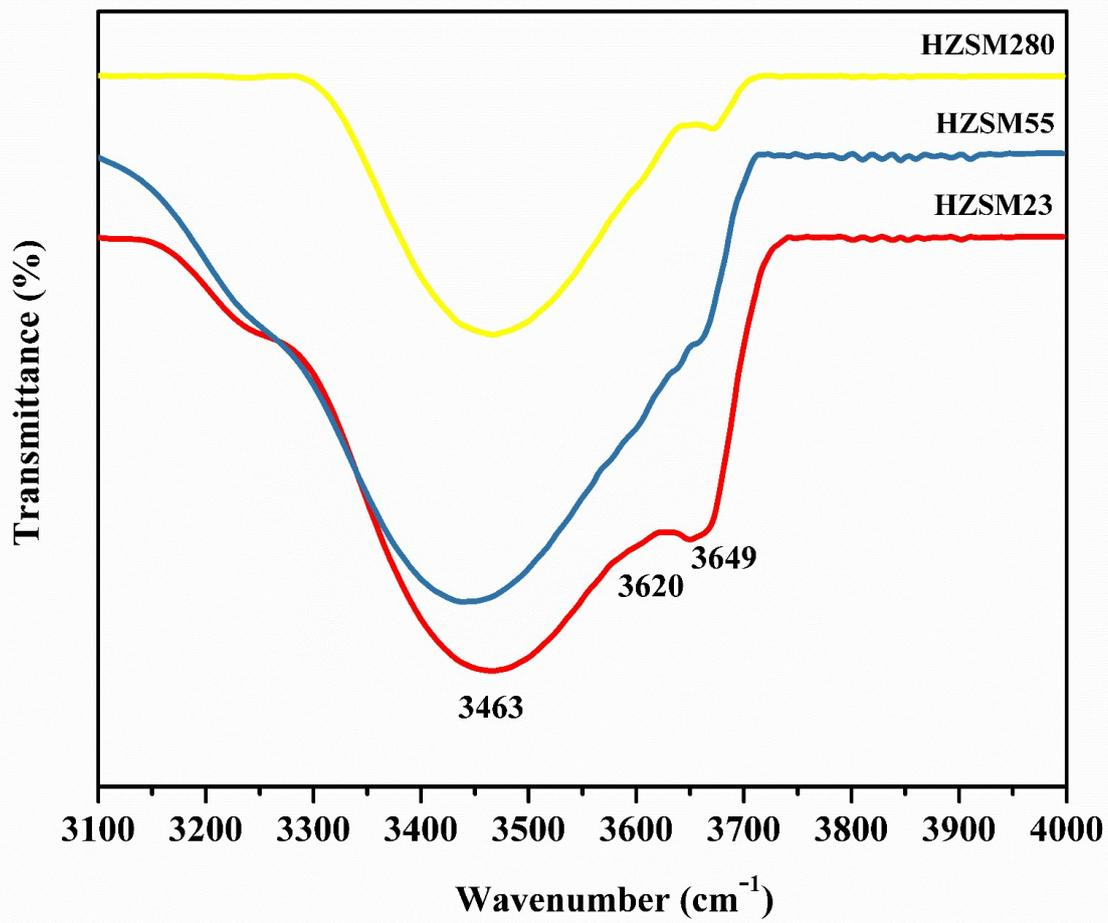
**Figure S6** FTIR spectra of HZSM-5 catalyst.
