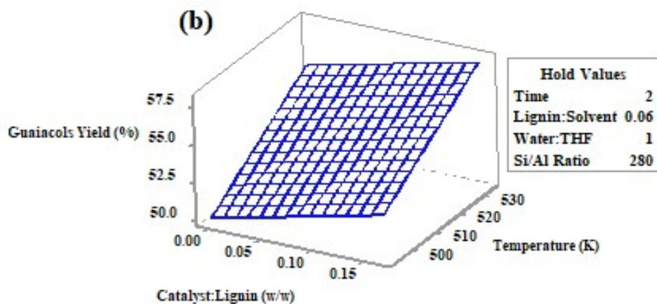
**Figure S13** Countours (a) and surface plots (b) representing effect of catalyst-to-lignin (w/w) ratio and Temperature (K) on guaiacol yield (%).
