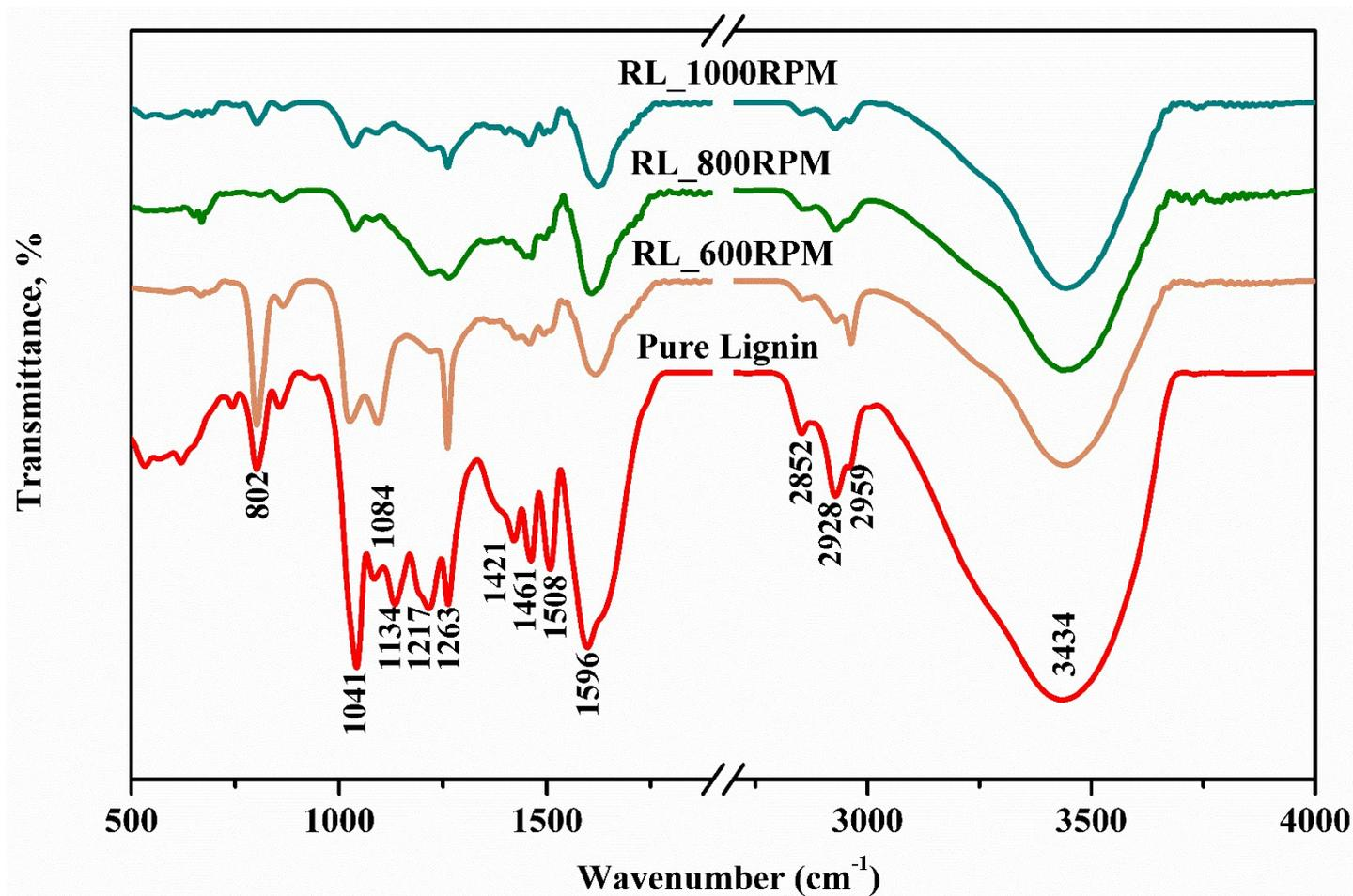
**Figure S1(b)** FTIR spectra of fresh lignin and resultant residual lignin after depolymerization reaction at different stirrer speed. Reaction conditions: 12g lignin, HZSM5-55 (1.2g), NaOH (1g), lignin-to-solvent ratio (1:15.0 w/v), water-to-THF ratio (1:1 v/v), Temperature (533 K), Time (2h).
