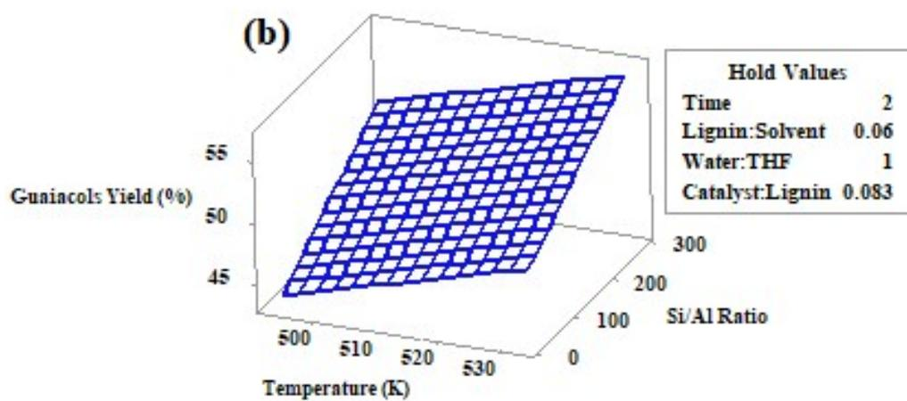
**Figure S14** Countours (a) and surface plots (b) representing effect of Temperature (K) and Si/Al ratio of HZSM5 on guaiacol yield (%).
