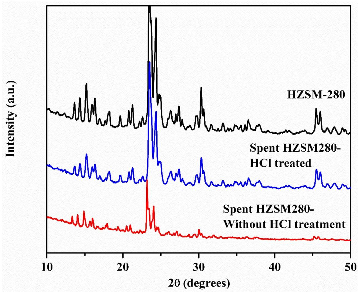
**Figure S3(a)** XRD pattern of parent and spent HSM280 with and without acidification process.
