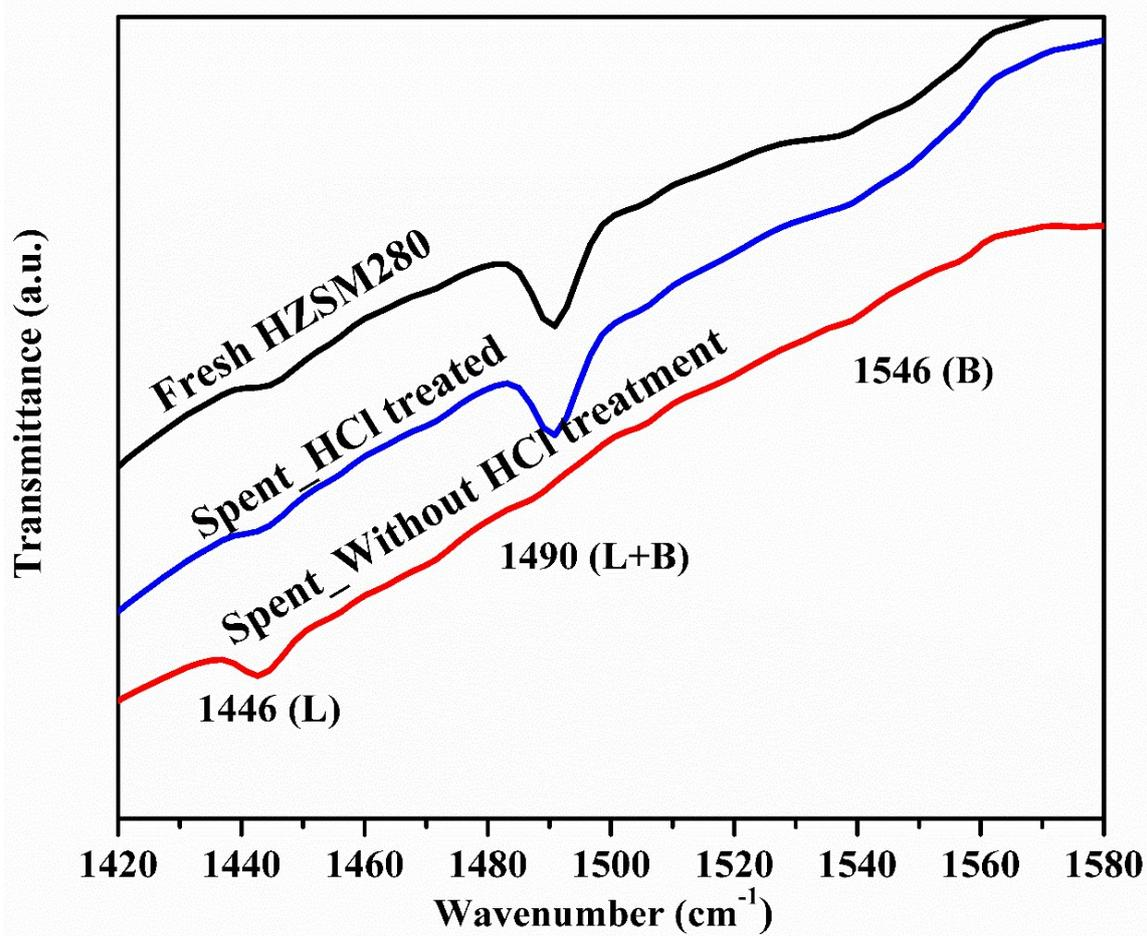
**Figure S3(b)** Pyridine FTIR spectra of parent HZSM280 and spent HSM280 with and without acidification process.
