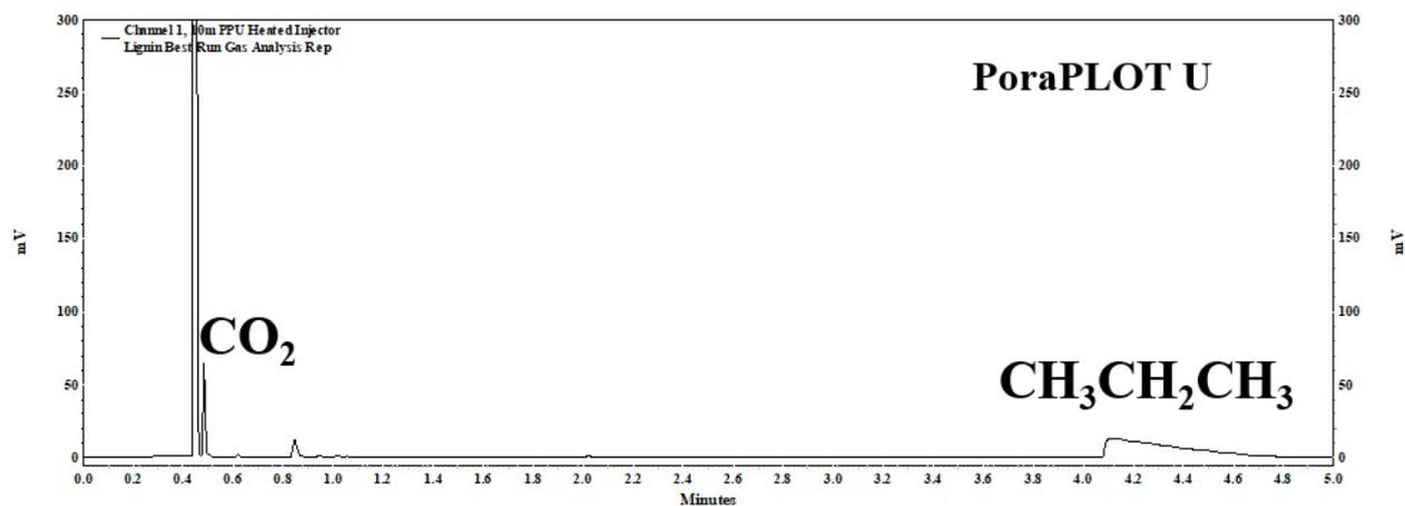
**Figure S9** Micro GC- TCD chromatogram of gaseous products generated during lignin depolymerization Reaction conditions: 12g lignin, HZSM280 (1.2g), NaOH (1g), lignin-to-solvent ratio (1:15.0 w/v), water-to-THF ratio (1:1 v/v), Temperature (533K), Time (2h), RPM (800).
