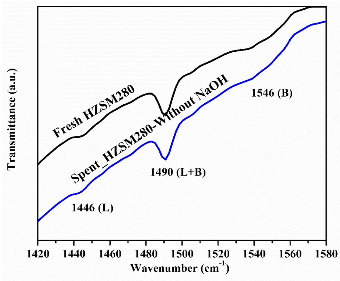
**Figure S18(c)** Pyridine absorbed FT-IR spectra of parent and spent HZSM280 after lignin depolymerization reaction in the absence of NaOH.
