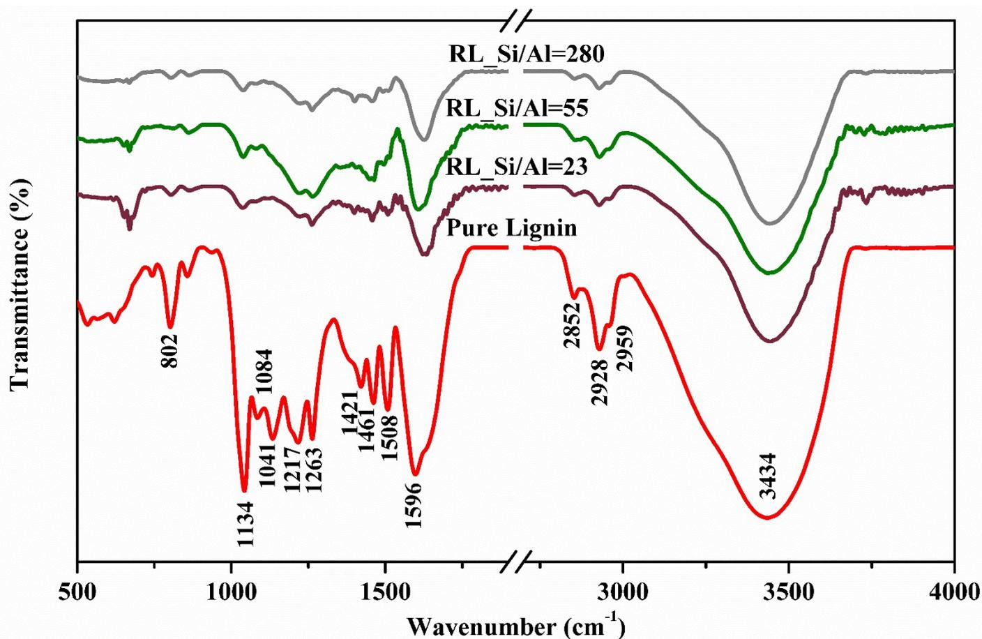
**Figure S10** FTIR spectra of fresh lignin and resultant residual lignin after depolymerization reaction at different Si/Al ratio of HZSM-5. Reaction conditions: 12g lignin, HZSM-5 (1.2g), NaOH (1g), lignin-to-solvent ratio (1:15.0 w/v), water-to-THF ratio (1:1 v/v), Temperature (533 K), Time (2h), RPM (800).
