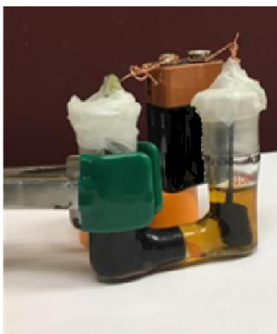
Figure S2. Electrochemical H-Cell used to perform reactions described in the manuscript. Reticulated Vitreous Carbon electrodes were employed as cathode and anode. Electrolysis is carried out by connecting the electrodes to a commercially available battery.
