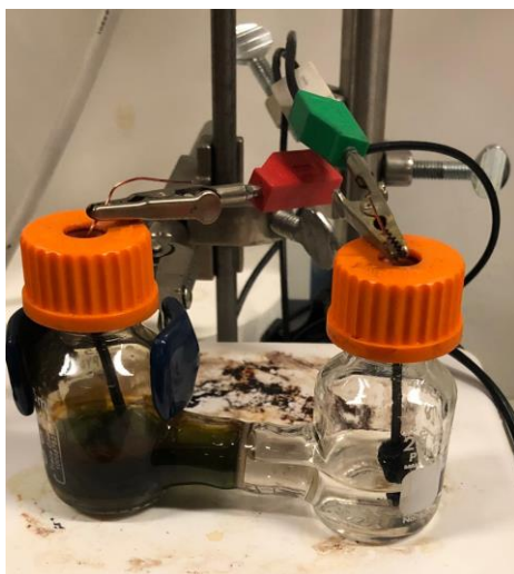
Figure S1. Electrochemical H-Cell used to perform reactions described in the manuscript. Reticulated Vitreous Carbon electrodes were employed as cathode and anode.
