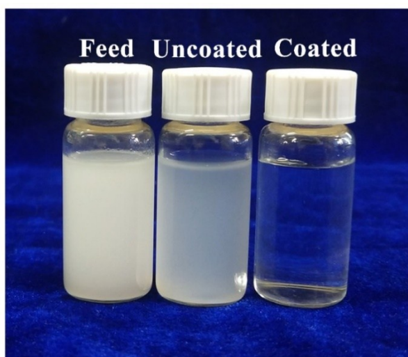
Fig. S13. The digital images of the kerosene-in-water emulsion before and after one-time separation by the original PVDF membrane (the middle vial) and the loess-coated membrane (the right vial).
