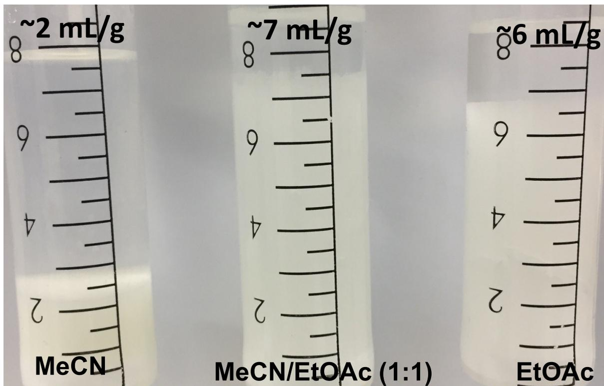
Figure S1. Swelling of a PS/DVB resin in MeCN, EtOAc and MeCN/EtOAc (1:1).
