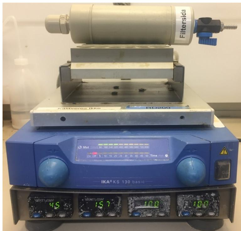
Figure S4. Sealed SPPS reactor on an IKA® KS basic 130 apparatus.
