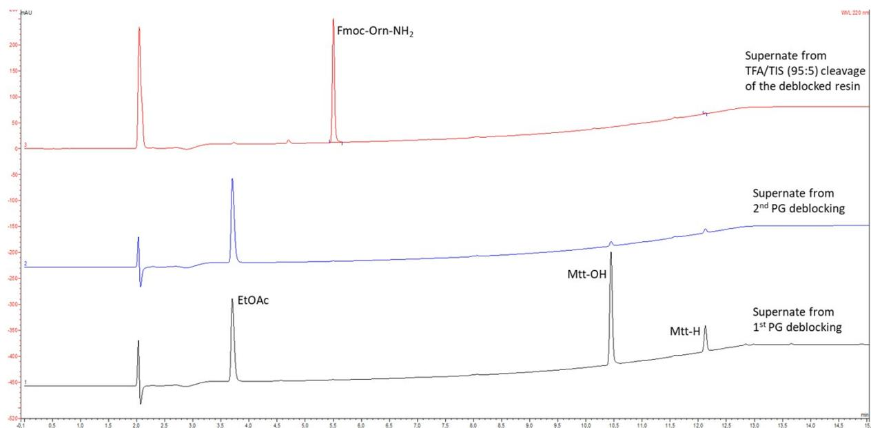
**Figure S3.** HPLC analysis of Table 1, entry 14 deblocking of Fmoc-Orn(Mtt)-RMG AMS resin. Content of Fmoc-Orn-NH<sub>2</sub> in supernates in 1<sup>st</sup> + 2<sup>nd</sup> deblockings: 0.09 mAu $\times$ min (0.7%). Content of Mtt-H + Mtt-OH in the supernate from TFA/TIS (95:5) cleavage after Mtt deblocking: 0.04 mAu $\times$ min (0.2%).
