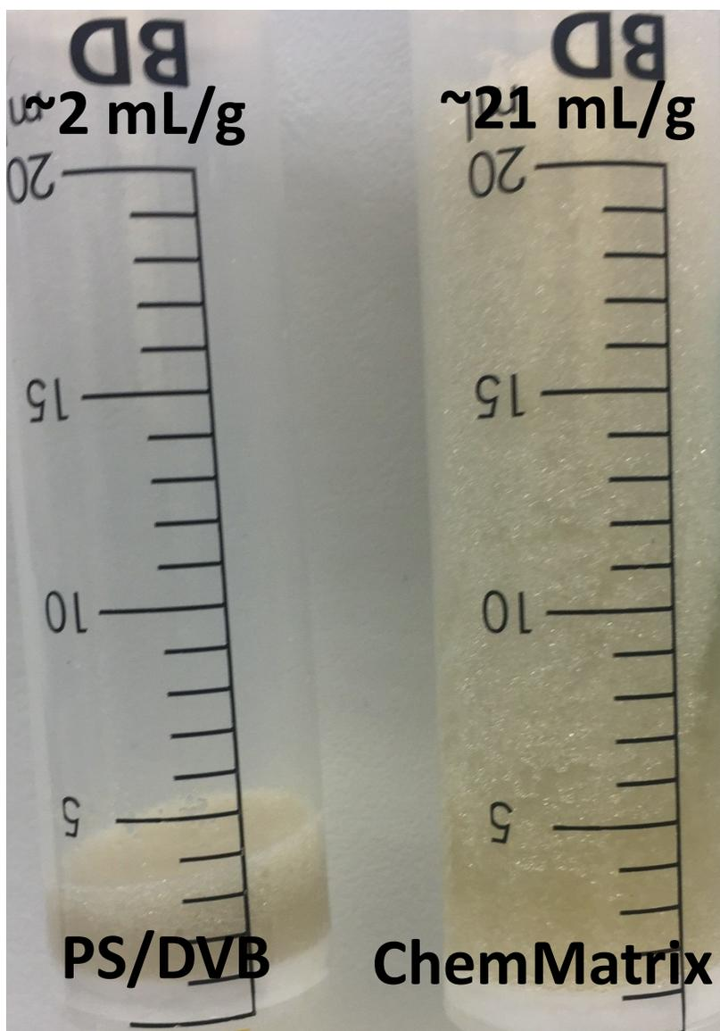
**Figure S2.** Swelling of a PS/DVB resin and a ChemMatrix resin in TFA.
