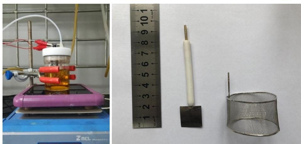
**Fig. S5:** Electrosynthetic installation for gram scale
