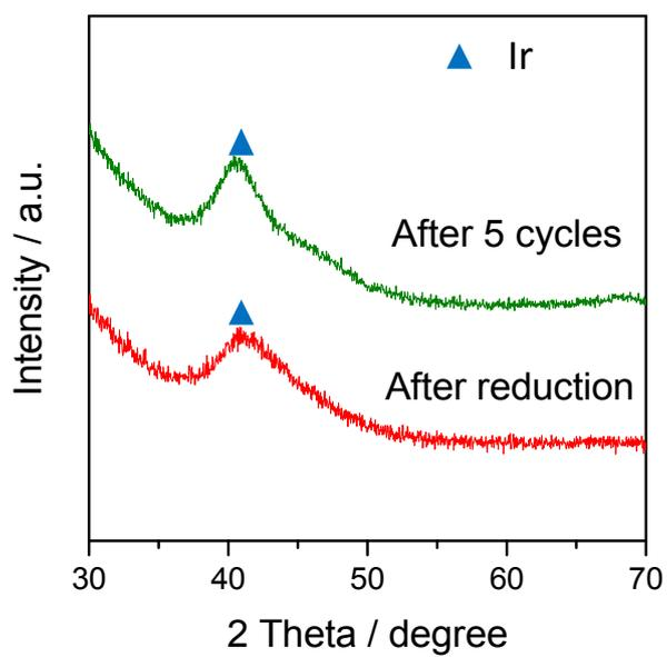
**Fig. S2** XRD patterns of the Ir-ReO<sub>x</sub>/SiO<sub>2</sub> (Re/Ir=2) catalyst. a: after reduction, b: after 5 cycles.
