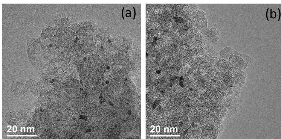
**Fig. S3** TEM images of the Ir-ReO<sub>x</sub>/SiO<sub>2</sub> (Re/Ir=2) catalyst. (a): after reduction, (b): after 5 cycles.
