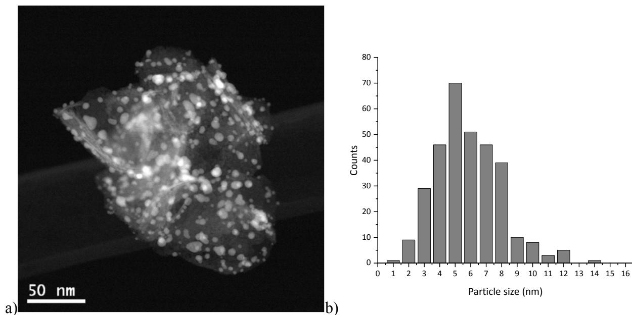
**Figure S2** a) STEM-HAADF image of fresh Pd-nNiO and b) particle size distribution.
