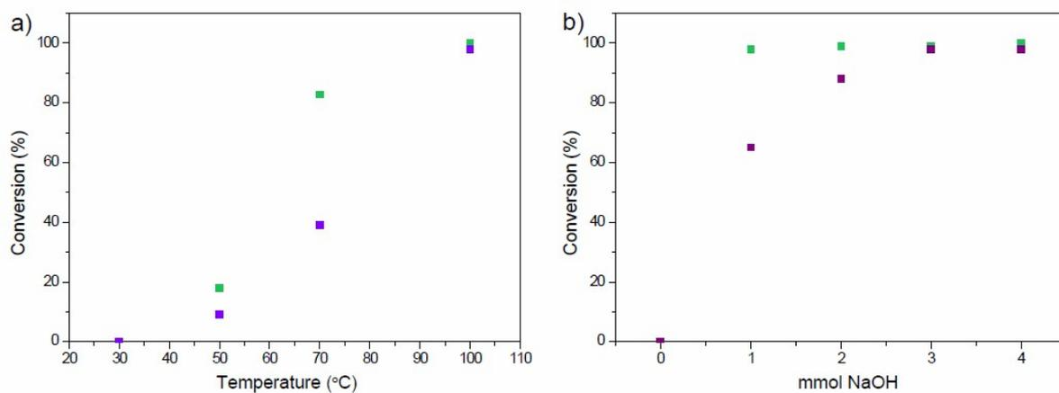
Figure S8. Optimization in a) temperature and b) base amount of the SM cross-coupling reaction for GA-Pd-100 (green) and GO-Pd-100 (purple) between bromobenzene and phenylboronic acid.
