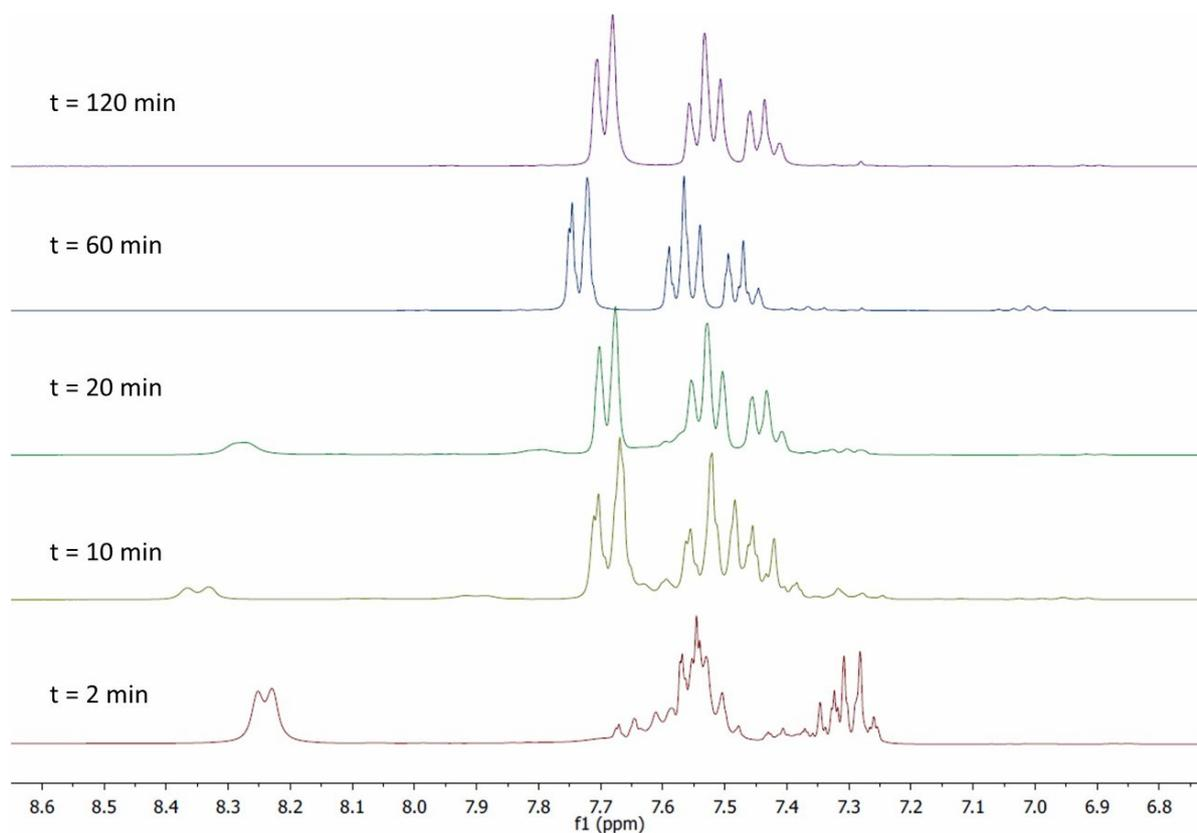
Figure S6. NMR tracking ( $\text{CDCl}_3$ , 300.1 MHz, 298 K) of the SM coupling between bromobenzene and phenylboronic acid (standard conditions) catalysed by GA-Pd-100.
