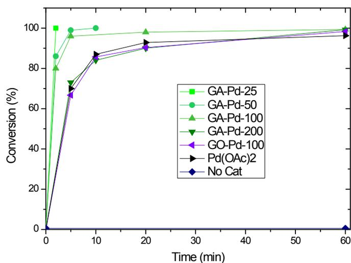
Figure S7. Kinetic profiles of the SM cross-coupling reaction between bromobenzene and phenylboronic acid (standard conditions).
