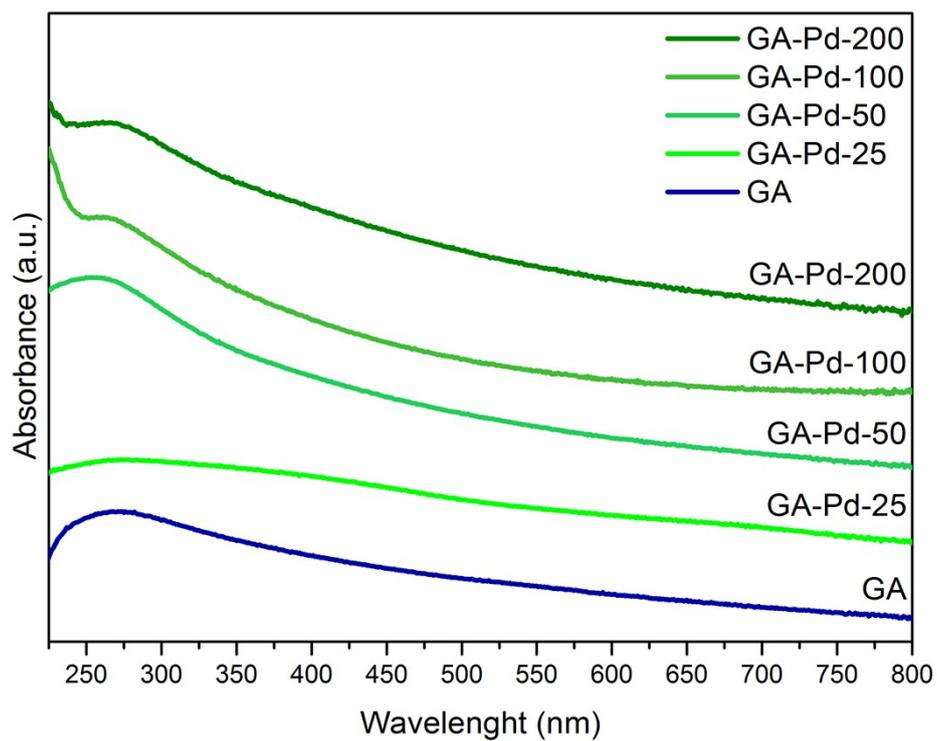
Figure S2. UV-Vis spectra of the different GA-Pd materials.
