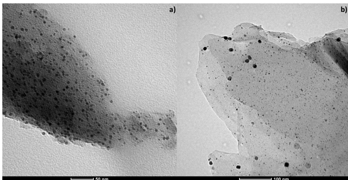
Figure S5. TEM image of a) GA-Pd-100 and b) GO-Pd-100 after 20 min of impregnation
