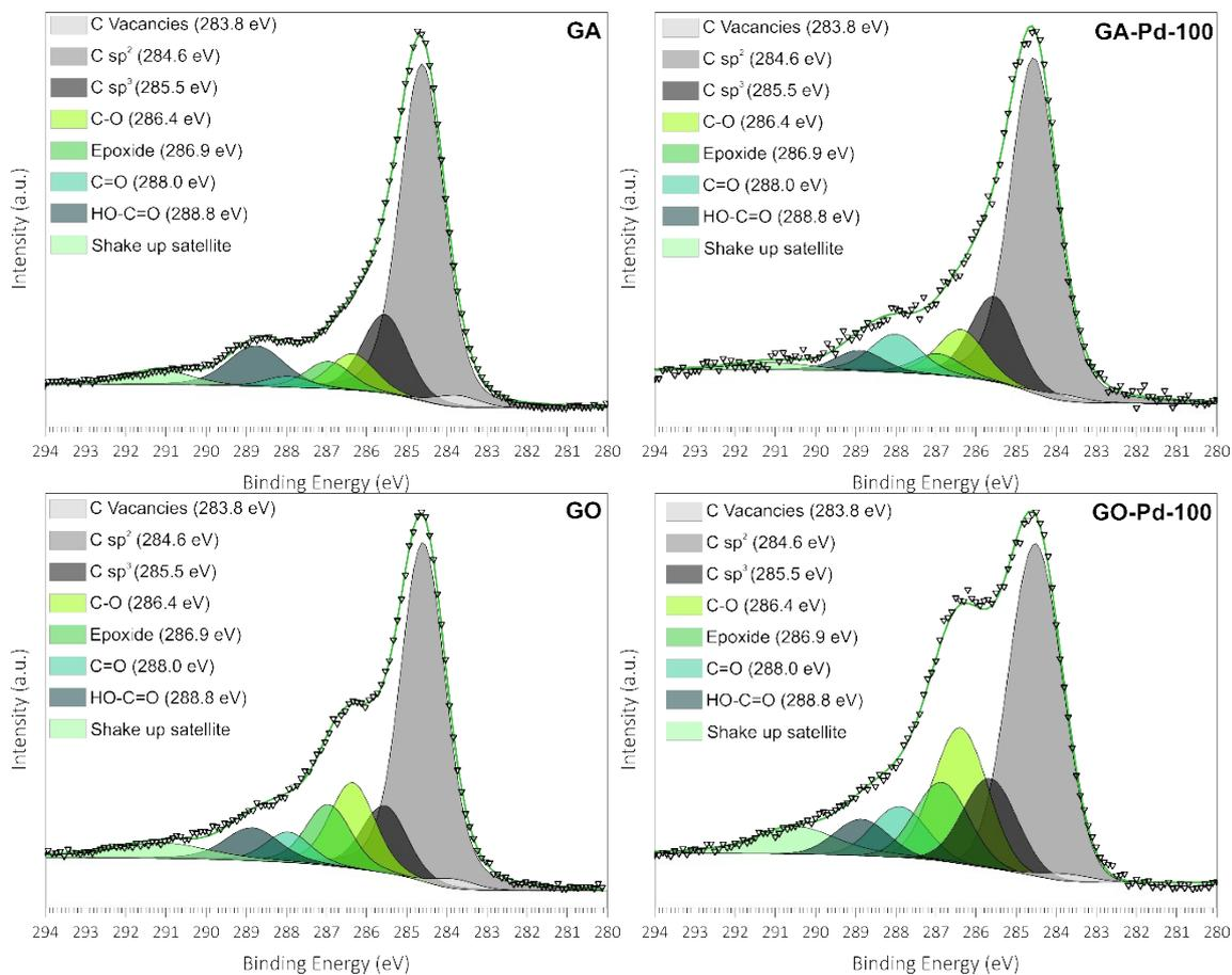
Figure S1. C 1s photoemission lines of pristine (left) and after impregnation (right) materials.
