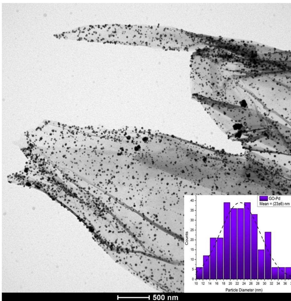
Figure S4. TEM image of GO-Pd-100. Inset: particle size distribution.
