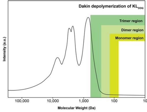
**Figure S11.** Mw distribution of  $KL_{DDQ}$  post Dakin depolymerization
