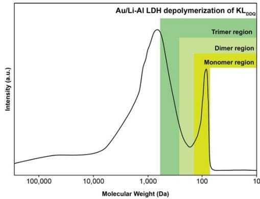
**Figure S15.** Mw distribution of  $KL_{DDQ}$  post Au/Li-Al LDH depolymerization
