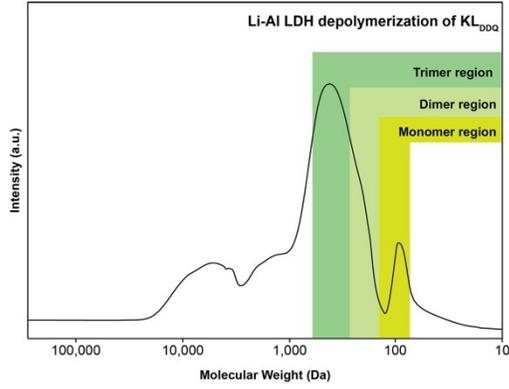
**Figure S13.** Mw distribution of  $KL_{DDQ}$  post Li-Al LDH depolymerization
