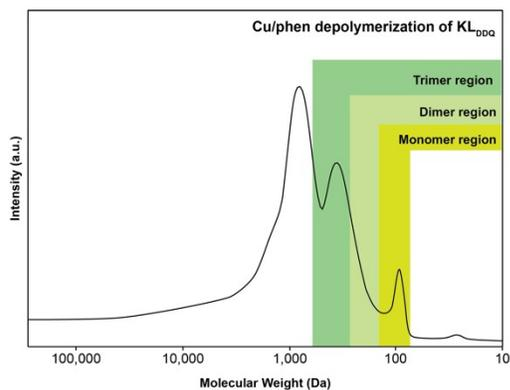
**Figure S9.** Mw distribution of  $KL_{DDQ}$  post Cu/phen depolymerization
