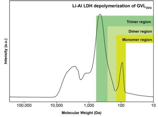
**Figure S14.** Mw distribution of  $GVL_{DDQ}$  post Li-Al LDH depolymerization
