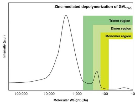
**Figure S4.** Mw distribution of GVL<sub>DDQ</sub> post zinc depolymerization
