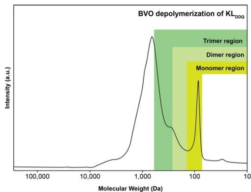
**Figure S7.** Mw distribution of  $KL_{DDQ}$  post BVO depolymerization
