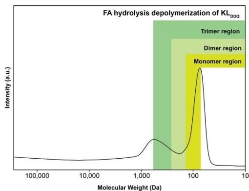
**Figure S5.** Mw distribution of  $KL_{DDQ}$  post FA hydrolysis depolymerization
