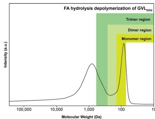
**Figure S6.** Mw distribution of  $GVL_{DDQ}$  post FA hydrolysis depolymerization
