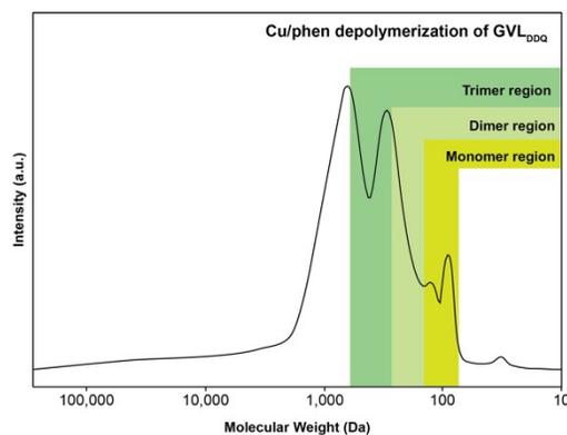
**Figure S10.** Mw distribution of  $GVL_{DDQ}$  post Cu/phen depolymerization
