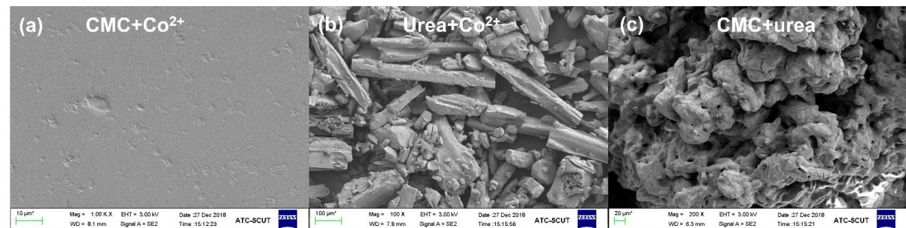
**Figure S2** SEM images of unpyrolyzed Co@NG-0 precursor (a), Co/Urea precursor (b), NC-6 precursor (c).
