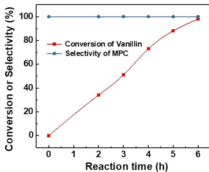
**Figure S8** Effect of reaction time on THD of vanillin. Reaction conditions: 0.5mmol vanillin in 10 mL water, 250 mg FA, 160 °C, Co@NG-6 catalyst (2.3 mol% metal).
