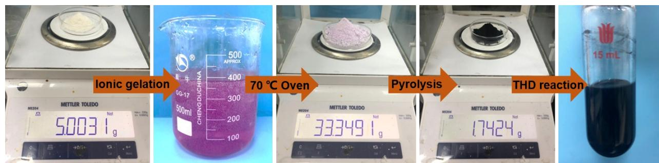
**Figure S1** Schematic illustration for the scale-up synthesis of Co@NG-6.
