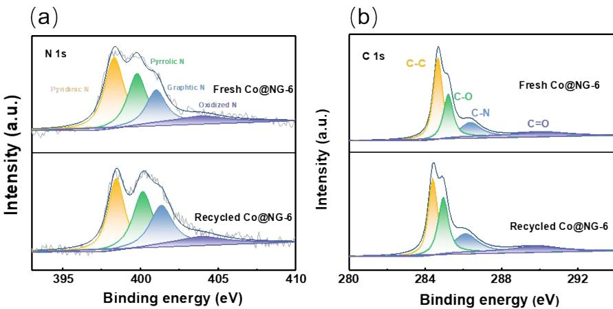
**Figure S9** XPS N 1s spectrum (e) and C 1s spectrum of Co@NG-6 before and after reaction.
