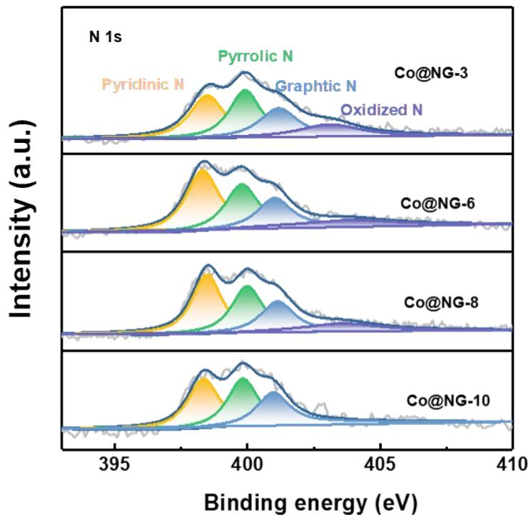
**Figure S6** High-resolution N 1s spectrum of Co@NG-U samples.
