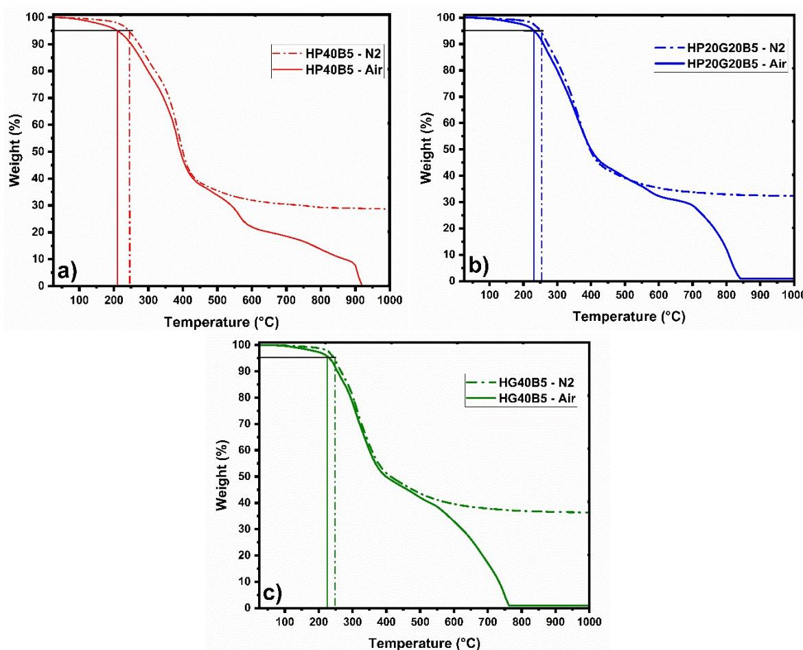
**Figure S5.** Weight ratio vs temperature for the non-isothermal degradation of humins based resins conducted under inert (dash line) and oxidative atmosphere (solid line)
