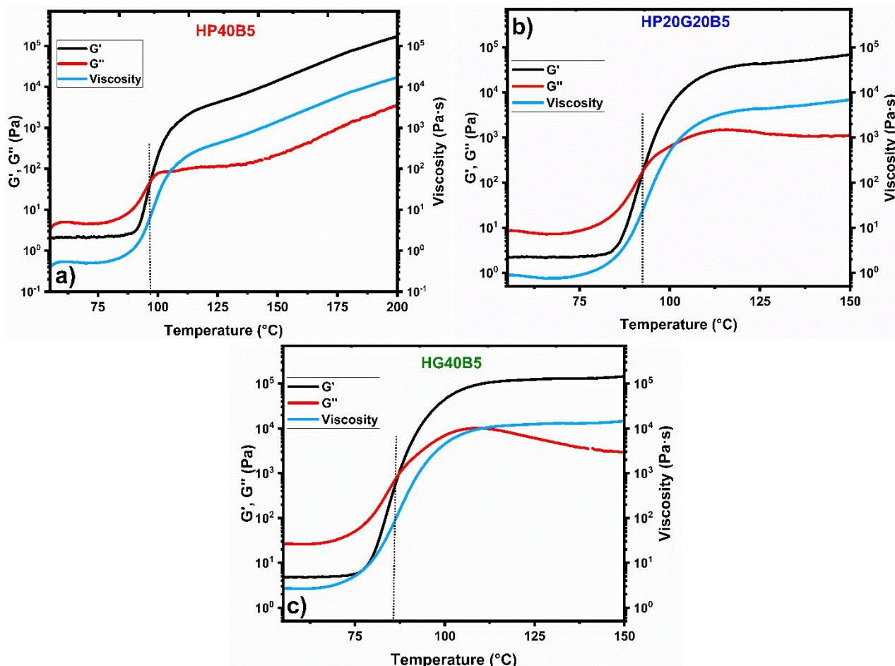
**Figure S3.** Rheometry study of the copolymerization systems: a) 55% H- 40% PEGDE- 5% BDMA, b) 55% H- 20% PEGDE- 20% GDE- 5% BDMA, c) 55% H- 40% GDE- 5% BDMA
