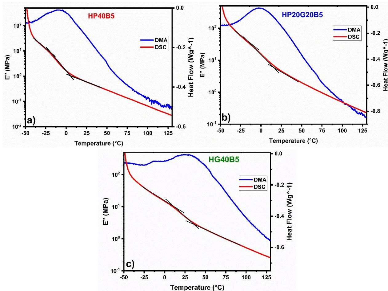
**Figure S4.** DMA mechanical response of materials as compared to DSC scans showing the glass transition temperature for the copolymerized humins-based resins
