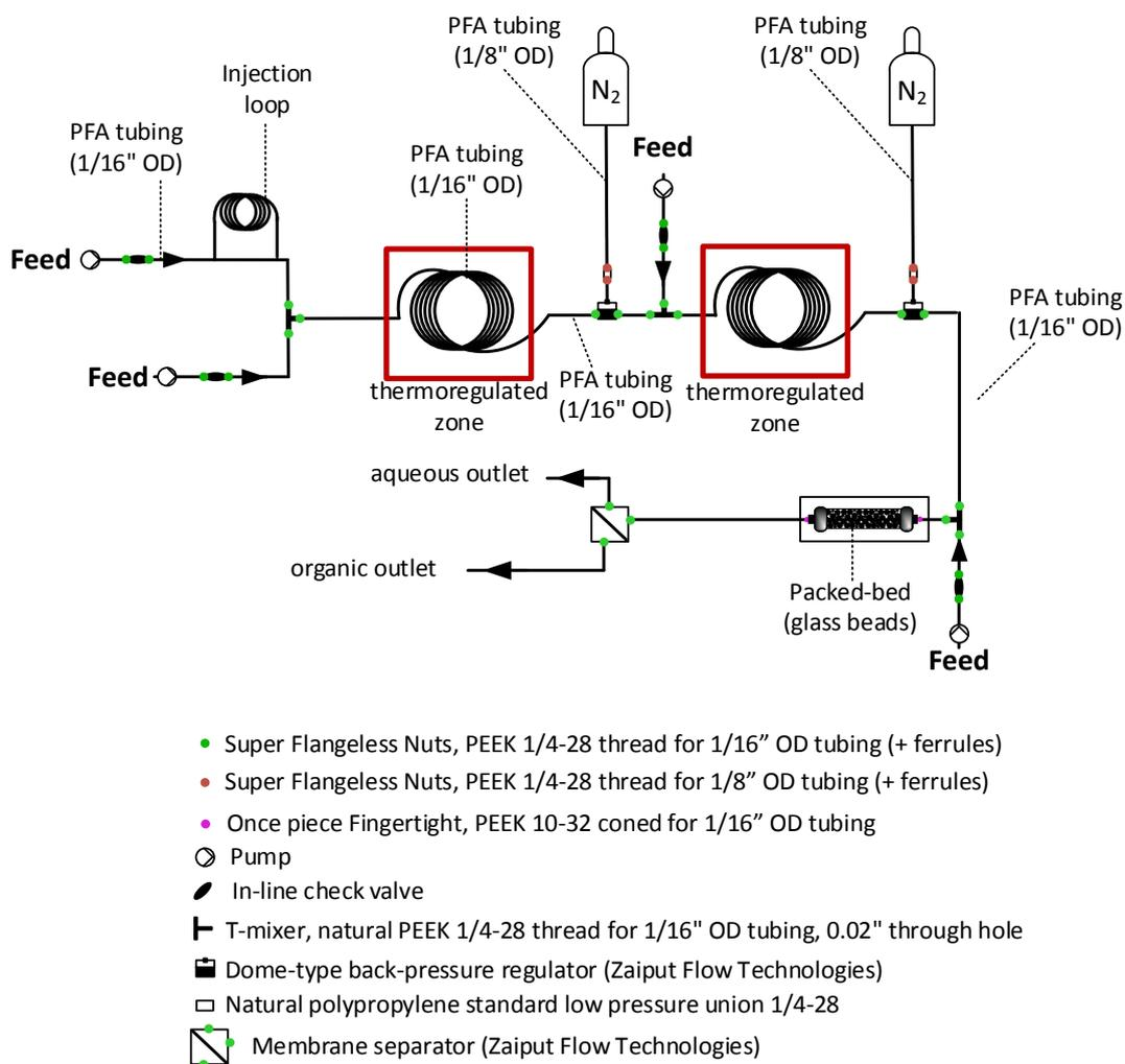
**Figure S3.** Detailed setup for the concatenated hydrochlorination/dechlorination sequence of glycerol (**1**) featuring the in-line extraction module (pressure regulation downstream the membrane separator is omitted for clarity).
