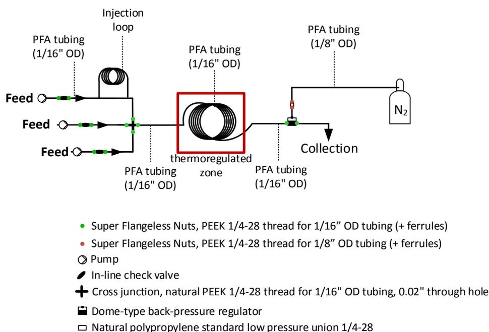
**Figure S2.** Detailed setup for the continuous flow hydrochlorination of glycerol (1) in presence of an organic carrier.
