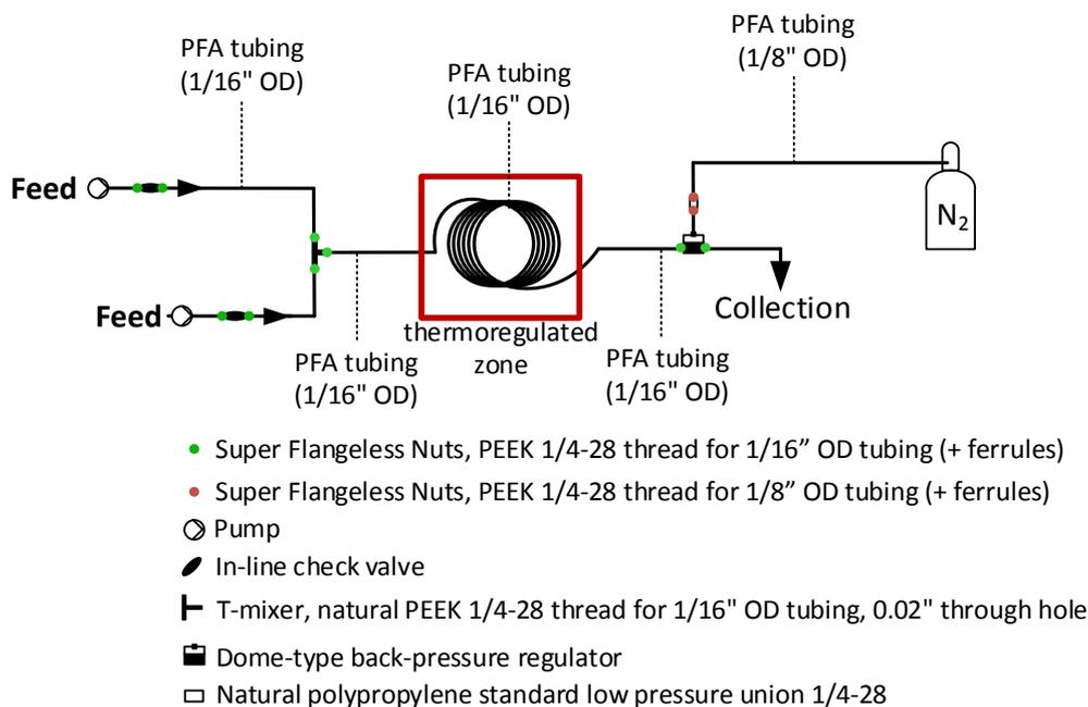
**Figure S6.** Detailed setup for the catalyst-free continuous flow aminolysis of glycidyl derivatives **8a,b** toward propranolol **10a**.
