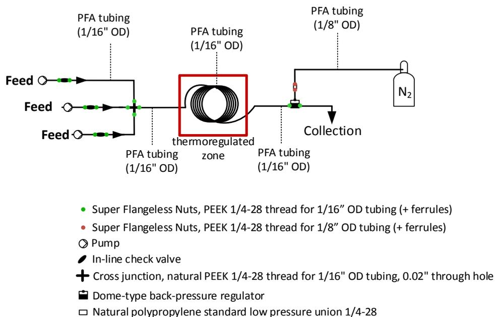
**Figure S7.** Detailed setup for the catalyzed continuous flow aminolysis of glycidyl derivatives **8a,b** toward APIs **10a-d**.
