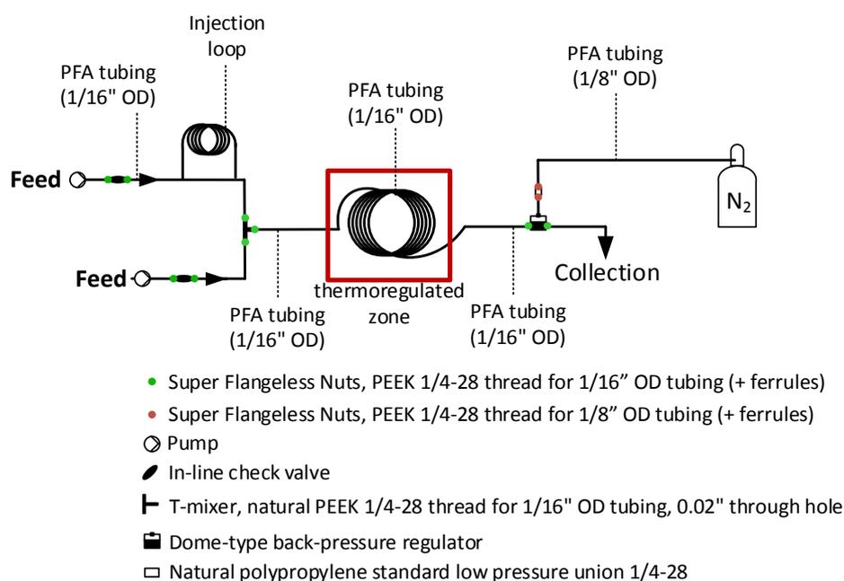
**Figure S1.** Detailed setup for the continuous flow hydrochlorination of glycerol (1).
