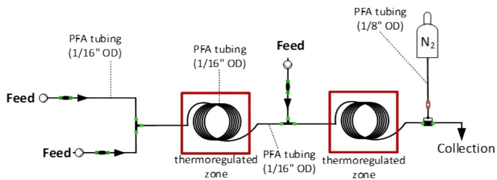
**Figure S8.** Detailed setup for the catalyst-free continuous flow etherification/aminolysis sequence toward APIs **10a,b**.
