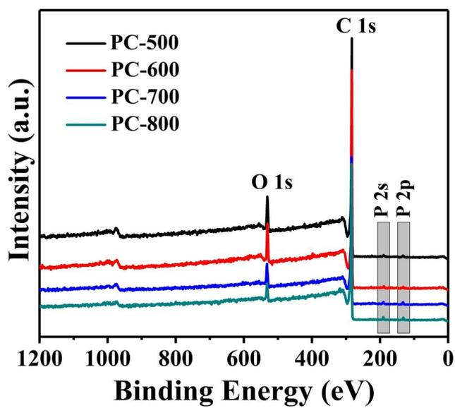
Fig. S3. The wide scan spectra of PC-500, PC-600, PC-700 and PC-800 catalysts.
