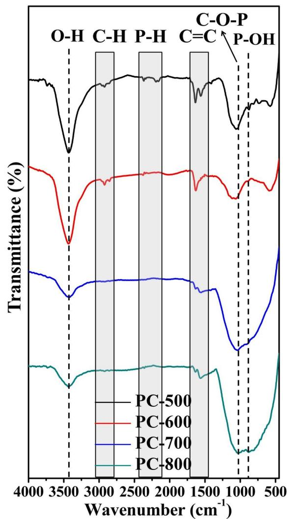
**Fig.S7.** The FT-IR spectra of PC-500, PC-600, PC-700 and PC-800 catalysts.
