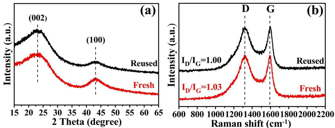
**Fig. S10.** The comparison between fresh and reused PC-700 catalyst in PXRD patterns (a) and Raman spectra (b).
