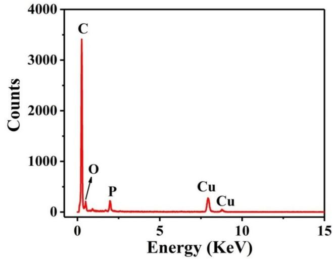
Fig. S4. The EDX spectrum of PC-700 catalyst.
