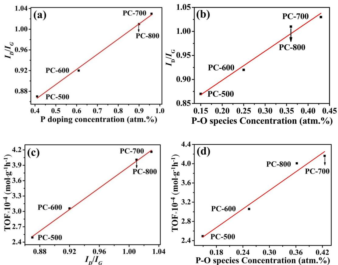
**Fig.S6.** (a) Linear correlation between the P doping concentration and the values of  $I_D/I_G$ . (b) Linear correlation between the P-O species concentration and the values of  $I_D/I_G$ . (c) Linear correlation between the values of  $I_D/I_G$  and TOF values in aerobic oxidation of benzyl alcohol. (d) Linear correlation between the P-O species concentration and TOF values in aerobic oxidation of benzyl alcohol.
