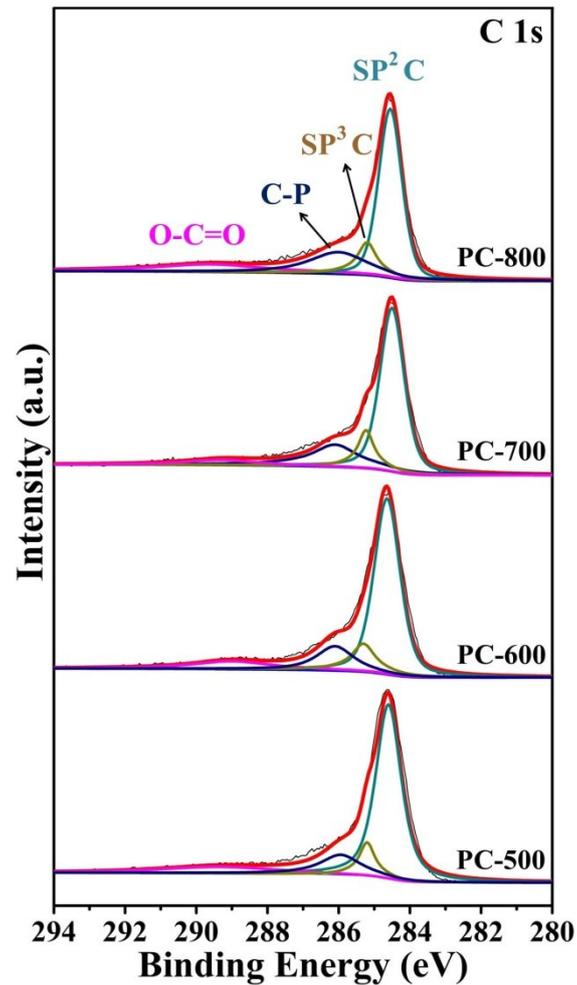
Fig. S5. XPS C 1s spectra of PC-X catalysts, i.e., PC-500, PC-600, PC-700 and PC-800, respectively.
