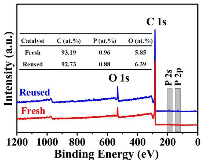
**Fig. S11.** The comparison between fresh and reused PC-700 catalyst of the contents of C, O and P in XPS wide scan spectrum.
