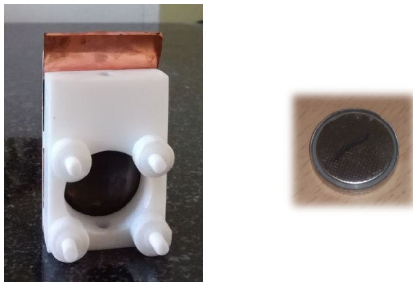
Fig. S8. (left) Electrolytic cell design. The anode wall is removed to show the electrolyte compartment and copper foil cathode coated with germanium nanoparticles after electrolysis. (right) Sample of fabricated half cell.
