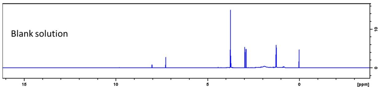
Fig. S5 NMR spectra of the residual solution after solvothermal reaction without GCN material
