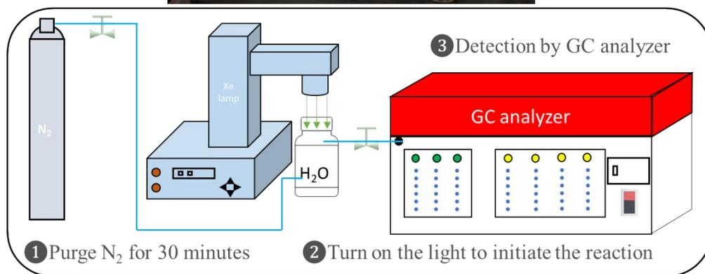
Fig. S1 Optical photo and schematic diagram of photocatalytic reaction system
