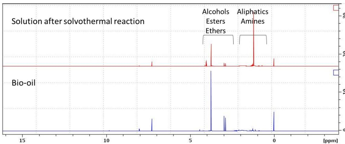
Fig. S4 NMR spectra of the crude bio-oil and the liquid solution after solvothermal reaction
