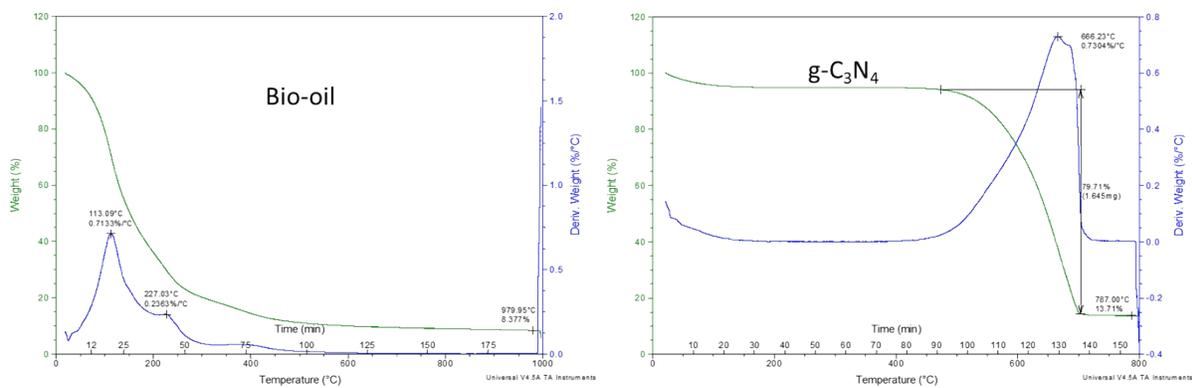
Fig. S7 TG analysis of bio-oil liquids and  $\text{g-C}_3\text{N}_4$  sample
