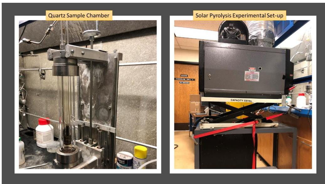
Fig S3 Optical photo of solar pyrolysis experimental set-up and quartz sample chamber
