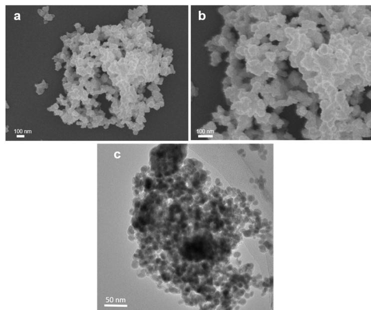
**Fig. S2** (a, b) SEM images and (c) TEM image of as-synthesized nickel nanoparticles.
