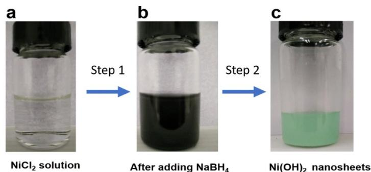
**Fig. S1** The color changes in the preparation process of hierarchical porous  $\alpha$ -Ni(OH)<sub>2</sub> nanosheets.
