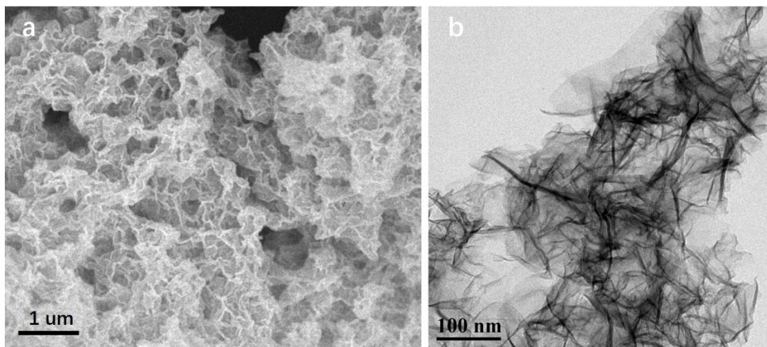
**Fig. S5** (a) SEM image and (b) TEM image of the  $\alpha$ -Ni(OH)<sub>2</sub> electrode materials after cycling test.
