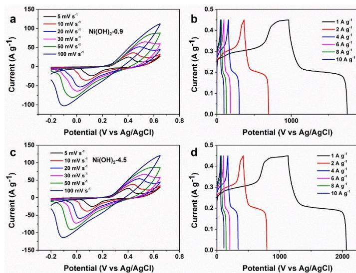
**Fig. S6** (a, b) CV curves at various sweeping rates and GCD curves at various current densities for  $\text{Ni(OH)}_2\text{-}0.9$ . (c, d) CV curves at various sweeping rates and GCD curves at various current densities for  $\text{Ni(OH)}_2\text{-}4.5$ .
