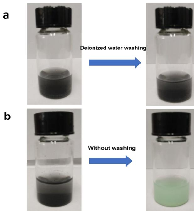
**Fig. S4** Color changes of solution with Ni nanoparticles. (a) Ni nanoparticles prepared in the first step were washed using deionized water and then stocked in the fresh deionized water. (b) Ni nanoparticles prepared in the first step were not washed and kept stationary state in the origin solution.
