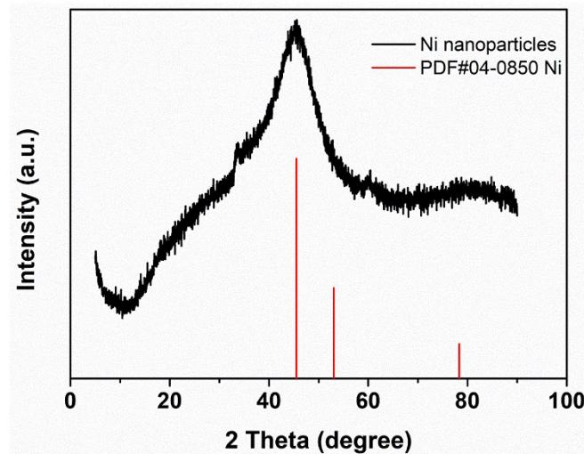
**Fig. S3** XRD pattern of as-synthesized Ni nanoparticles.
