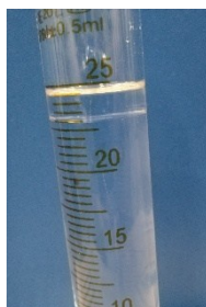
Figure S5. Digital photographs of the solution after Kolbe electrolysis. The unreacted CA and hydrophobic products (i.e. tetradance, heptane, and the isomers of heptene) gathered together on the surface of the solution. An obvious phase boundary was formed between the aqueous solution of bicarbonates and hydrophobic biofuels products.
