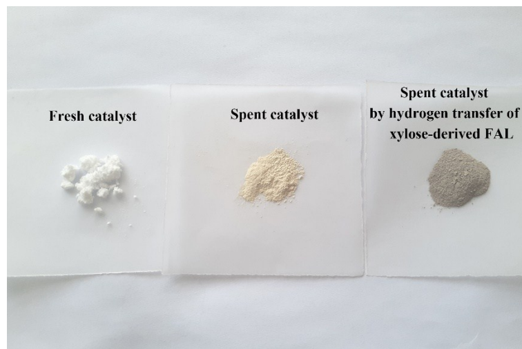
Figure S8. The color change of the BZC catalyst before and after the reaction.
