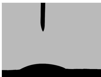
Fig. S7 Contact angle (CA) of a water droplet on the surface of Zr-tannin.
