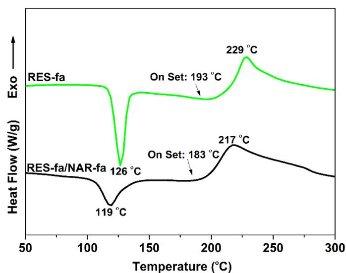
**Figure S13.** DSC thermograms of benzoxazine resins (RES-fa and **RES-fa/NAR-fa**
