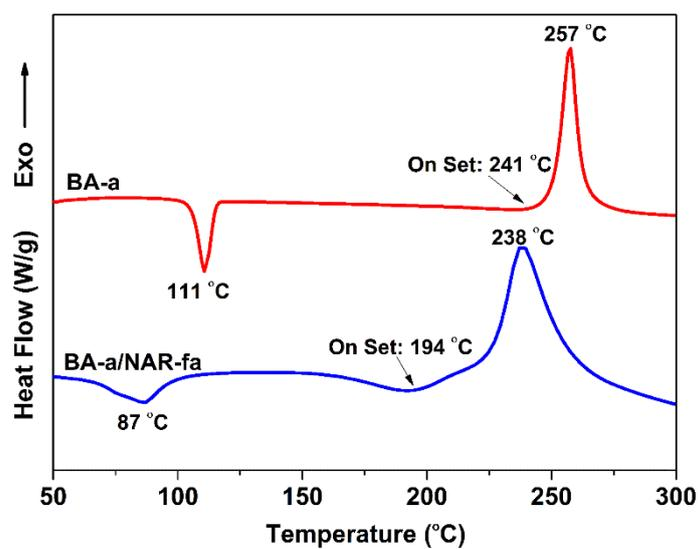
**Figure S12.** DSC thermograms of benzoxazine resins (BA-a and **BA-a/NAR-fa blend**).
