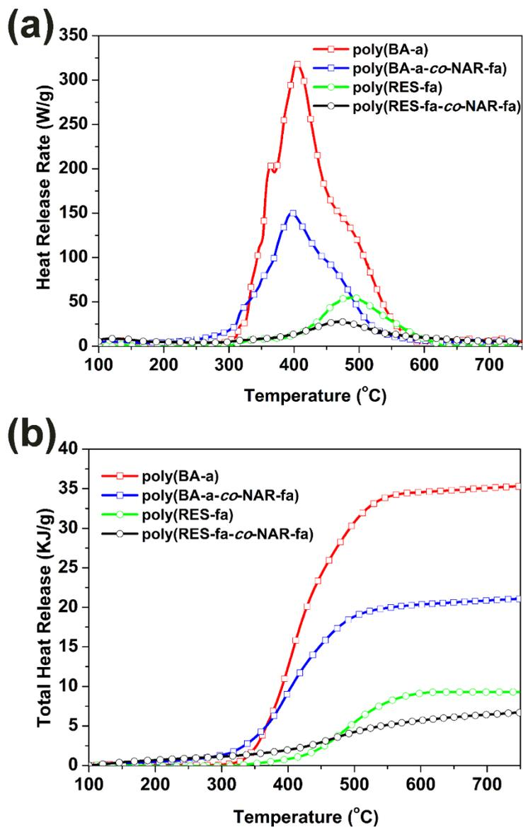
**Figure S16.** Microscale combustion calorimetric (MCC) analysis of polybenzoxazines. Plots of the heat release rate (a) and total heat release (b) as a function of the temperature.
