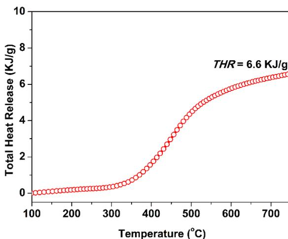
**Figure S11.** Microscale combustion calorimetric (MCC) analysis of **poly(NAR-fa)**. Plots of the total heat release as a function of the temperature.
