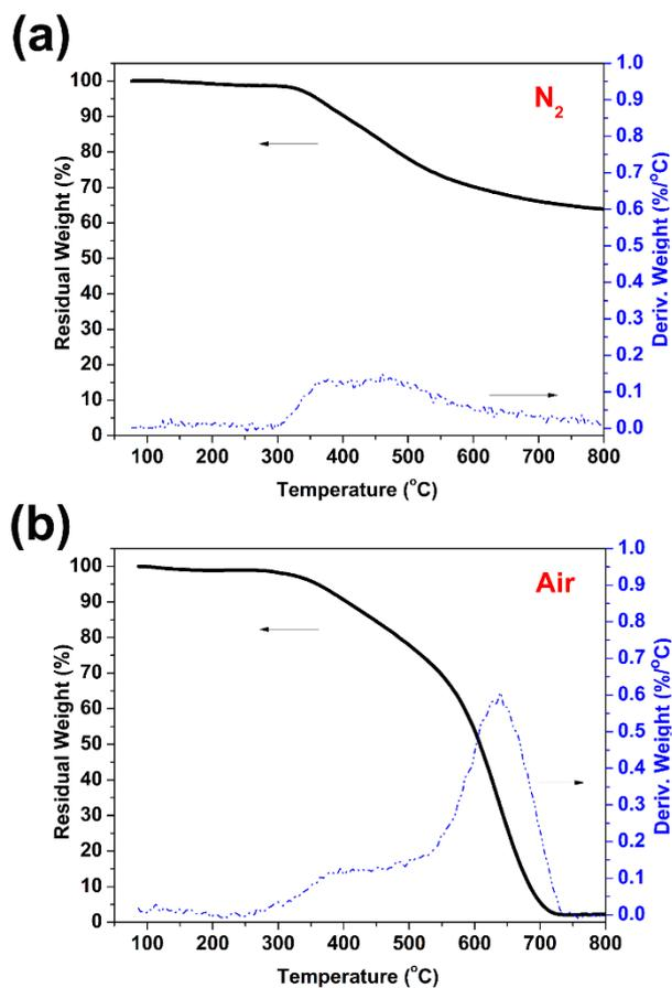
**Figure S10.** TGA (—) and DTG (···) thermograms of **poly(NAR-fa)** under nitrogen (a) and air (b) atmospheres.
