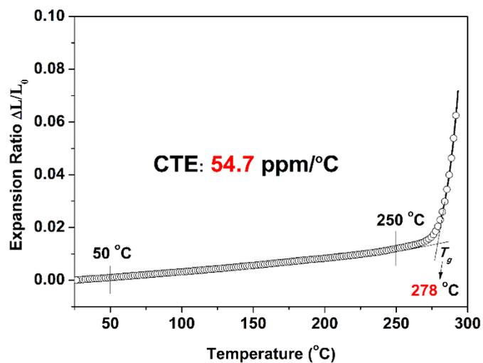
**Figure S9.** Thermomechanical analysis of **poly(NAR-fa)**.
