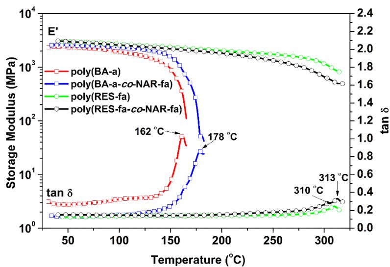
Figure S14. Dynamic mechanical analysis of polybenzoxazines.
