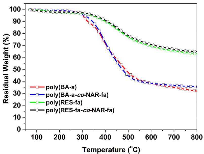
Figure S15. TGA (—) thermograms of polybenzoxazines under nitrogen atmosphere.
