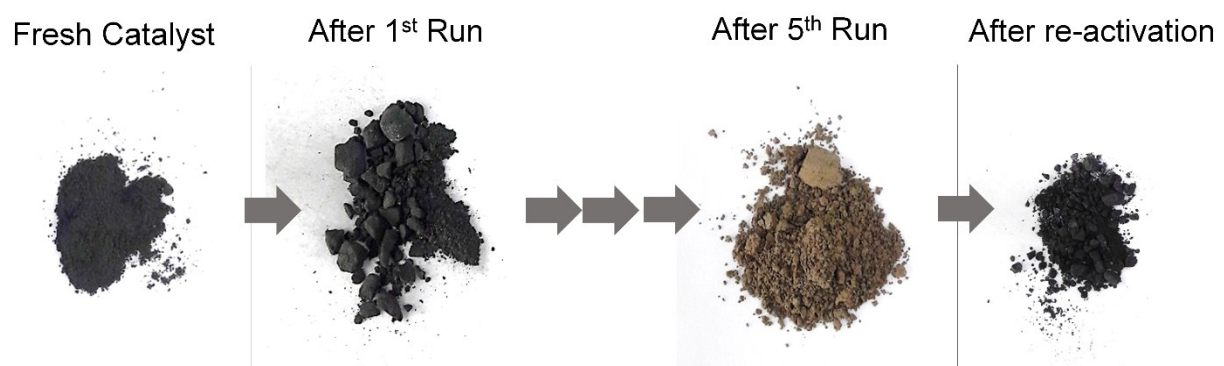
Fig. S13 Photographs of fresh, spent, and re-activated catalysts showing color changes. Re-activation conditions: 500 °C, 4 h, 5% H 2 /Ar at flow rate of 30 mL min -1 .
