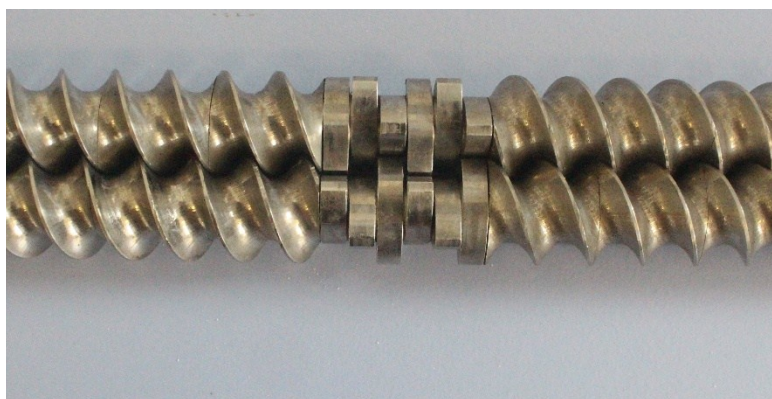
Fig. S1.3†: Screw configuration for Kneading zone 2
