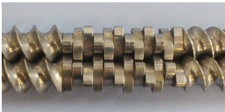
Fig. S1.4†: Screw configuration for Kneading zone 3
