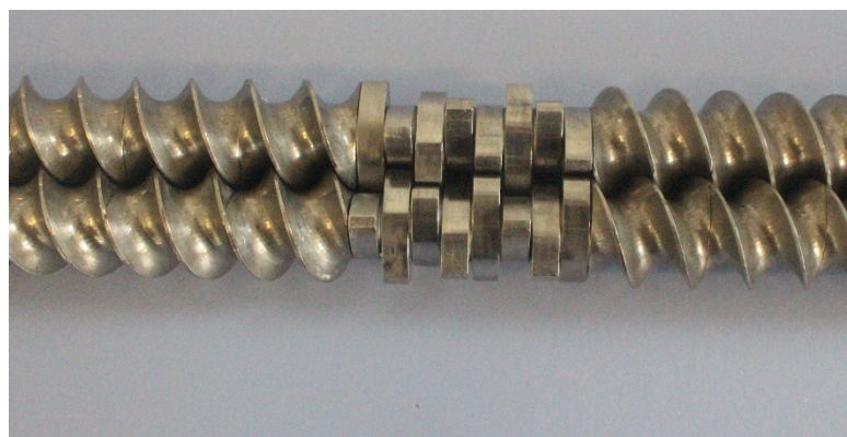
Fig. S1.2†: Screw configuration for Kneading zone 1
