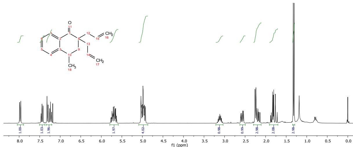
Figure 32.  $^1\text{H}$  NMR spectrum of **6c**
