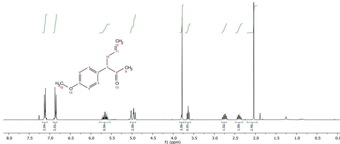
**Figure 18.**  $^1\text{H}$  NMR spectrum of **3f**
