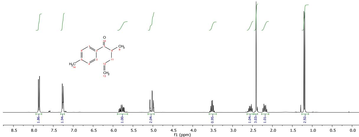
**Figure 5.**  $^1\text{H}$  NMR spectrum of **3b**
