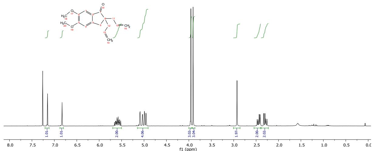
Figure 40.  $^1\text{H}$  NMR spectrum of 6f
