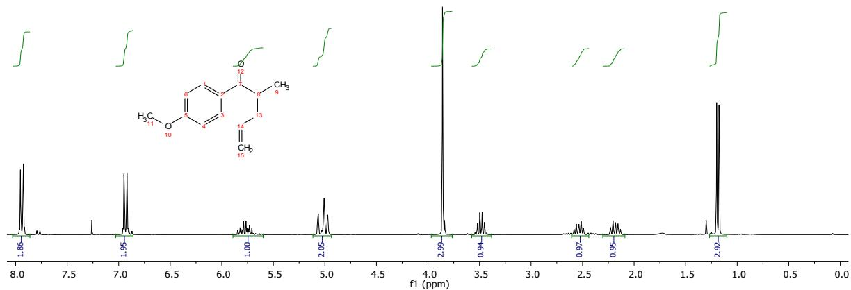
**Figure 7.**  $^1\text{H}$  NMR spectrum of 3c
