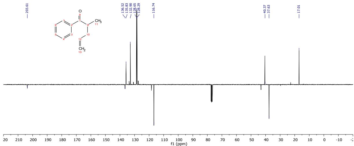
Figure 2. APT NMR spectrum of 3a
