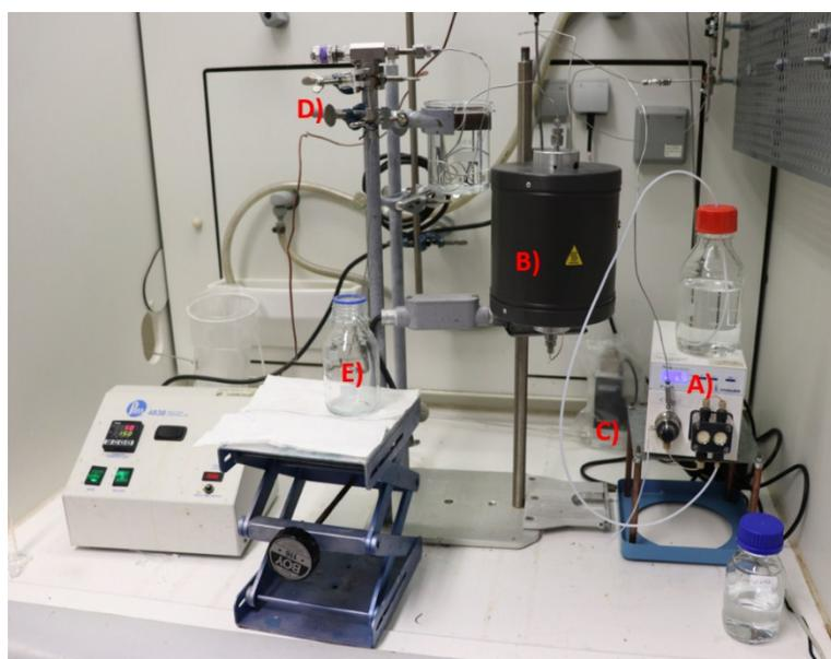
**Figure S3.** The reaction set up consists of A) HPLC pump equipped with pressure control B) heating unit (see the inner part of it at Figure S4) C) Mass flow controller for H<sub>2</sub> D) relief valve used for pressure controlling, connected with E) Sample collector.
