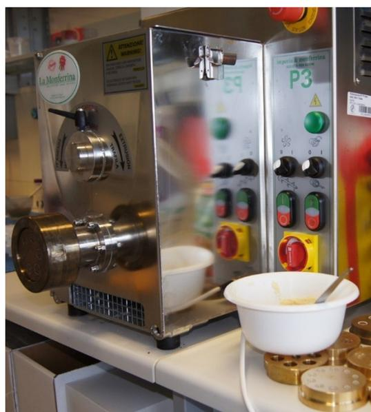
**Figure S1.** The extrusion machine from La Monferrina P3.
