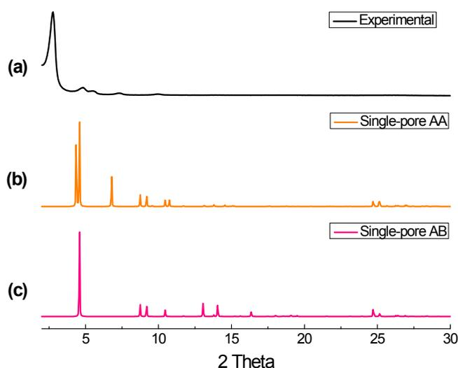
**Figure S46.** Comparison of the experimental PXRD of **COF-NJU-1** with the simulated patterns of the single-pore isomer with AA and AB stacking.
