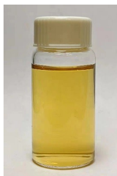
Figure S5 The degraded polymer solution after degradation in 0.5 M NaOH solution for 5 h.
