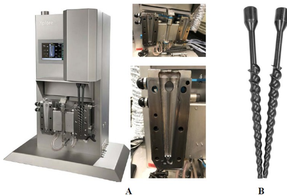
Fig. 1 Photographs of Xplore® MC 15 micro twin-screw extruder (A) and screws (B).
