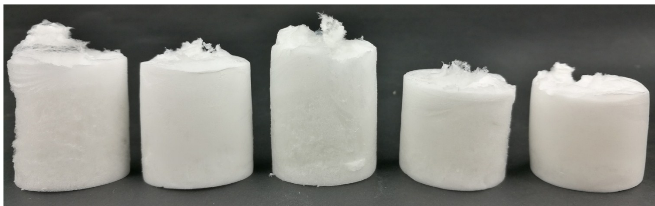
5 Figure S2. Aerogels produced by freeze-drying from CNFs obtained from DES treated cellulose fibers, from left to right: CCIMI 15 min 60 °C; CCIMI 180 min 60 °C; CCIMI 15 min 100 °C; CCIMI 180 min 100 °C; CCUrea 120 min 100 °C
