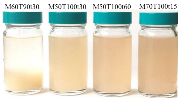
Figure S2. Stability of aqueous dispersion of LCNFs at 0.2% after standing for two weeks at 4 °C
