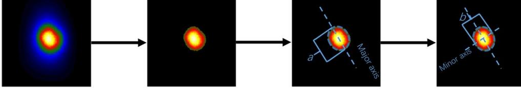
Fig. S3 Schematic diagram of plasma flatness calculation
