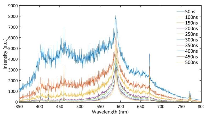
Fig. S1 Typical LIBS spectra at different detection delay time from 50 to 500 ns.
