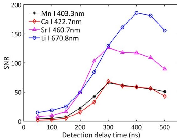
Fig. S2 SNRs of different analytical lines as a function of detection delay time.
