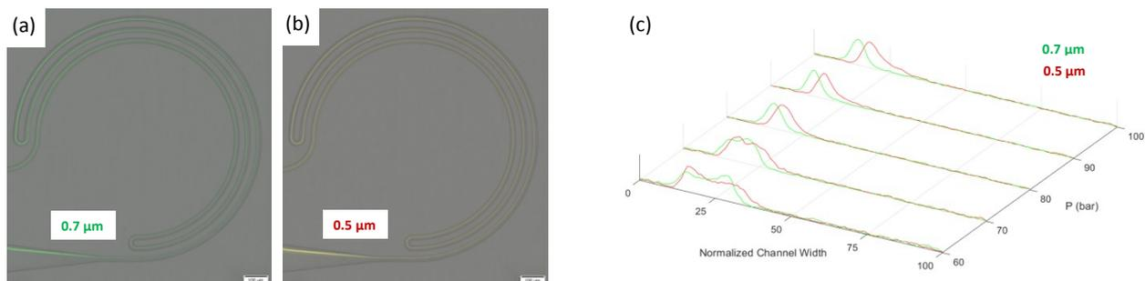
**Figure S5** Performance of a microfluidic chip with three loops, cross section  $7.3 \times 20 \mu\text{m}$  ( $H \times W$ ) and 0.5 mm in  $R$  with (a) 0.7 and (b) 0.5  $\mu\text{m}$  particles at 90 bar (45  $\mu\text{L}/\text{min}$ ). (c) Intensity plots 60–120 bar (30–60  $\mu\text{L}/\text{min}$ ). In the normalized channel width 0 and 100 represent the inner and outer wall respectively.
