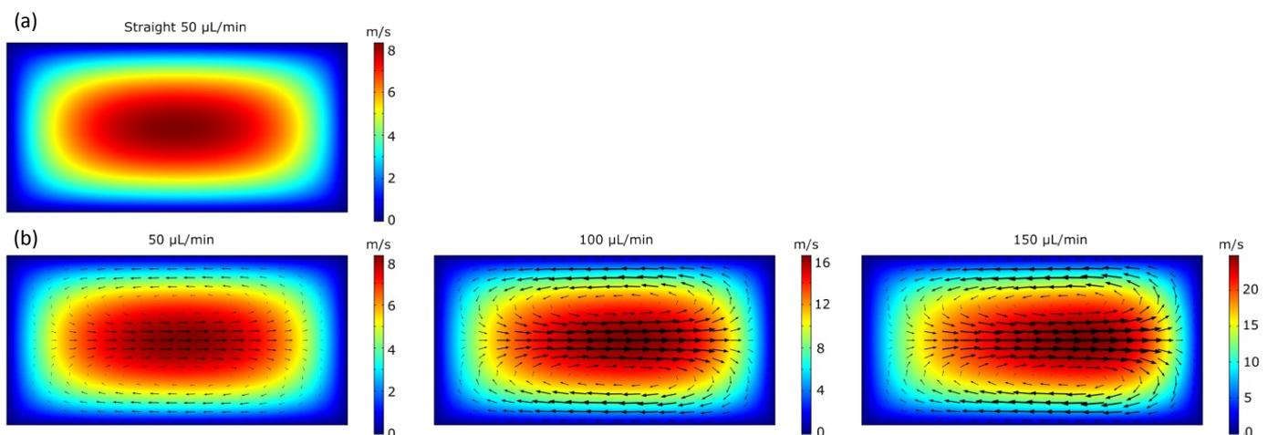
**Figure S6** COMSOL simulations of flow profiles (main flow and secondary flow) in a microchannel with cross section  $10 \times 20 \mu\text{m}$  ( $H \times W$ ). (a) Straight microchannel and (b) curved microchannel with 0.5 mm in radius. \*The arrows of the secondary flow were scaled to improve the visibility (a factor 1/2 and 1/4 for 100 and 150  $\mu\text{L}/\text{min}$ , relatively to the 50  $\mu\text{L}/\text{min}$  image).
