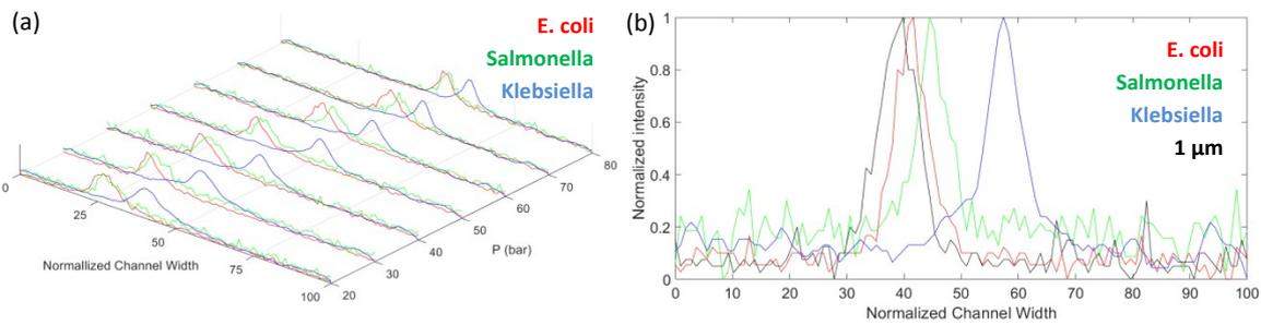
**Figure S9** (a) Intensity profiles in a microchannel with 0.5 mm in  $R$  and cross section  $10 \times 20 \mu\text{m}$  ( $H \times W$ ) with bacteria at 20 to 80 bar (30 to 120  $\mu\text{L}/\text{min}$ ). (b) Intensity profile of the bacteria and  $1 \mu\text{m}$  particles at 60 bar (90  $\mu\text{L}/\text{min}$ ). In the normalized channel width 0 represents the inner wall and 100 the out wall.
