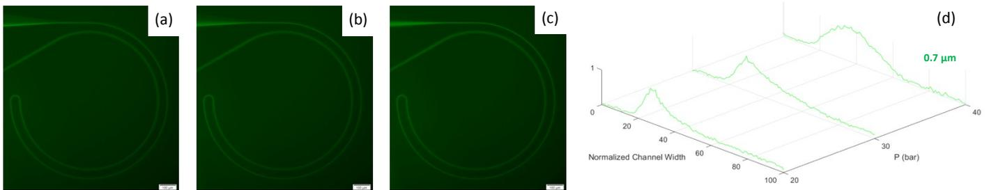
**Figure S1** Performance with of 0.7  $\mu\text{m}$  particles in a microfluidic chip with 0.5 mm in  $R$  and cross section  $10 \times 20 \mu\text{m}$  ( $H \times W$ ) at 20, 30 and 40 bar (30, 45 and 60  $\mu\text{L}/\text{min}$ ). (a-c) Raw images. (d) Intensity profiles. In the normalized channel width 0 and 100 represent the inner and outer wall respectively.
