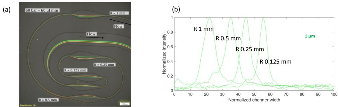
**Figure S3** (a) Positions of equilibrium of 1 and 2  $\mu\text{m}$  particles (green and red respectively) at different radii (1, 0.5, 0.25 and 0.125 mm) at 60 bar – 60  $\mu\text{L}/\text{min}$ . (b) Intensity profile of 1  $\mu\text{m}$  particles; from left to right, 1, 0.5, 0.25 and 0.125 mm in  $R$ . In the normalized channel width 0 and 100 represent the inner and outer wall respectively.
