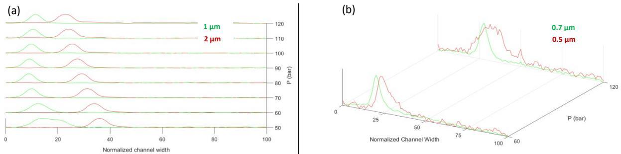
**Figure S4** Intensity profiles in a microfluidic chip with 0.5 mm in  $R$  and cross section  $7.3 \times 20 \mu\text{m}$  ( $H \times W$ ). (a) 1 and 2  $\mu\text{m}$  particles from 50 to 120 bar (37 to 90  $\mu\text{L}/\text{min}$ ). (b) 0.5 and 0.7  $\mu\text{m}$  particles at 60 and 120 bar (45 and 90  $\mu\text{L}/\text{min}$ ). In the normalized channel width 0 and 100 represent the inner and outer wall respectively.
