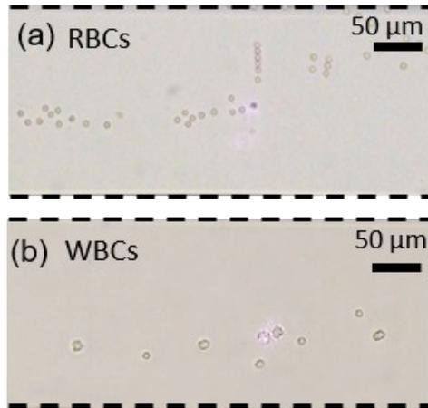
Figure S3. Optical mobility test of RBCs and WBCs, the flow rate is keep the same with of CC-RBCs mobility test. Although RBCs (a) is relatively smaller than WBCs (b), the higher RI resulting in obviously larger displacement.
