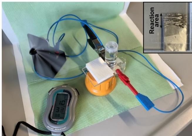
**Fig. S13** Running time measurement of a mini-fan (power rating 10 mW) powered by a paper-based  $\mu$ Al-air battery (geometric electrode active area:  $8 \times 15 \text{ mm}^2$ ). The inset shows that after 70 min discharge the Al anode is almost fully consumed.
