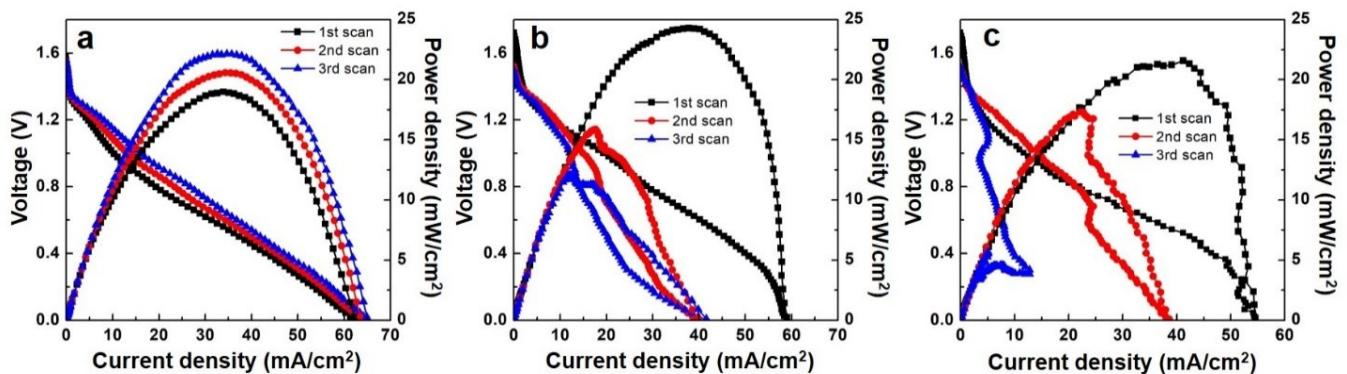
**Fig. S4** Polarization ( $V$ - $I$ ) and power density curves of paper-based  $\mu$ Al-air battery with 1.5 M (a), 2.0 M (b) and 2.5 M (c) KOH solution by continuous staircase linear scan voltammetry.
