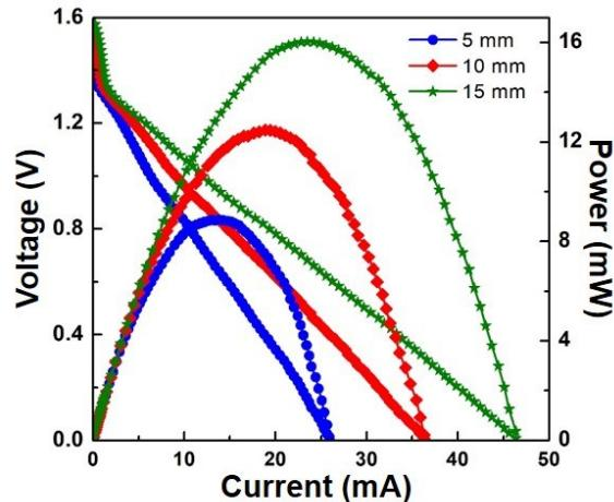
**Fig. S12** Polarization ( $V$ - $I$ ) and power density curves of paper-based  $\mu$ Al-air batteries with different electrode sizes.
