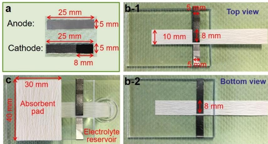
**Fig. S1** (a) Dimensions of the anode and cathode electrodes. (b) Display of the prototypical paper-based  $\mu$ Al-air battery from top and bottom view. (c) A prototypical paper-based  $\mu$ Al-air battery during discharge.
