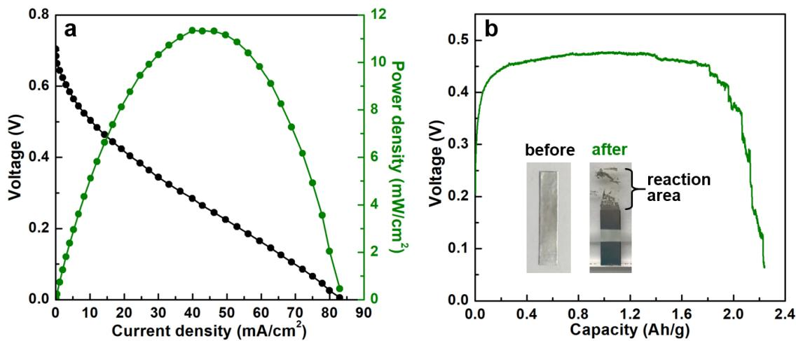
**Fig. S9** Polarization ( $V$ - $I$ ) and power density curve (a) and discharge curve (b) of the paper-based  $\mu$ Al-air battery by using 2 M NaCl as electrolyte. The insets are the optical photos of the anode aluminum foil after discharge.
