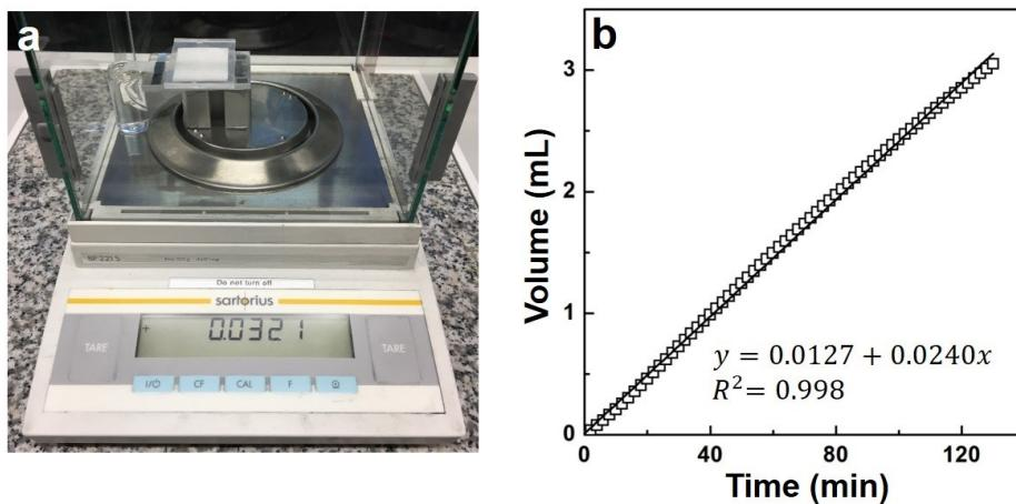
**Fig. S2** (a) Flow rate measurement of the electrolyte (1.5 M KOH solution) on paper channel (VWR grade 417). (b) The volume of the electrolyte accumulated on absorbent pads was plotted against elapsed time. The flow rate calculated by linear regression is marked.
