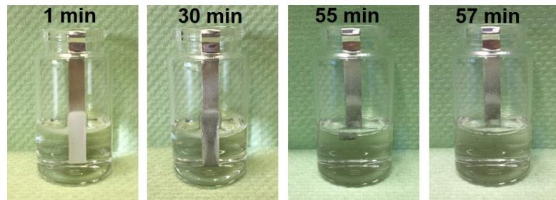
**Fig. S7** Aluminum foil ( $8 \times 5 \text{ mm}^2$ ) immersed in 1.5 M KOH solution.
