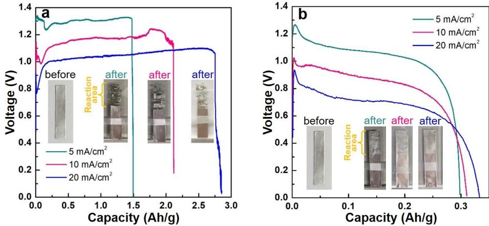
**Fig. S6** Discharge curves of paper-based  $\mu$ Al-air battery (a) and non-fluidic Al-air battery (b) under different current density ( $5, 10, 20 \text{ mA}/\text{cm}^2$ ). The insets are the optical photos of the anode aluminum foil after discharge.
