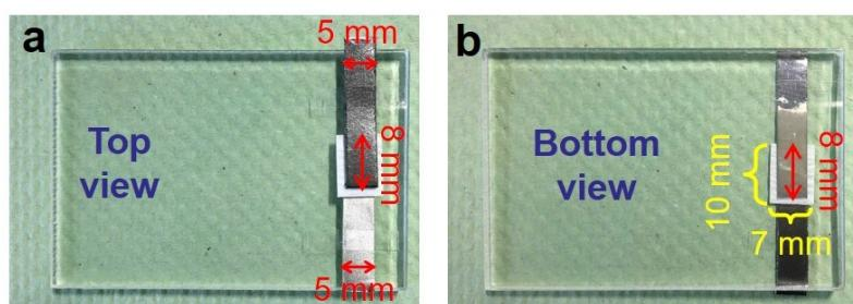
**Fig. S5** Display of the prototypical paper-based non-fluidic Al-air battery from top (a) and bottom (b) view. Reaction area for both anode and cathode electrodes are  $8 \times 5$  mm<sup>2</sup>. The size of paper is  $10 \times 7$  mm<sup>2</sup>.
