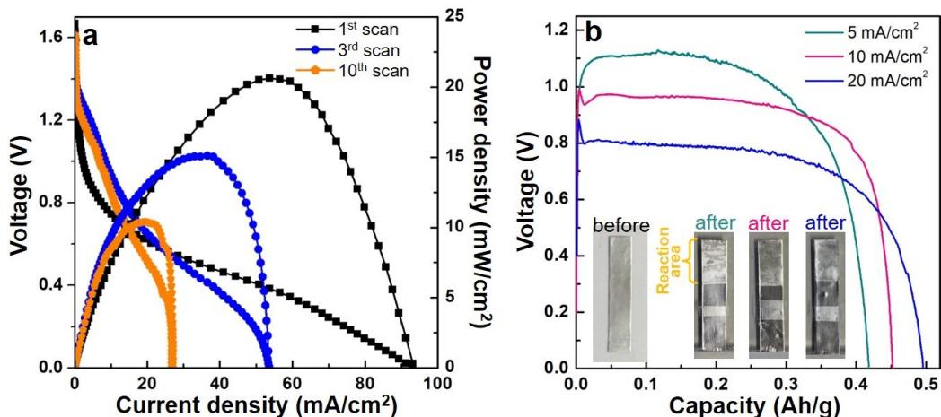
**Fig. S8** Performance of non-fluidic Al-air battery using gas diffusion layer air electrode at the cathode. (a) Polarization ( $V-I$ ) and power density curves recorded at different scan numbers. (b) Discharge curves of
