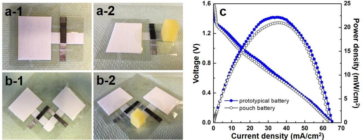
**Fig. S3** A paper-based  $\mu$ Al-air pouch battery before (a-1) and during discharging (a-2). Two paper-based  $\mu$ Al-air pouch batteries connected in series before (b-1) and during discharging (b-2). (c) Polarization ( $V$ - $I$ ) and power density curve of a single paper-based  $\mu$ Al-air battery in pouch configuration.
