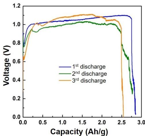
**Fig. S10** Mechanically recharging tests. Discharge curves of three paper-based μAl-air battery by using the same cathode electrode.
