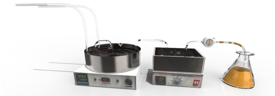
Figure S1. The schematic diagram of continuous method for full-spectrum carbon dots synthesis.
