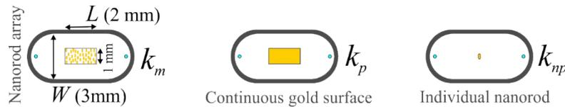
**Figure S6.** Schematic and dimension of the flow cell used for nanorod substrates.
