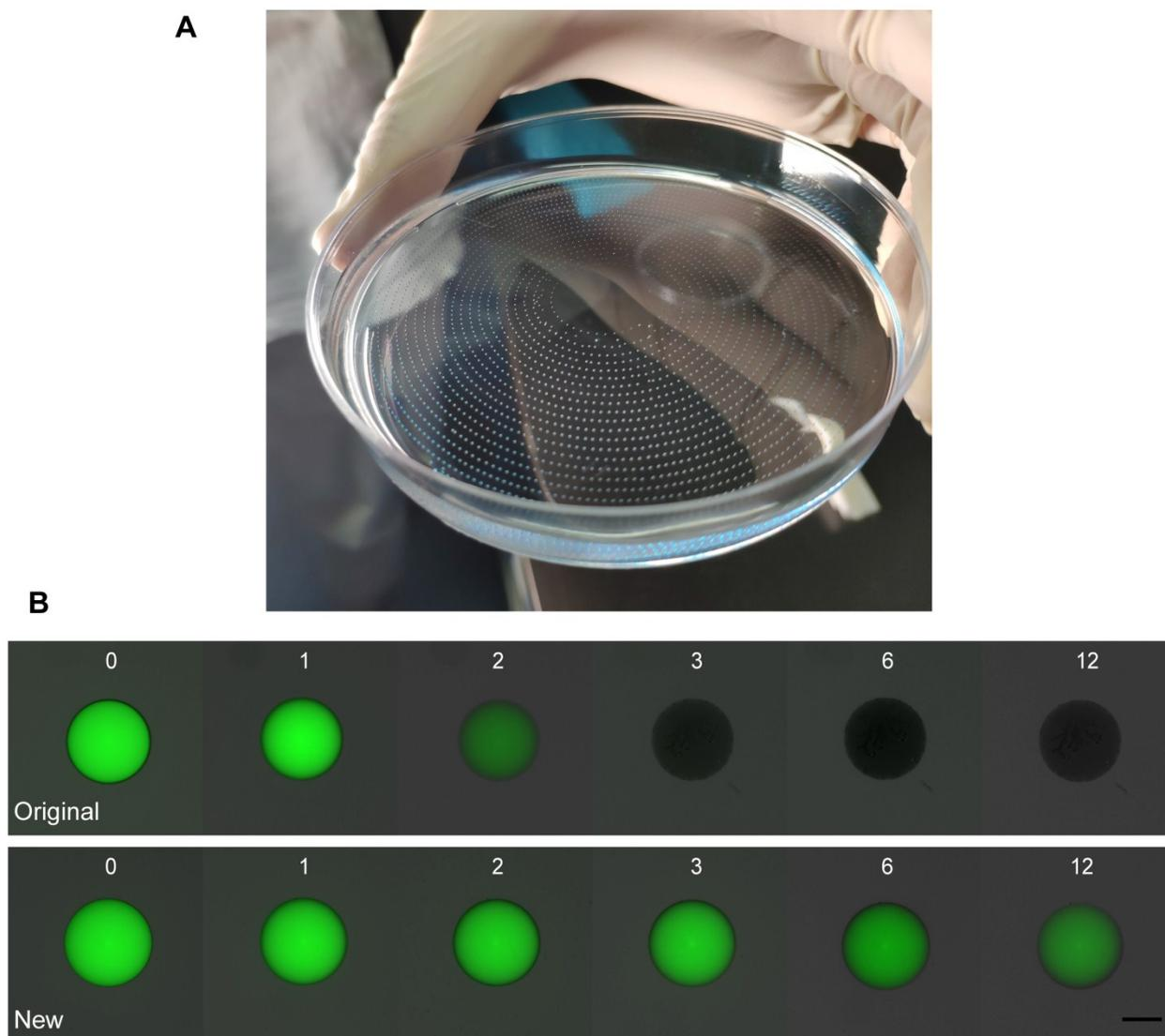
**Figure S1.** Droplet evaporation comparison of improved method and the original MSP method. (A) a picture of the MSP Petri dish; (B) Original means the method to prevent droplet evaporation in previous study (2016) and New means the method used in this study. The MSP droplets were put in 30 °C isothermal incubator with for up to 12 days. The time-lapse fluorescence photomicrographs were taken at T=0, 1, 2, 3, 6, 12 days. Scale bar is 150  $\mu\text{m}$ .
