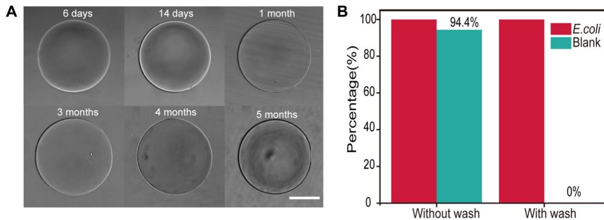
**Figure S2.** (A) The droplets evaporation control by recording the microscopic images of MSP droplets with long-term observation up to 5 months at room temperature ( $\sim 20\text{ }^{\circ}\text{C}$ ); Scale bar is  $150\text{ }\mu\text{m}$ ; (B) Contamination control with Droplet Picker: droplets with GFP-*E.coli* encapsulated called *E.coli* and without bacteria called blank, the two types of droplets were picked continually one by one.
