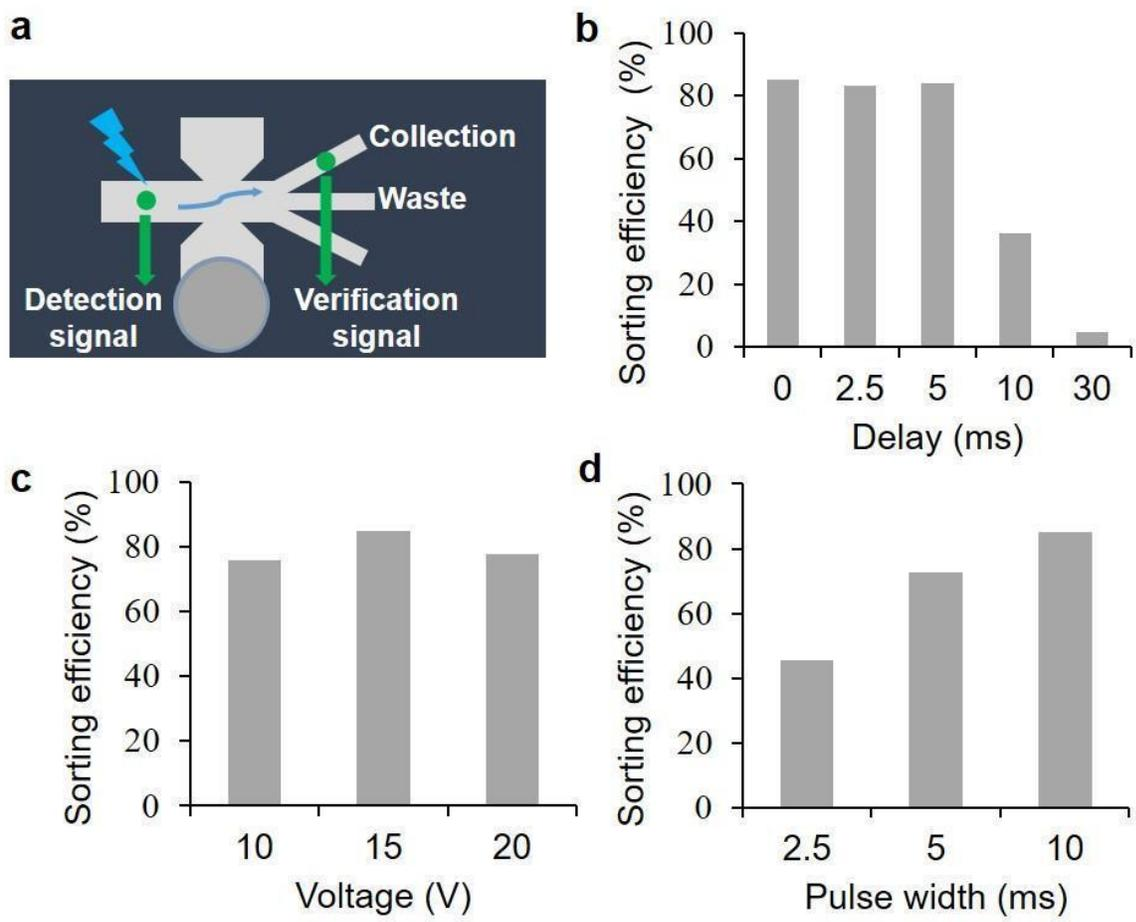
**Figure S2. Optimization of pulse delay, voltage, and width for actuator activation.**
