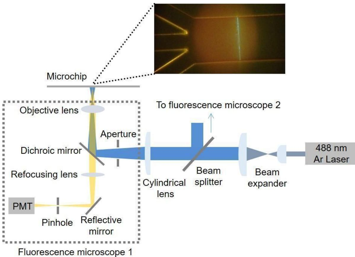
**Figure S1. Illustration of the optical setup for detection system.** Fluorescence microscope 2 is same with fluorescence microscope 1 and not represented in the figure. Also shown is a microscopic image of the linear focused beam on the chip near the inlet channels.
