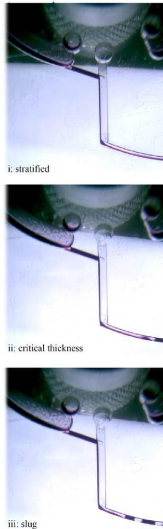
Figure2. Detailed steps of the transition from stratified flow to slug flow, i) the thickness of the stratified flow is growing through accelerating the lab-disc ii) liquid thickness is reached to a critical value and the liquid climb to the upper wall of the microchannel due to dominance of the surface tension forces, iii) the air is trapped in the form of a bubble among the liquid plugs.
