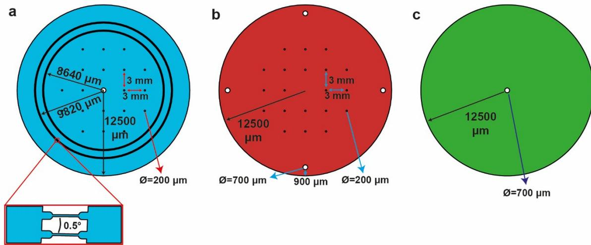
**Fig. S7. Additional feature sizes of the three microfluidic layers.** The critical features of **(a)** filtering, **(b)** transmission and **(c)** collection layers are noted. The symbol 'Ø' denotes the diameter value.
