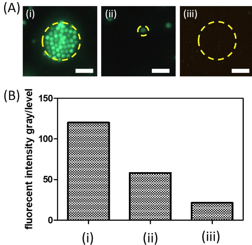
**Fig. S1** Signal enhancement at different stages. (A) Fluorescent images of (i) concentrated microbeads with sandwiched immunocomplexes (secondary enrichment), (ii) dispersed microbeads with sandwiched immunocomplexes (primary enrichment), and (iii) dispersed fluorescent dyes (no enrichment). The dotted circle defines where the signal intensity is measured. The scale bar denotes 15  $\mu\text{m}$ . (B) Mean fluorescent intensities of the three cases (i), (ii), and (iii).
